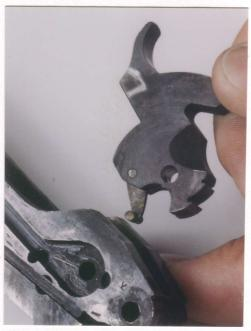
**35.** Remove the hammer upward. **Repairs Only:** Do not remove the stirrup.
