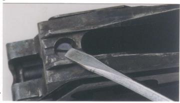
**32.** Remove the mainspring tension screw.
