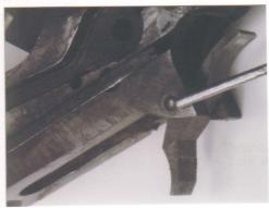
**25.** Drift out the sear pin, and remove the sear. \*\* Note placement.
