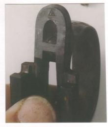
10. The trigger and its spring are easily removed from the top of the guard. The pin was removed in Step # 7. Not recommended for normal takedown: There is also a trigger stop screw at the rear inside of the guard and it is easily backed out. If this is done, though, it will have to be readjusted during reassembly.
