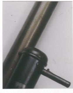
39. Remove the two opposed screws at the front of the magazine tube and take out the end cap and ring toward the front. Caution: The magazine spring will be released, so control it and ease it out. Remove the spring and follower toward the front.
