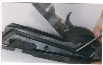
34. Be sure the shell guide plate is still swung up out of the way, and drift out the hammer pin toward the right.
