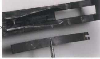
**36.** Nudge the mainspring toward the rear. When it has cleared the front bridge of the carrier, the spring can be removed upward.
