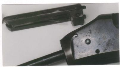
13. Slide the bolt all the way to the rear of the receiver and remove it.
