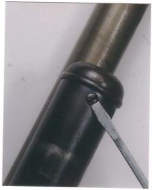
**40.** Remove the screws on each side of the magazine band, and move the band off toward the front. When the band is removed, the screw bushing at the center can be taken out. The action slide and magazine assembly can now be removed toward the front.
