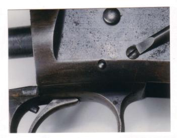
**6.** Remove the small screw on the right side of the receiver, just forward of the trigger cross pin.
