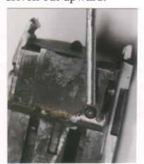
22. The right extractor is removed by inserting a small screwdriver between the extractor and its plunger. Depress the plunger toward the rear, and lift the extractor out of its recess. Keep the plunger under control, slowly release the
