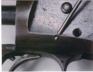
8. Cock the hammer, push the carrier release button on the right side, and insert a tool between the bolt and carrier, through the port in the right side of the receiver, to nudge the carrier downward. Remove the carrier downward and toward the front.
