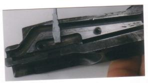
**30.** Remove the action slide lock spring.
