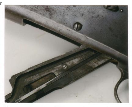
**9.** Slide (or tap with a non marring hammer) the trigger guard unit out toward the rear.
