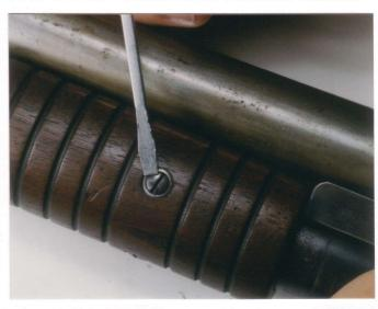
42. Remove only for Repairs: Barrel tightness in the receiver is adjustable by backing out
