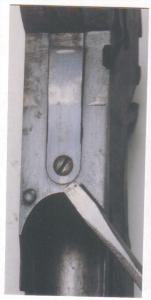
**24.** Remove the sear spring screw on the underside of the carrier, and take off the spring downward.\*\*Read reassembly tip after Step #36.
