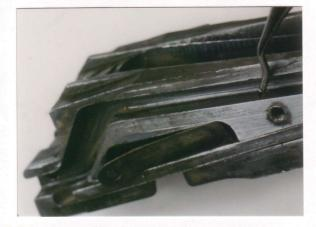
28. Insert a slim drift in the access hole in the lower edge of the action slide track, and push out and remove the slide lock joint pin downward. As the pin emerges, it can be grasped and pulled out.
