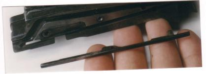
**29.** Remove the action slide lock bar.
