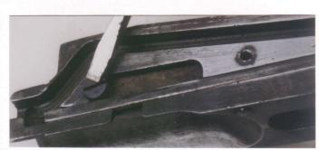
**26.** Remove the action slide lock spring screw to ease the tension off the action slide lock bar.
