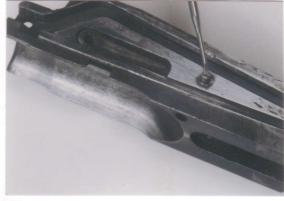
**27.** Remove the slide lock joint pin stop screw.
