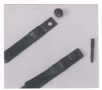
15. Older Version Shown: In older versions, the right and left shell stops are held in place by screws through the side walls of the receiver. In newer versions, the shell stops are retained by vertical pivot screws in the lower edge of the receiver on each side(they would be directly below the screw shown). Back out the screws,
