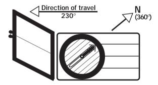
Figure  $8.3\,^\circ$  Boxing the compass needle. To take, e.g., a  $230^\circ$  heading, set the compass so  $230^\circ$  is in front of you (direction of travel). Box the compass by rotating the entire compass until the orienting arrow completely surrounds the red (north) end of the magnetic needle. Proceed in the desired direction of travel, maintaining the  $230^\circ$  heading by keeping the magnetic needle inside the orienting arrow.
