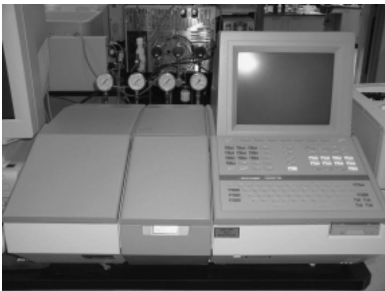
FIGURE I.3 Infrared spectrophotometry instrument. The spectra from the IR instrument are referred to as “fingerprint spectra” of a compound, which aids in classification of the chemical.
