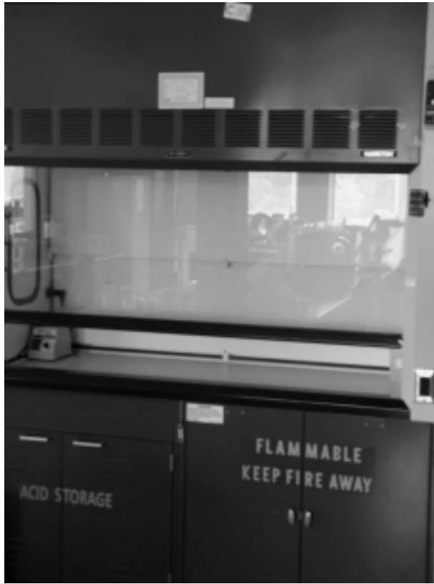
FIGURE F.9 Fume hood used for safe handling of chemicals and other hazardous materials.
