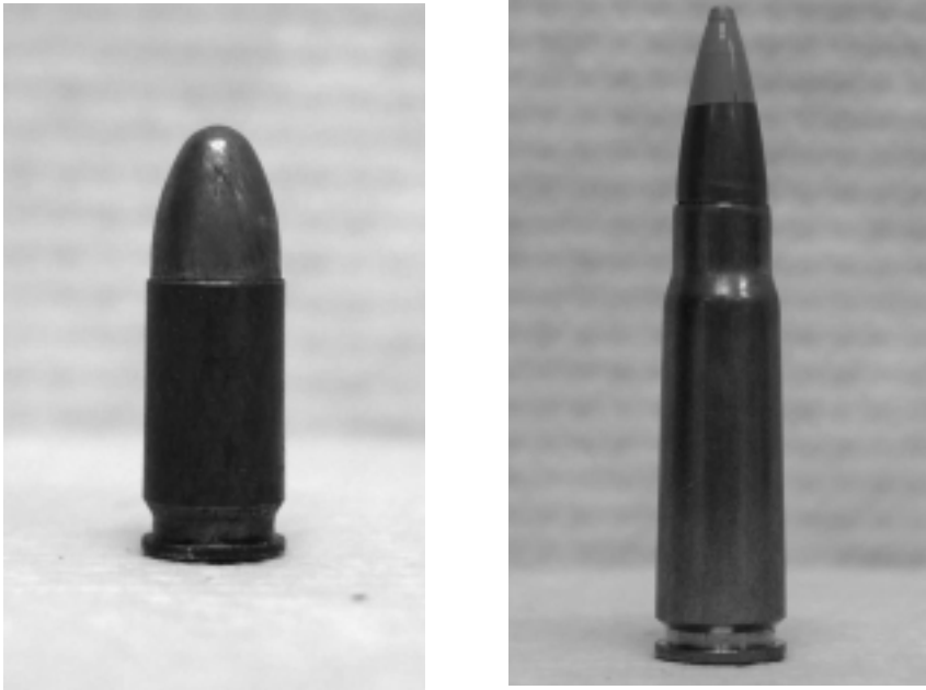
FIGURE B.8 (A) Pistol cartridge with copper-jacketed projectile. (B) Rifled cartridge with metal point bullet.
