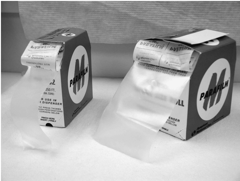
FIGURE P.2 A translucent, waxy, solid paper of various widths can be used for wrapping around the top of glass or plastic tubes to prevent the liquid inside the tube from spilling out.
