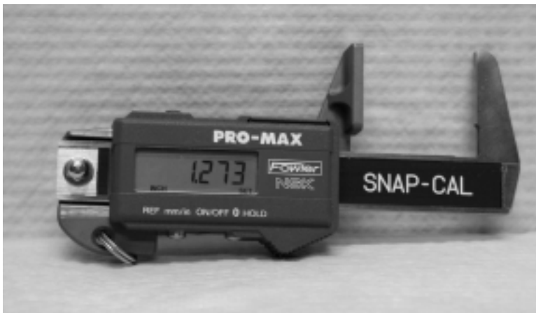
FIGURE V.1 Vernier caliper with a digital display. Used by firearm examiners to measure the gauge of a firearm.
