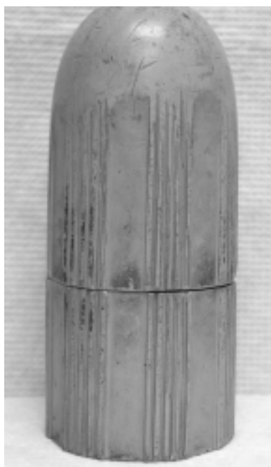
FIGURE L.1B A wooden model of a bullet is used to show how the lands and grooves on a bullet can line up.
