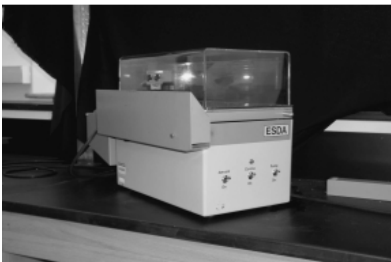
FIGURE E.6 Used by document examiners for reading indented writing from suspected pages.
