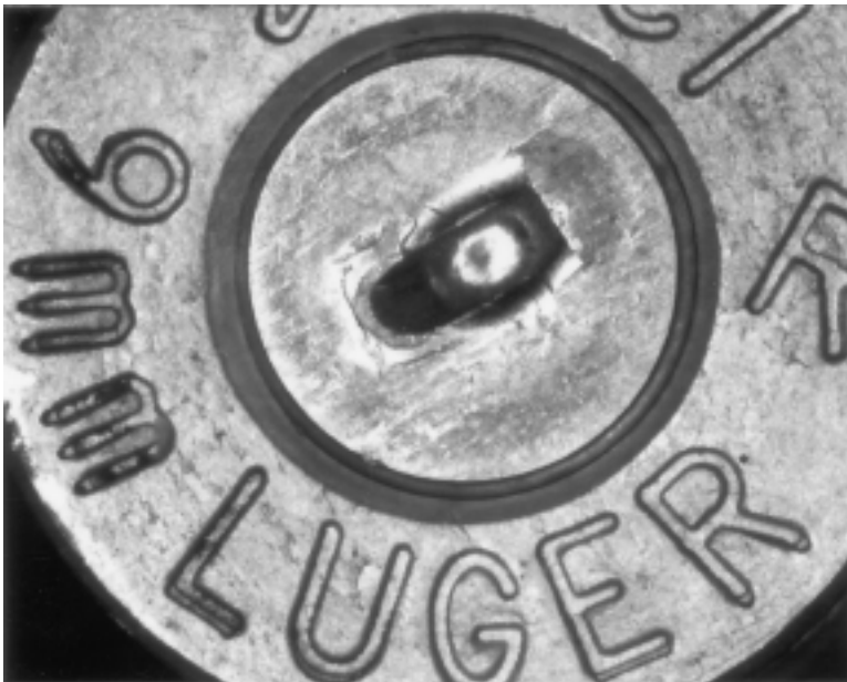
FIGURE F.4 Microscopic examination of a firing pin drag mark.
