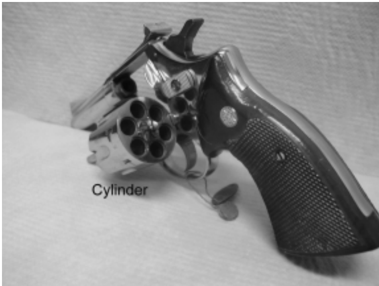
FIGURE C.23 The revolving cylinder contains six firing chambers, each able to accommodate a single cartridge.
