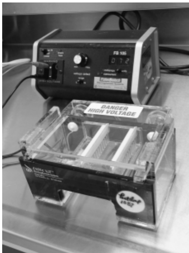
FIGURE E.3 Electrophoresis setup showing gel chamber with plastic combs and a power supply.
