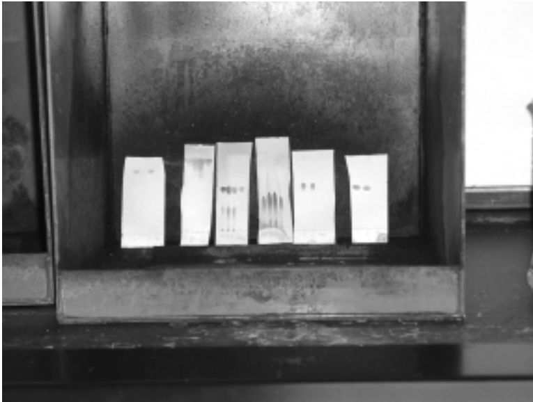
FIGURE C.15 The separation of drugs that have been spotted on thin-layer silica plates. Special chemical sprays that produce a color reaction are applied to the plates. This method of separation is performed inside a spraying chamber.
