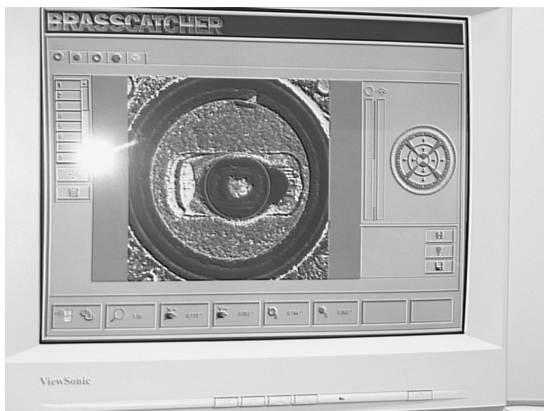
FIGURE F.5 The use of the IBIS for identifying a firing pin impression.
