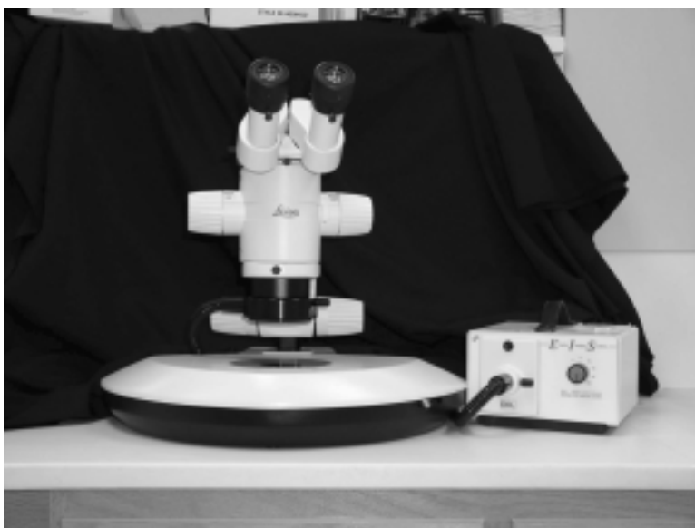
FIGURE S.13B Stereomicroscope used for the screening of trace evidence (fingernail scrapings, hairs, fibers, etc.).
