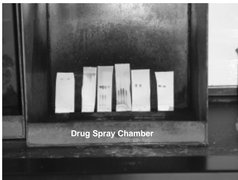
FIGURE C.12 Spraying chamber for developing thin-layer chromatograph (TLC) plates in drug chemistry.
