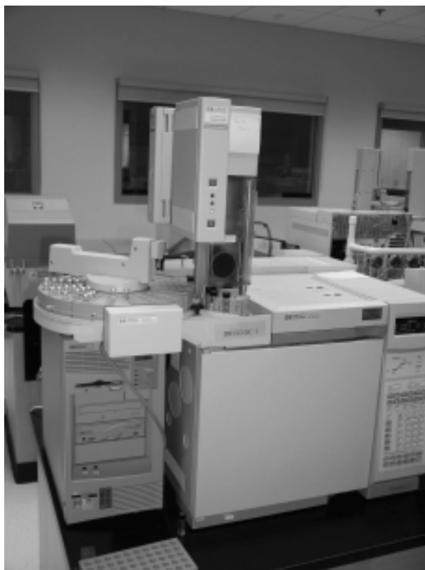
FIGURE G.2 The gas chromatography separates compounds by their size, shape, and reactivity with the chemical coating of the GC column. This GC has a robotic arm and a carousel so the instrument can automatically inject the samples from the glass vials into the column.
