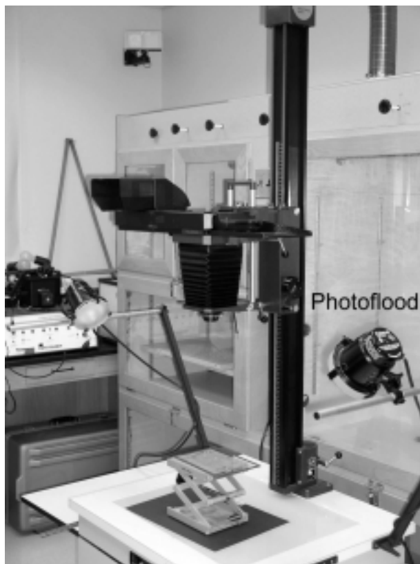
FIGURE P.6 A photoflood lamp setup with an overhead camera. The photoflood lamps provide the needed lighting for taking pictures.
