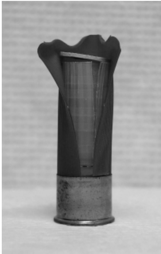
FIGURE S.5A Opening of a shotshell showing the inside.
