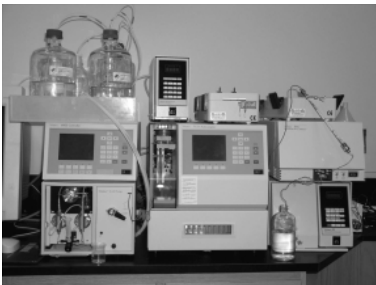
FIGURE L.4 The LCMS utilizes a closed system and pumps to pressurize the solvent (mobile phase) and to force the liquid through the column.
