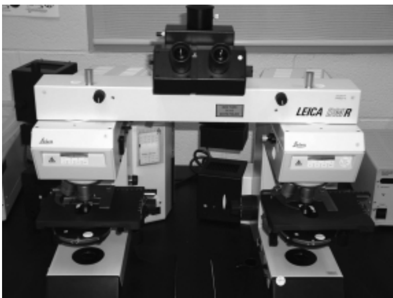
FIGURE S.13A Comparison microscope used to compare latent fingerprints lifted from crime scene to suspect's fingerprint cards.
