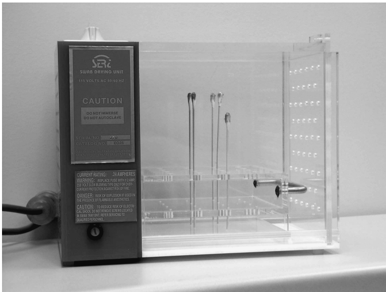
FIGURE S.18 A container for storing wet swabs. Air is then circulated through the container, which will allow the swabs to air dry. The container prevents contamination of the swabs as they are drying.
