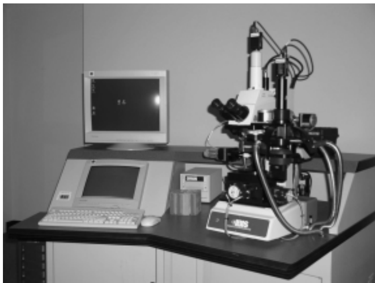
FIGURE I.1 Workstation for the IBIS, including computer and microscope.
