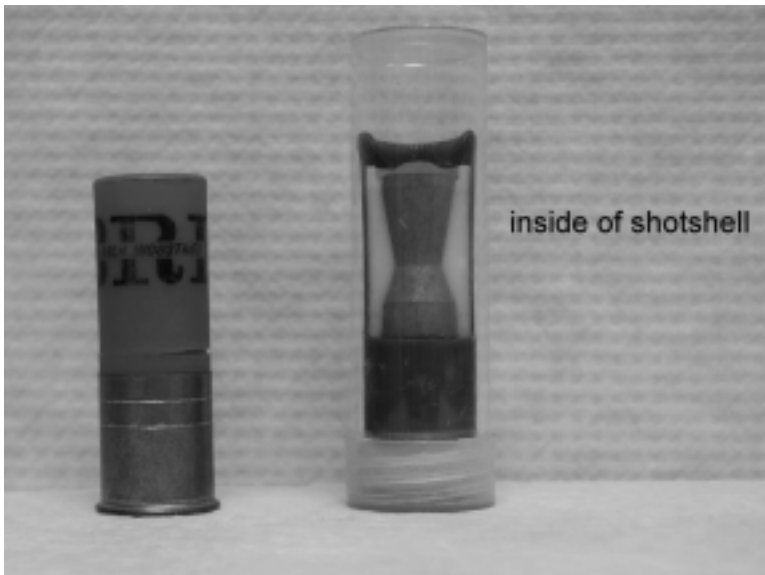
FIGURE S.5B Cut away section of a shotshell.
