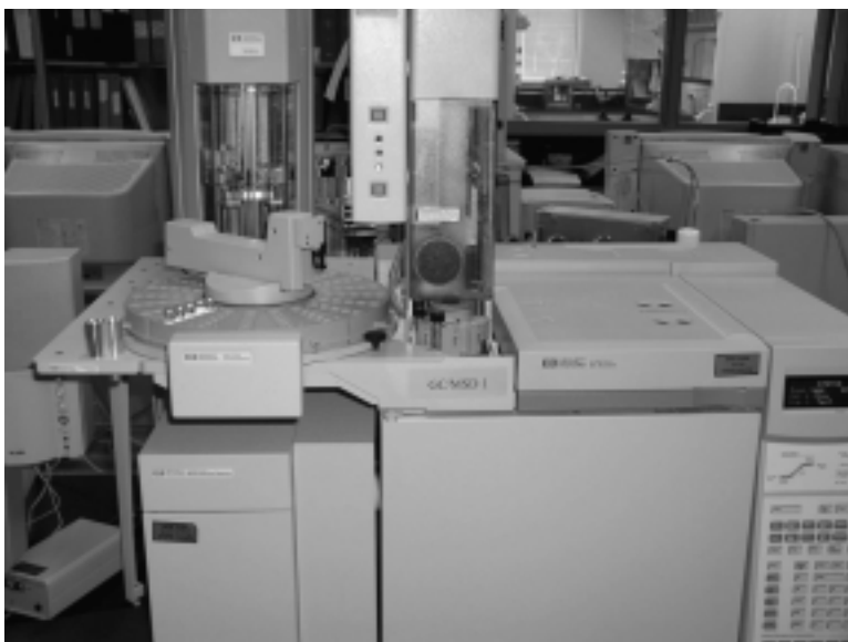
FIGURE G.5 GC/MS instrument. The gas chromatography (GC) instrument separates the compounds, and the mass spectroscopy (MS) provides information concerning the chemical properties of each of the compounds as it elutes from the chromatographic column.
