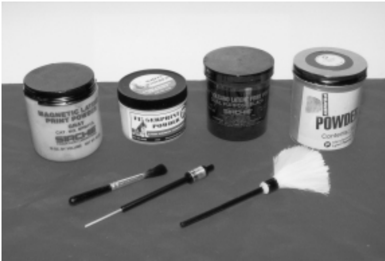
FIGURE F.3 Different types of fingerprint dust powder and brushes.
