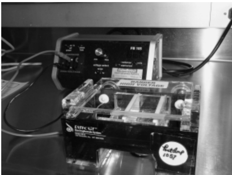
FIGURE G.6 Gel electrophoresis unit with power supply unit.
