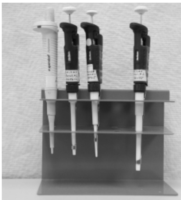
FIGURE M.7 Handheld mechanical pipettes that can deliver a specific volume of liquid. Each pipette contains an adjustable dial that can be set for a specific volume measured in microliters.
