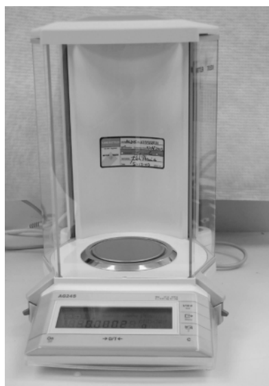
FIGURE A.3 Analytical balances used for measuring reagents, dry chemicals, and for measuring the accuracy of manual pipettes (the amount of fluid dispensed).
