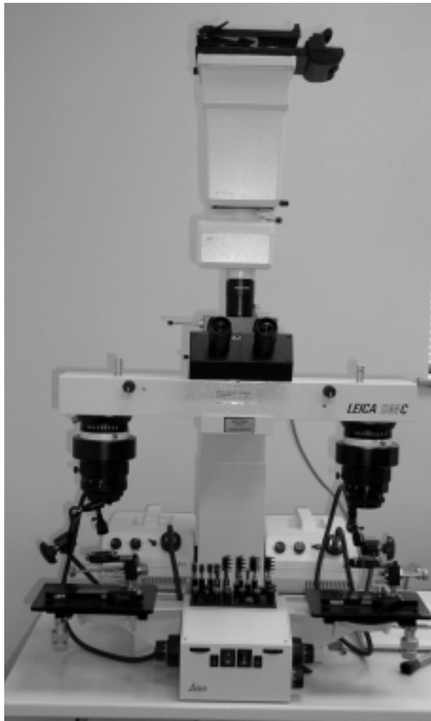
FIGURE C.17 A firearms examiner's (ballistics) comparison microscope. It has an optical bridge, separate objectives, dual focusing stages, specimen holders, and two illuminators, the angles and intensities of which are independently adjustable.
