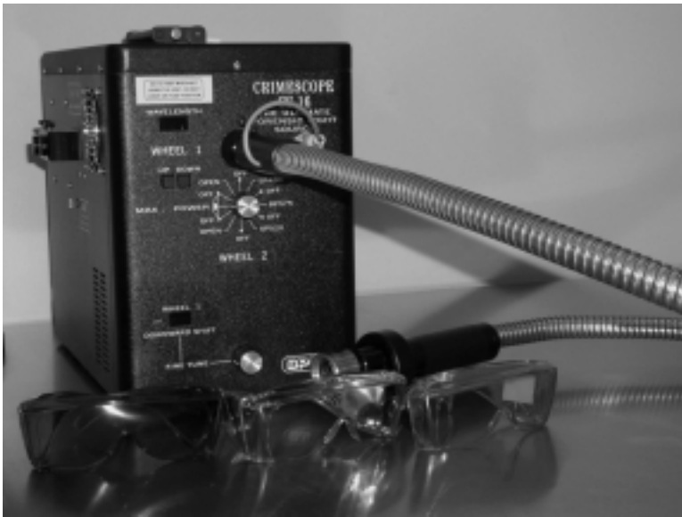
FIGURE C.22 An alternate light source made by SPEX® uses different wavelengths of light. With special color glasses one can observe various types of stains found on evidence.
