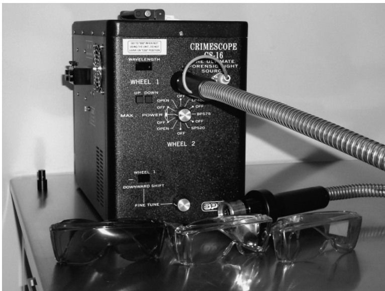
FIGURE A.1 An alternate light source manufactured by SPEX®.
