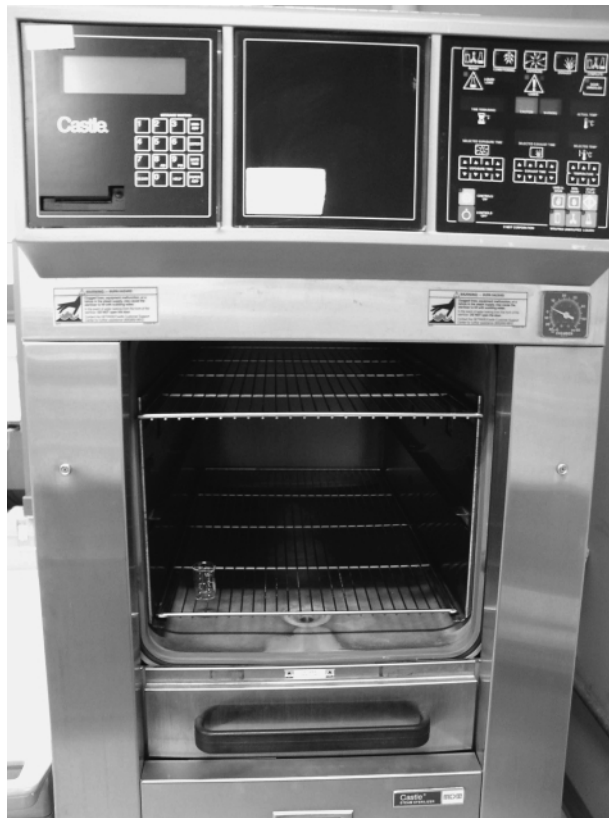
FIGURE A.10 An enclosed chamber for the sterilization under pressure of laboratory glassware, instruments, plastic tubes, etc.
