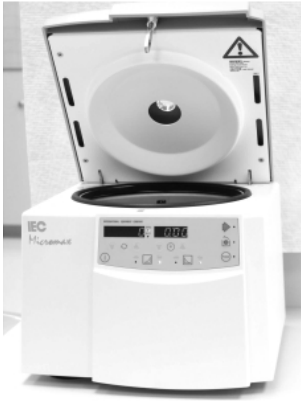
FIGURE C.7 A rotary machine with accessory containers, tubes, and rotors for the separation by controlled centrifugal force of substances having different densities.
