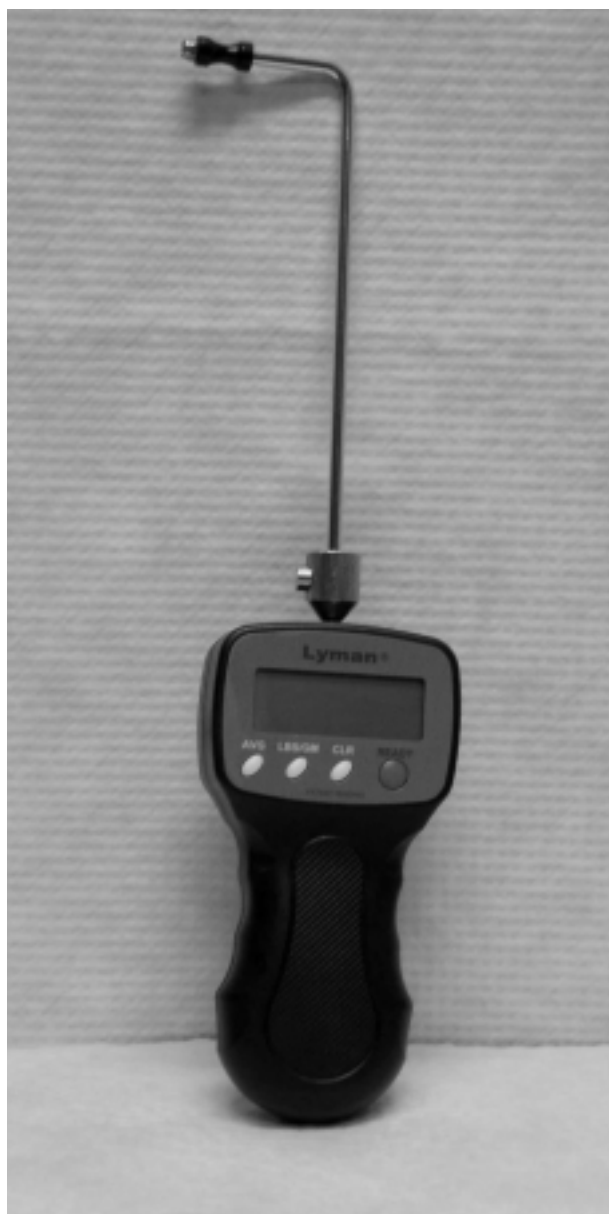
FIGURE T.9B A handheld trigger pull gauge with a digital readout.
