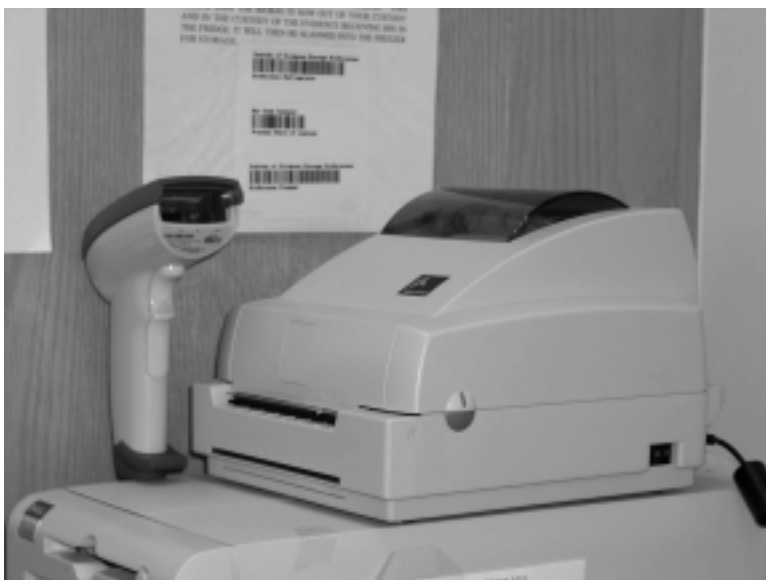
FIGURE L.6 The LIMS uses a bar code method for the identification of evidence. The picture shows the bar code labelmaker and a handheld scanner.
