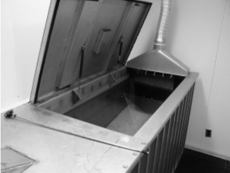
FIGURE B.9 A metal tank filled with water allowing the firearm examiner to recover bullets from the test firing of handguns.
