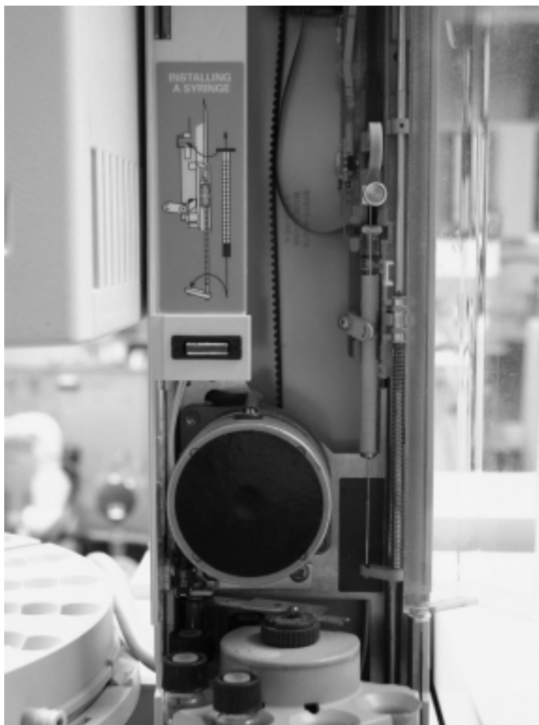
FIGURE I.4 Injection port uses a syringe to automatically aspirate the sample from the vial and inject the sample into the column of the GC/MS instrument.
