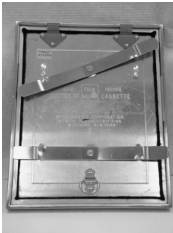
FIGURE C.4 A metal case that is lightproof. It is used for the development of the autoradiograph.
