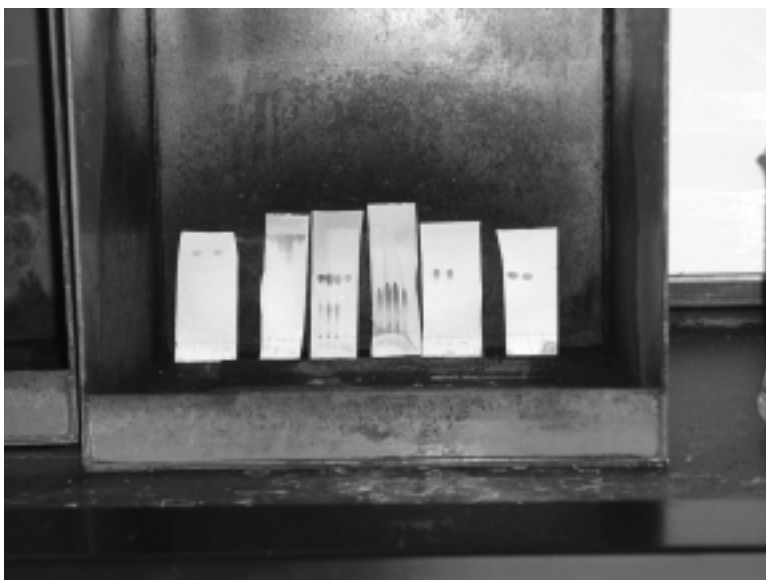
FIGURE T.4 Drug chemistry spraying chamber on TLC plates.
