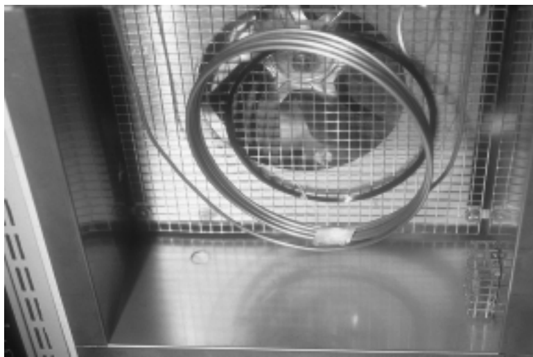
FIGURE P.1 Inert material packed into capillary columns used in gas chromatography.
