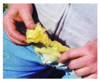
The 40-layered Kevlar pad is light, thin and pliable. After four months in one of Davis' boots, it was little the worse for wear because Kevlar quickly conformed to individual foot contours.
