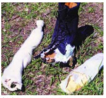
(below) Effects on boot and simulated foot by two ounces of HE are graphic: Amost half the boot is destroyed. In contrast, the sock (filled with wet sand and half a dozen wooden stakes to simulate human bones and protected by Davis' Kevlar pad), though slightly damaged, remained intact. In a real AP mine blast with this measure of Kevlar protection, a man's foot would almost certainly be broken, but victim wouldn't lose the foot, as is usually the case with small AP mines like the Russian PMN.
