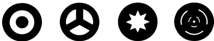
Figure 224. Cross-sections of propellant grains which burn with a constant surface area.
