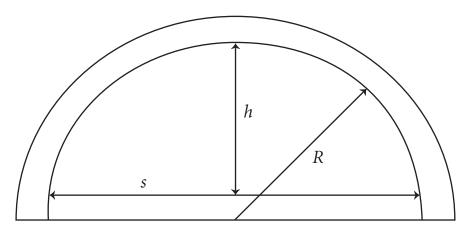
The formula  $s^2 = 8Rh - 4h^2$  gives the relationship between the center height (*h*) of the arch, the radius of curvature (*R*) of the arch, and the distance (*s*) spanned by the arch.
