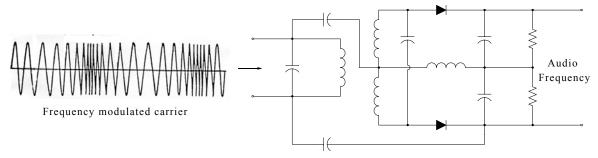
Figure 2.55. Foster-Seely discriminator circuit
