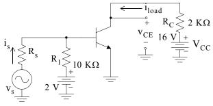
Figure 3.62. Transistor amplifier for Example 3.15
