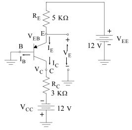
Figure 3.17. PNP transistor for Example 3.7
