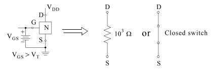
Figure 6.47. Condition under which an NMOS device behaves as a closed switch
