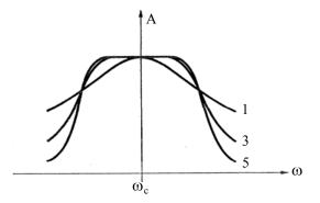
Figure 9.16. Maximally flat multistage tuned amplifiers
