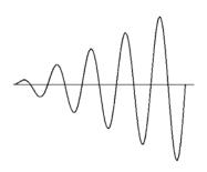
Figure 1.15. Characteristics of an unstable system
