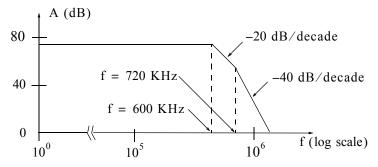
Figure 8.16. Asymptotes for the high-frequency characteristics of the amplifier for Example 8.7
