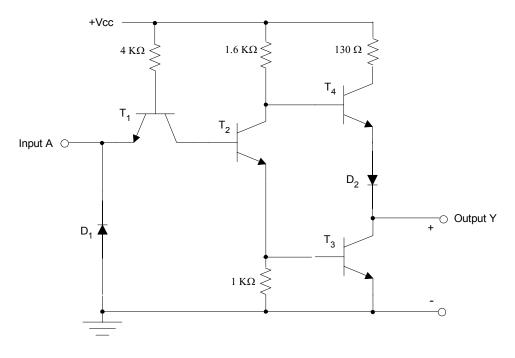
Figure 6.8. Circuit of the SN7404 Inverter
