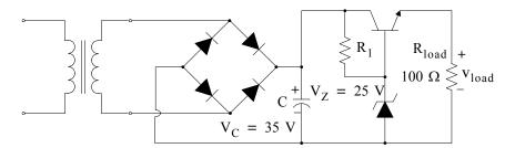
Figure 3.56. DC power supply for Example 3.14
