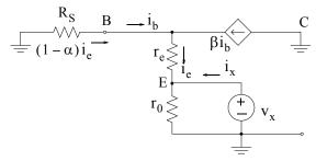
Figure 3.82. Equivalent circuit for the computation of the output resistance
