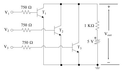
Write the truth table for the input combinations of 0 V and 5 V with respect to the ground. Which type of logic gate does this circuit represent?
