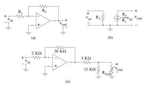
6. For the circuit below compute  $v_{5K\Omega}$  using Thevenin's theorem.
