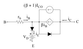
Figure 3.52. A more accurate model for the transistor
