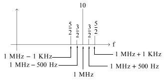
Figure 9.4. Frequency spectrum for Example 9.1
