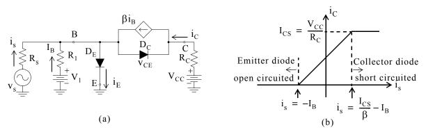
Figure 3.55. Piecewise linear model for the circuit of figure 3.53 and its current transfer characteristics
