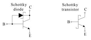
Figure 6.64. Bipolar NPN transistor with Schottky diode and its representation as Schottky transistor
