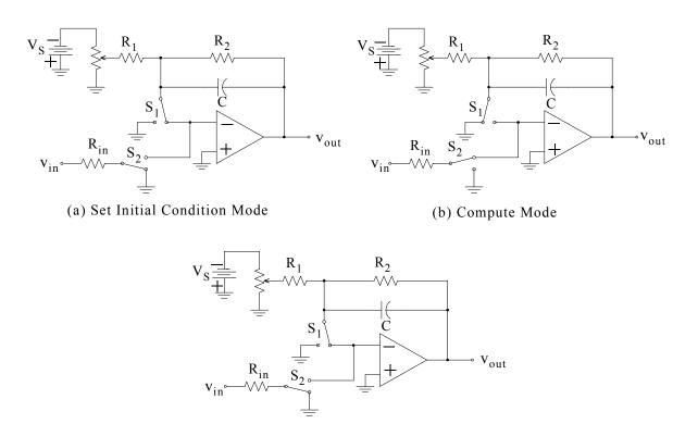
(c) Hold Mode Figure 5.94. Integrator circuit mode control
