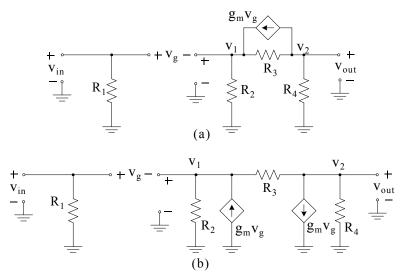
Figure 8.4. Equivalent circuits for Example 8.2
