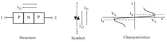
Figure 4.23. Diac structure, symbol, and characteristics
