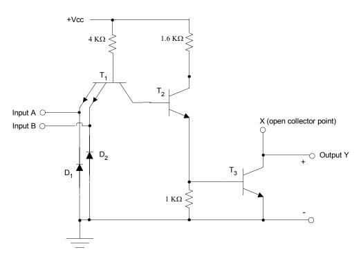
Figure 6.32. Open-collector TTL configuration
