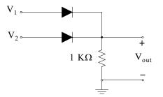
Write the truth table for the input combinations of 0 V and 5 V with respect to the ground. Which type of logic gate does this circuit represent?
