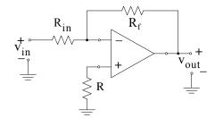
Figure 5.3. Circuit of inverting op amp
