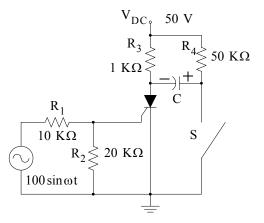
a. Just before the switch closes, the voltage drop across the SCR is 1 V and the voltage drop across the capacitor is 49 V with the polarity as shown. The capacitor voltage cannot change instantaneously so immediately after the switch is closed, the capacitor voltage will be -49 V as shown in the figure below, and the SCR will be Off.
