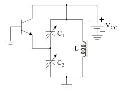
Figure 10.7. Simplified circuit for the Colpitts oscillator
