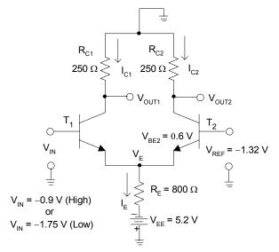
Figure 6.41. Basic ECL circuit
