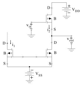
Figure 4.20. Typical common-drain (source follower) amplifier
