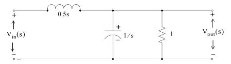
Figure 1.12. Circuit of Example 1.2 in the *s* – *domain*
