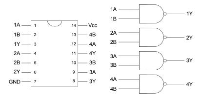
Figure 6.18. The SN7400 Quad 2-input NAND gate
