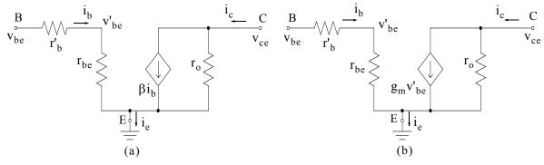
Figure 3.65. Alternative forms for the transistor model
