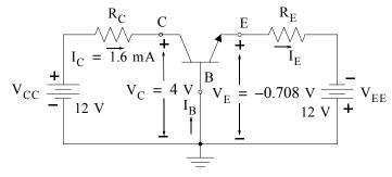
Figure 3.10. Transistor circuit for Example 3.3 - Computations for  ${\rm R}_{\rm E}$
