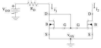
Figure 4.17. Typical circuit of a current mirror
