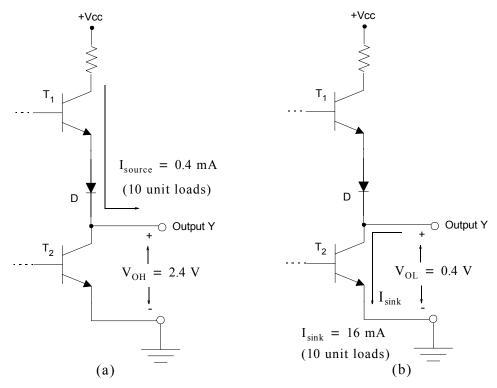
Figure 6.31. Current sourcing and current sinking
