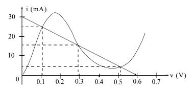
Figure 2.73. Graphical solution for the determination of the current i for the circuit of Figure 2.72
