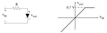
Figure 2.42. Circuit where  $v_{out}$  =  $v_{in}$  when diode does not conduct and  $v_{out} \approx 0.7~V$  when  $v_{in} \ge 0.7~V$
