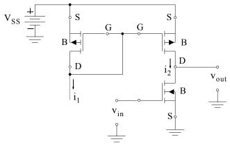
Figure 4.18. Typical CMOS common-source amplifier
