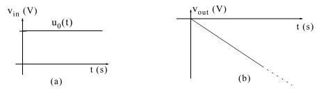
Figure 5.55. The output voltage of the circuit of Figure 5.57(a) when the input is the unit step function
