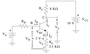
Figure 3.16. Circuit for Example 3.6
