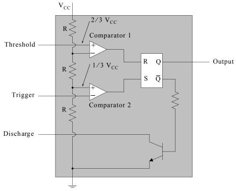
Figure 7.4. Simplified circuit for the 555 Timer
