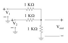
a. With  $V_1 = V_2 = 0$  V,  $V_{out} = 0$  V. With  $V_1 = 0$  V, and  $V_2 = 5$  V,  $R_1$  is in parallel with  $R_3$  and by the voltage division expression
