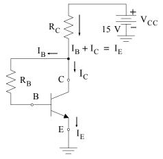
Figure 3.30. Circuit for Example 3.10 with assigned current directions
