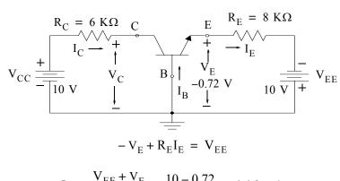
$$I_E = \frac{V_{EE} + V_E}{R_E} = \frac{10 - 0.72}{8 \times 10^3} = 1.16 \text{ mA}$$
