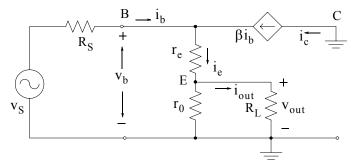
Figure 3.81. The simplified common-collector transistor amplifier equivalent circuit
