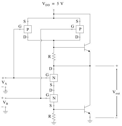
Figure 6.68. The basic BiCMOS NAND gate
