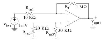
Figure 5.31. Circuit for Example 5.10 with  $v_{in1}$  acting alone
