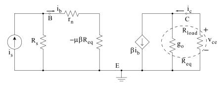
Figure 3.61. The circuit of Figure 3.60 with the voltage source  $\mu v_{ce}$  replaced by the resistance  $-\mu\beta R_{eq}$
