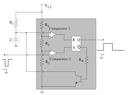
Figure 7.21. A monostable multivibrator using a 555 timer circuit.
