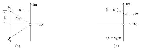
Figure 9.10. Graphical representation of the relations  $s_1 = -\alpha + j\beta$ ,  $s_2 = -\alpha - j\beta$ , and  $\beta^2 = \alpha^2 - \omega_0^2$
