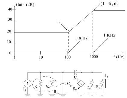
Figure 8.28. Simplified model of the transistor amplifier for Example 8.6
