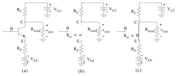
Figure 3.31. Simple amplifier with resistive load
