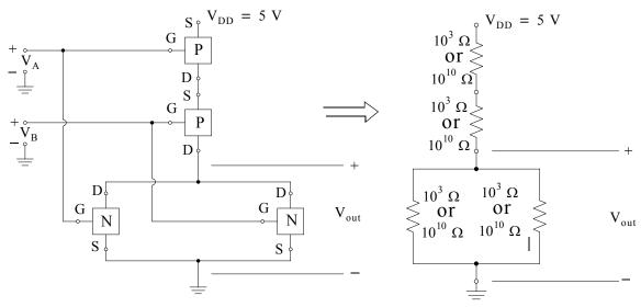
Figure 6.55. 2-input CMOS NOR gate
