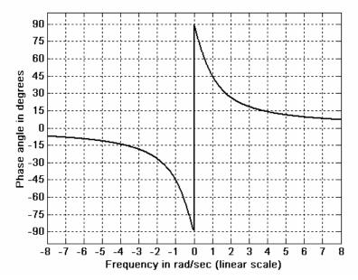
Figure 1.25. Phase characteristics of an RC high-pass filter with RC = 12. We draw the s – domain equivalent shown below.
