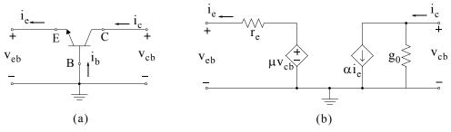
Figure 3.68. Common-base transistor circuit and its equivalent
