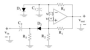
Figure 7.20. A monostable multivibrator using an op amp
