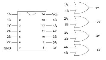
Figure 6.15. The SN7432 Quad 2-input OR gate
