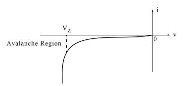
Figure 2.13. The reverse biased region of a junction diode
