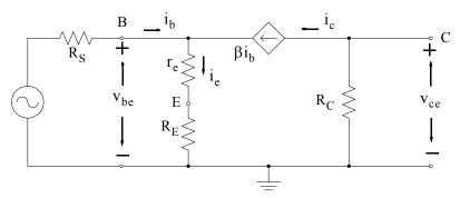
Figure 3.76. The simplified common-emitter transistor equivalent circuit
