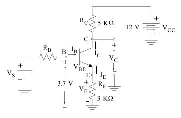
Since  $V_B = 3.7$  V it is reasonable to assume that the base-emitter junction is forward-biased and thus  $V_{BE} = 0.7$  V. Then,
