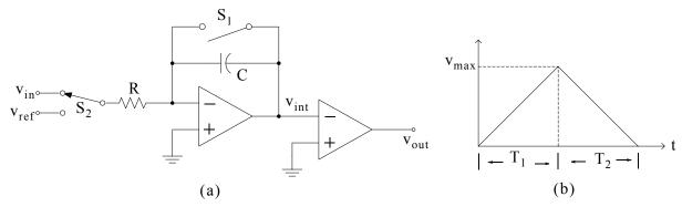
Figure 5.91. An ADC with dual-slope architecture
