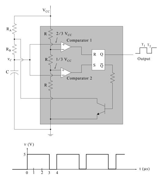
2. For the astable multivibrator below  $V_{CC} = 5 \text{ V}$  and C = 1 nF. Find the values for the resistors  $R_A$  and  $R_B$  so that the circuit will produce the waveform shown.
