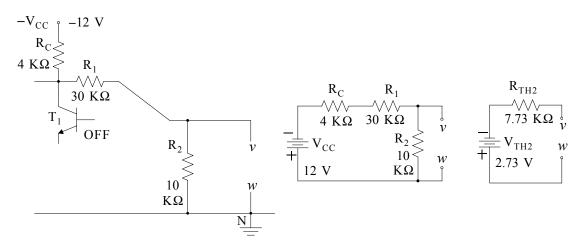
Figure 7.30. Base circuit for the computation of Thevenin equivalent, Example 7.5 From Figure 7.30
