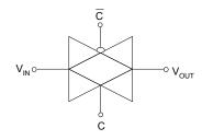
Figure 6.62. Symbol for the CMOS transmission gate
