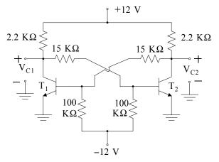
Figure 7.23. Fixed-bias flip-flop circuit for Example 7.4.
