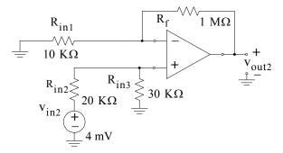
Figure 5.32. Circuit for Example 5.10 with  $v_{in2}$  acting alone
