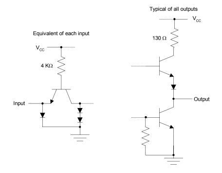
Figure 6.28. Circuit for the SN7486 XOR gate
