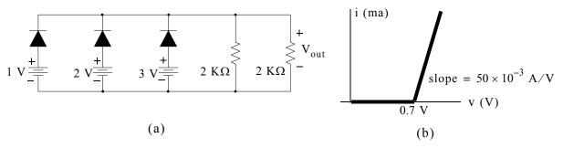
Figure 2.22. Circuit and piecewise linear i – v characteristics for Example 2.4
