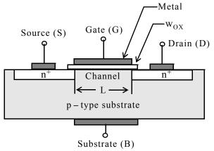
Figure 4.8. Cross section of an n-channel MOSFET
