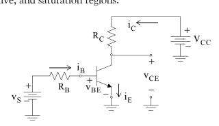
Figure 3.85. Transistor circuit for defining the regions of operation
