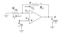
Figure 5.22. Non-inverting op amp circuit for derivation of (5.4)
