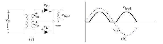
Figure 2.36. Full-wave rectifier with centered tapped secondary winding
