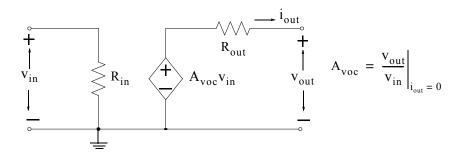
Figure 1.19. Circuit model for voltage amplifier where  $A_{voc}$  denotes the open circuit voltage gain The ideal characteristics for the circuit of Figure 1.19 are  $R_{in} \rightarrow \infty$  and  $R_{out} \rightarrow 0$ .
