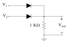
By inspection, when  $V_1 = V_2 = 0 V$ , the output is  $V_{out} = 0 V$ . When  $V_1 = 0 V$  and  $V_2 = 5 V$ , or  $V_1 = 5 V$  and  $V_2 = 0 V$ , or  $V_1 = V_2 = 5 V$ , one or both diodes conduct and the output is  $V_{out} = 5.0 - 0.7 = 4.3 V$  and thus the truth table is as shown below.
