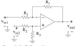
Figure 5.63. Differential input op amp
