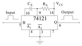
Figure 7.18. The 74121 monostable multivibrator
