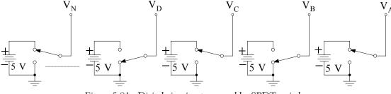
Figure 5.81. Digital circuit represented by SPDT switches
