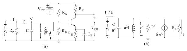
Figure 9.7. Impedance transformation in a tuned transistor amplifier and its model
