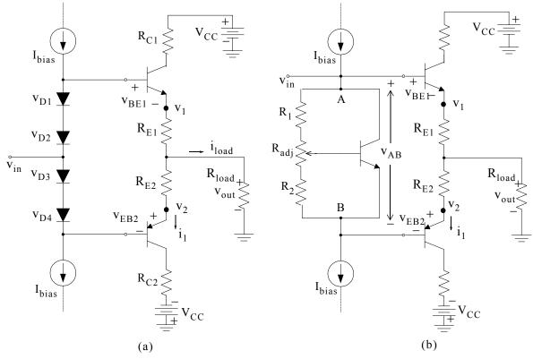
Figure 3.40. Two possible arrangements for the output stage of a typical Class AB amplifier For sinusoidal signals into the load  $R_{load}$ , the RMS voltage will be
