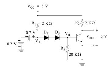
With  $V_A = 0.2 V + 0.7 V = 0.9 V$ , the transistor is OFF. For the transistor to be ON, the voltage  $V_A$  with respect to the ground would have to be
