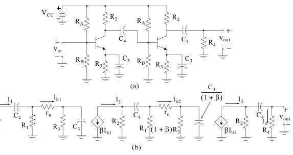
Figure 8.18. Cascaded amplifier circuit and its low-frequency equivalent for Example 8.8.
