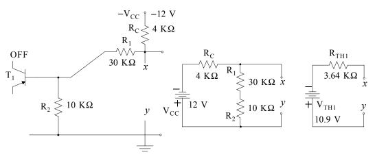
Figure 7.29. Collector circuit for the computation of Thevenin equivalent, Example 7.5 From Figure 7.29
