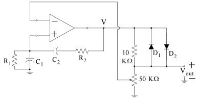
Figure 5.79. The Wien bridge oscillator
