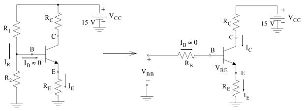
Figure 3.27. The transistor circuit of Example 3.9 and its Thevenin equivalent
