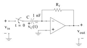
Figure 5.59. Differentiator circuit for Example 5.19
