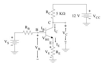
7. For the circuit below,  $\beta = 150$ . Find  $I_E$ ,  $V_E$ ,  $I_C$ ,  $V_C$ ,  $I_B$ , and determine whether this circuit with the indicated values operates in the active, saturation, or cutoff mode. Hint: The base-to-emitter junction of an NPN transistor is considered to be reverse-biased if  $V_B = V_E = 0$
