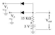
Write the truth table for the input combinations of 0 V and 3 V with respect to the ground. Which type of logic gate does this circuit represent?
