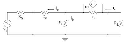
Figure 3.72. T-equivalent model for the common-base transistor
