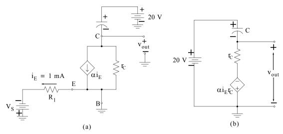
Figure 4.34. Piecewise-linear and equivalent circuits for the sawtooth generator of Figure 4.33
