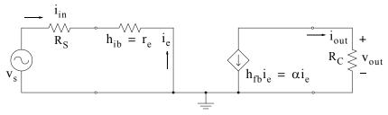
Figure 3.71. Simplified circuit for the computation of voltage gain in a common base transistor From Figure 3.71,
