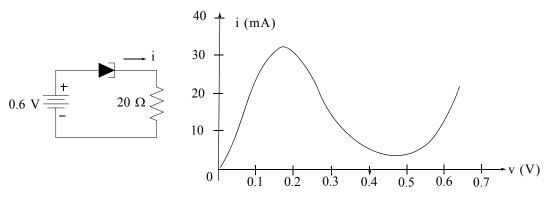
Figure 2.72. Circuit and tunnel diode i - v characteristics for Example 2.12
