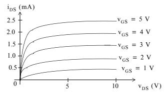
Figure 4.10. Current-voltage characteristics for typical MOSFET
