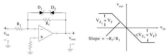
Figure 5.73. A positive and negative voltage limiter circuit and its transfer characteristics
