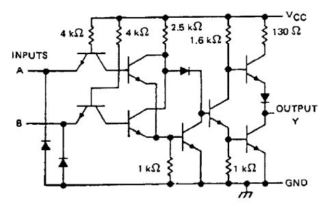
Figure 6.16. Circuit for the SN7432 Quad 2-input OR gate (Courtesy Texas Instruments)
