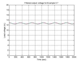
Figure 2.39. Voltage across the 2 K $\Omega$  resistor in Figure 2.36
