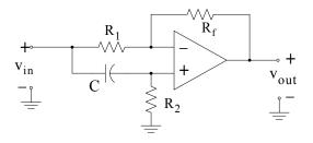
20. The circuit below is referred to as a *differential input integrator*. The resistors and capacitors are of equal value. Derive an expression for  $V_{out}(s)$  in terms of the input voltages and the circuit constants.
