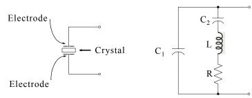
Figure 10.8. Symbol and equivalent circuit for a crystal
