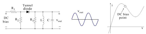
Figure 2.71. Tunnel diode oscillator circuit
