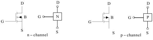
Figure 6.45. Designations for n- and p-channel MOSFETS
