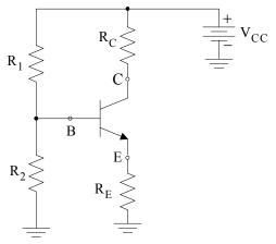
Figure 3.23. NPN Transistor with fixed bias
