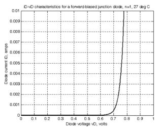
Figure 2.12. Voltage-current characteristics of a forward-biased junction diode.
