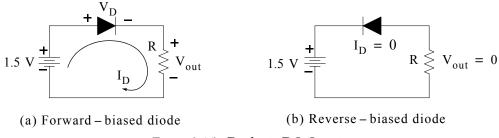
Figure 2.15. Diodes in DC Circuits
