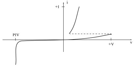
Figure 4.25. The voltage-current characteristics of a typical SCR
