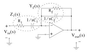
Figure 5.51. The s - domain equivalent circuit of Figure 5.50
