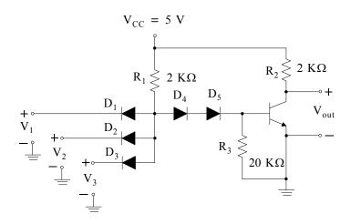
With one or more of the inputs  $V_1$ ,  $V_2$ , or  $V_3$  at 0 V, the given circuit becomes as shown below where the 0.2 V is assumed to be the output of a previous logic gate with logical 0.
