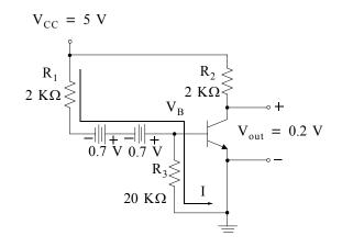
To determine the output voltage  $V_{OUT}$  we need to find out whether the transistor is ON or OFF. Let us assume that it is OFF. Then, by KVL
