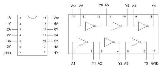
Figure 6.6. The SN7404 Hex Inverter IC
