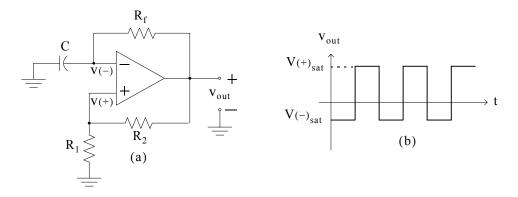
Figure 7.16. Unstable multivibrator circuit for Example 7.3
