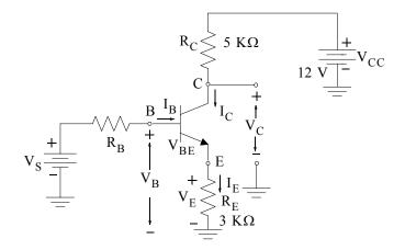
The transistor will be in the active mode for  $V_B > 0.7V$  and for  $V_B \le V_C$ . Since  $\beta = 110$ ,
