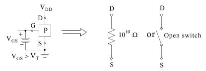
Figure 6.48. Condition under which a PMOS device behaves as an open switch
