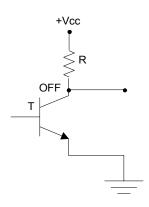
Figure 6.30. A passive pull-up circuit.
