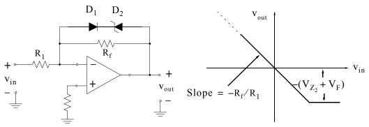
Figure 5.75. A negative voltage limiter circuit and its transfer characteristics
