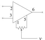
Figure 5.68. Offset nulling terminals of the 741 op amp
