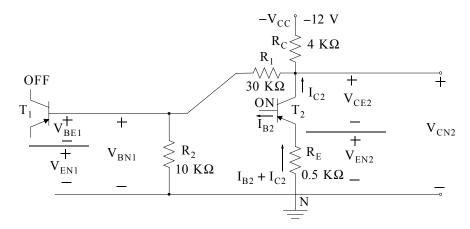
Figure 7.27. The circuit of Example 7.5 showing the connections between the base of  $T_1$  and collector of  $T_2$
