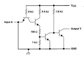
Figure 6.58. Circuit for the IC SN7407/SN7417 buffer (Courtesy of Texas Instruments)
