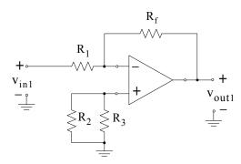
Figure 5.64. The circuit of Figure 5.63 with  $v_{in1}$  acting alone
