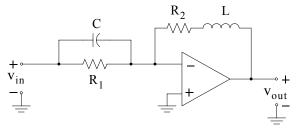
26. For the op amp circuit shown below, derive an expression for the output voltage  $v_{out}$  in terms of the input voltage  $v_{in}$ .
