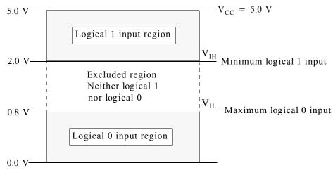
Figure 6.35. Valid logical 1 and valid logical 0 input regions for a typical IC gate
