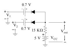
By inspection, when  $V_1 = V_2 = 0 V$ , or  $V_1 = 0 V$  and  $V_2 = 3 V$ , or  $V_1 = 3 V$  and  $V_2 = 0 V$ , the output is  $V_{out} = 0.7 V$ . When  $V_1 = V_2 = 3 V$ , the output is  $V_{out} = 3.7 V$  and thus the truth table is as shown below.
