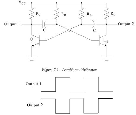
Figure 7.2. Output waveforms of the astable multivibrator
