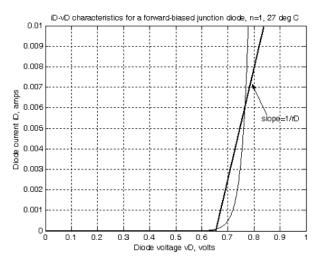
Figure 2.19. Straight lines for forward-biased diode characteristics approximations
