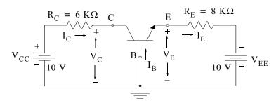
4. For the PNP transistor circuit below, it is known that  $R_B = 130 \text{ K}\Omega$ ,  $V_E = 2 \text{ V}$  and  $V_{EB} = 0.7 \text{ V}$ . Find  $\alpha$ ,  $\beta$ , and  $V_C$ . The circuit operates at T = 27 °C.
