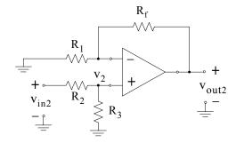
Figure 5.65. The circuit of Figure 5.67 with  $v_{in2}$  acting alone
