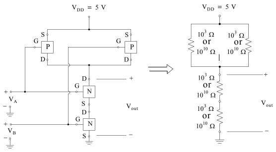
Figure 6.54. 2-input CMOS NAND gate
