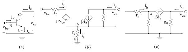
Figure 3.73. Common-emitter transistor circuit and its equivalent
