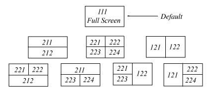
Figure A.7. Possible subplot arrangements in MATLAB
