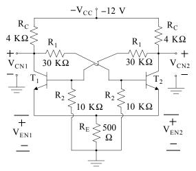
Figure 7.26. Self-bias flip-flop circuit for Example 7.5
