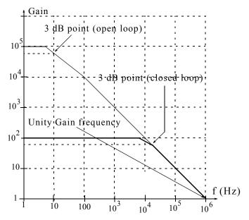
Figure 5.43. Closed-loop frequency response for a gain of 100
