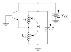
Figure 10.6. Simplified circuit for the Hartley oscillator
