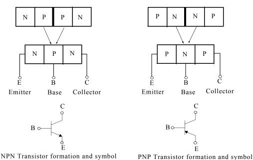
Figure 3.1. NPN and PNP transistor construction and symbols
