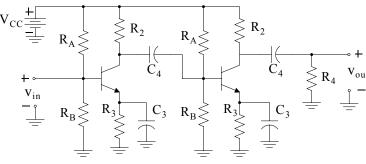
Figure 8.15. Cascaded amplifier for Example 8.7
