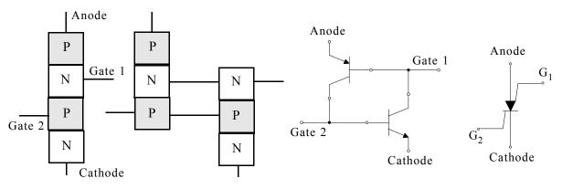
Figure 4.39. Parts of an SCS, the two-transistor equivalent circuit, and its symbol
