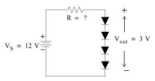
Since the diodes are identical, for the output voltage to be  $V_{out} = 3 V$ , the voltage drop across each diode must be 3 V/4 = 0.75 V, and since the change is  $\Delta V_D = 0.75 - 0.65 = 0.1 V$ , the current  $0.5 \times 10 = 5 \text{ mA}$ . Then,
