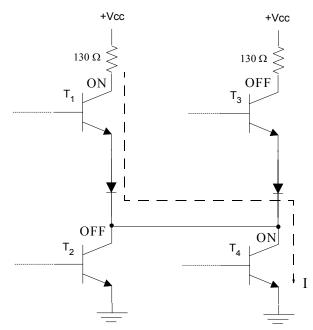
Figure 6.34. Improper wired AND connection
