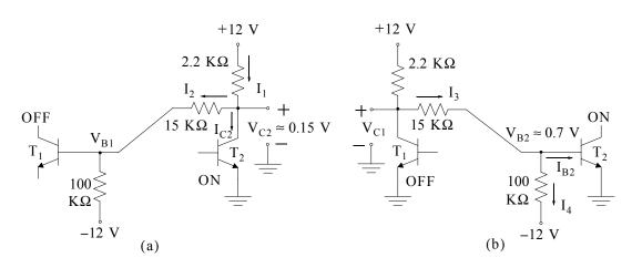
Let us first assume that transistor  $T_1$  is OFF and transistor  $T_2$  is ON. By the voltage division expression and the superposition principle,
