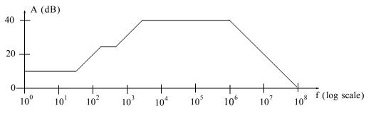
Figure 8.13. Combined low- and high-frequency amplitude versus frequency characteristics
