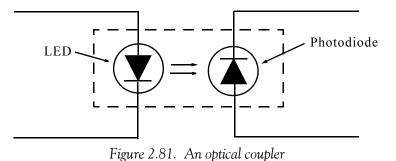
Isolation between the input and output is desirable because it reduces electromagnetic interference. Their most important application is in fiber optic communications links.
