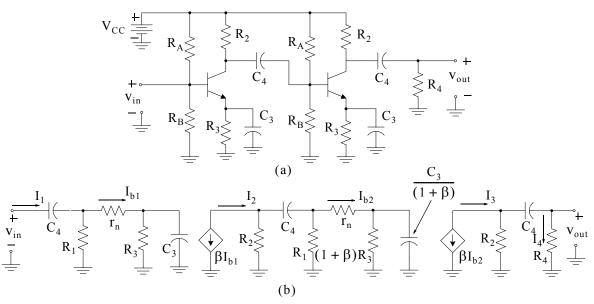
Figure 8.17. RC-coupled amplifier circuit and its model at low frequencies
