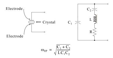
This is a parallel circuit and thus the resonant frequency occurs when the imaginary part of the admittance Y is equal to zero. Therefore,
