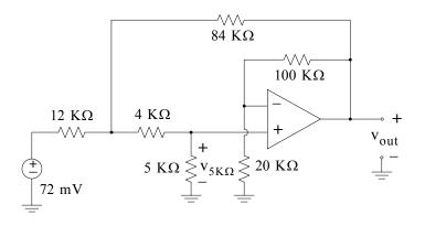
7. For the circuit below compute the gain  $G_v = v_{out}/v_{in}$ .
