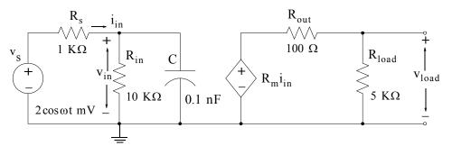
Find the overall voltage gain  $A_v$  =  $v_{load}/v_s$  if  $R_m$  = 100  $\Omega.$  Then, use MATLAB to plot the
