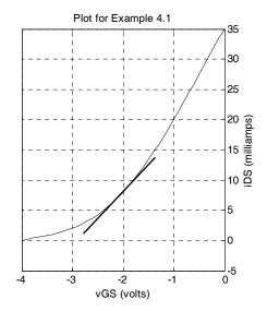
Figure 4.7. MATLAB generated plot for Example 4.1
