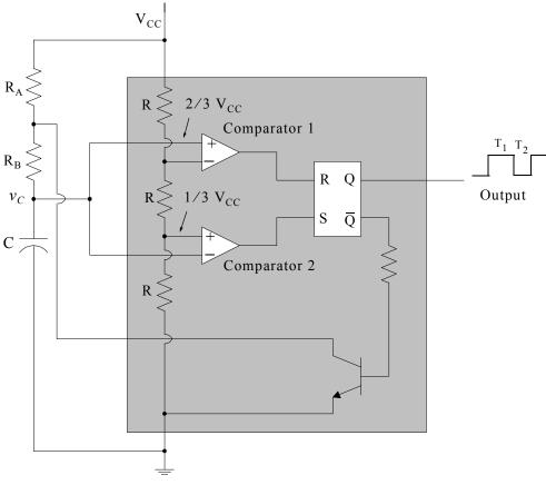
Figure 7.10. Astable multivibrator for Example 7.1
