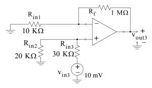
Figure 5.34. Circuit for Example 5.10 with  $v_{in3}$  acting alone
