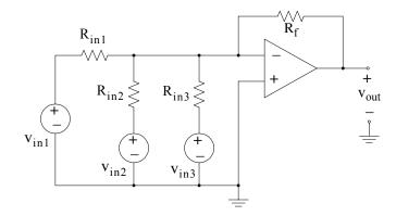
4. For the circuit below compute  $v_{out}$ .
