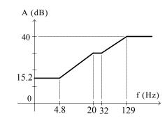
Figure 8.25. Logarithmic amplitude characteristic for Example 8.7
