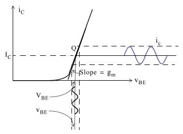
Figure 3.64. The transconductance  $\boldsymbol{g}_{m}$  defined
