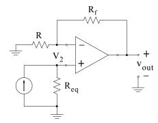
Figure 5.62. Equivalent circuit for the circuit of Figure 5.61
