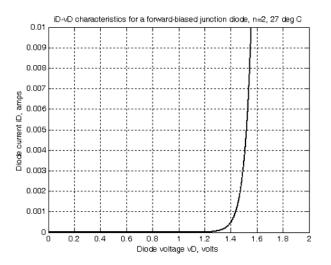
We observe that when n = 2, the diode begins to conduct at approximately 1.3 V.
