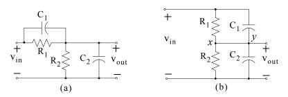
Figure B.2. A compensated attenuator and its equivalent drawn as a bridge
