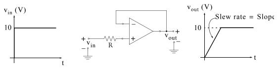
Figure 5.71. The resultant slew rate when a step function is applied to a unity gain op amp
