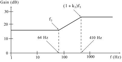
Figure 8.6. Amplitude characteristic for the amplifier of Example 8.3
