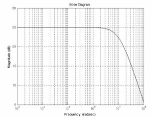
Figure 1.22. Bode plot for the voltage amplifier of Example 1.5
