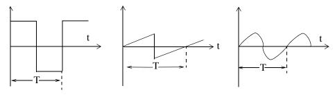
Figure 1.3. Examples of alternating waveforms
