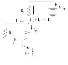
Figure 3.28. NPN transistor amplifier with self-bias
