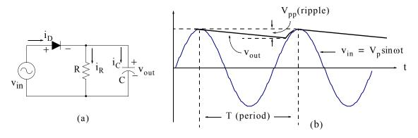
Figure 2.41. Peak rectifier used as an AC to DC converter
