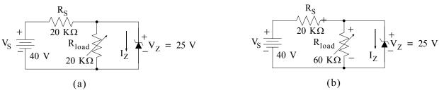
Figure 2.59. Circuits for Example 2.10 with Zener diodes to improve regulation
