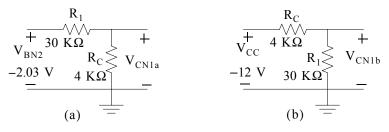
Figure 7.32. Circuits for the computation of  $V_{CN1}$ , Example 7.4
