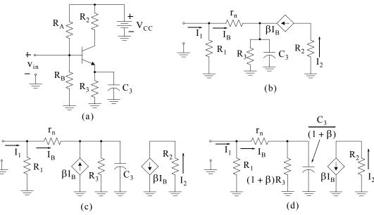
Figure 8.5. Transistor amplifier and equivalent circuits at low frequencies
