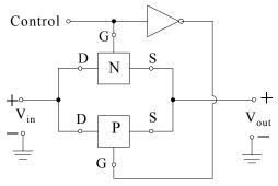
Figure 6.61. The CMOS transmission gate
