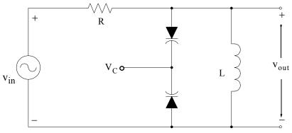
Figure 2.75. A varactor tuner circuit
