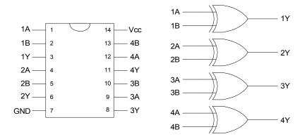
Figure 6.27. The TTL SN7486 Quad XOR gate
