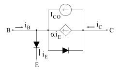
Figure 3.50. A transistor model
