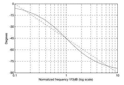
The plot above shows that the  $f_{3 dB} = 1$  KHz frequency occurs at  $\theta = -45^{\circ}$  and the asymptotic (dotted) line indicates that it drops at the rate of  $45^{\circ}/(\text{decade})$ . Therefore, the phase at 100 KHz is  $-90^{\circ}$  and because this is an inverting amplifier, we must add  $-180^{\circ}$  so the total phase shift is  $-270^{\circ}$  or  $+90^{\circ}$ .
