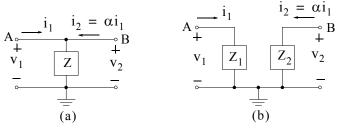
Figure C.16. Illustration for Miller's dual theorem
