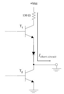
Figure 6.38. The definition of the output short-circuit current
