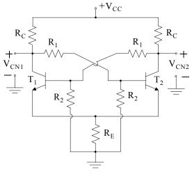
Figure 7.25. Self-bias flip-flop circuit
