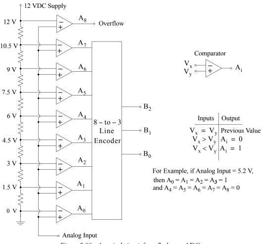
Figure 5.88. A typical circuit for a flash type ADC
