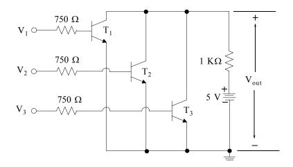
By inspection, when  $V_1 = V_2 = V_3 = 0$  V, none of the three transistors conduct and thus  $V_{out} = 5$  V. When one or more of the input voltages is 5 V one or more of the transistors will saturate and the output will be  $V_{out} = 0.2$  V  $\approx 0$  V. The truth table is as shown below and thus this circuit behaves as a 3-input NOR gate.
