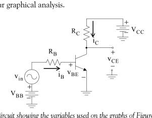
Figure 3.42. Circuit showing the variables used on the graphs of Figures 3.43 and 3.44
