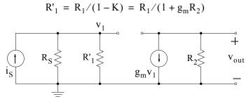
Figure C.18. Miller equivalent circuit for the circuit of Figure C.17
