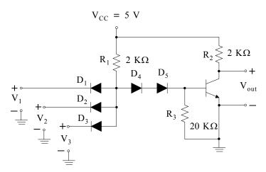
Write the truth table for the input combinations of 0 V and 5 V with respect to the ground. Which type of logic gate does this circuit represent?
