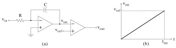
Figure 5.90. An ADC with single-slope architecture
