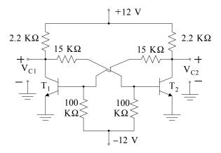
The transistors are identical and the curves supplied by the manufacturer specify that  $V_{CE2}(sat) = 0.15$  V and  $V_{BE2}(sat) = 0.7$  V. Assume that the transistors have a minimum  $h_{FE}$  value of 50. Using these voltages, recalculate the stable-state currents and voltages.
