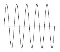
Figure 1.14. Characteristics of a marginally stable system
