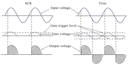
Figure 4.37. Comparison of SCR and Triac waveforms
