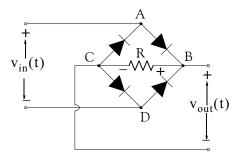
Figure 2.32. Full-wave rectifier circuit
