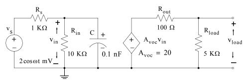
Figure 1.20. Amplifier circuit for Example 1.5
