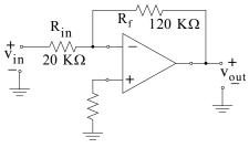
Figure 5.4. Circuit for Example 5.1
