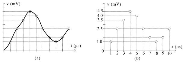
Figure 5.92. An analog voltage quantized in time and amplitude
