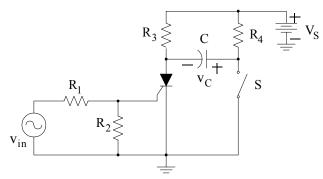
Figure 4.27. A switching circuit using an SCR
