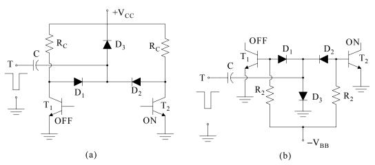
Figure 7.35. Methods of symmetrical triggering through diodes at the collectors or the bases of the transistors
