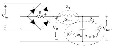
Figure 2.38. Phasor equivalent circuit for Example 2.7
