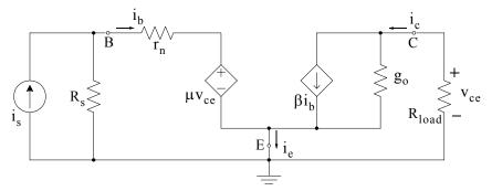
Figure 3.60. Transistor incremental model with external devices
