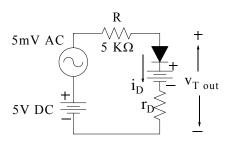
Figure 2.26. The piecewise linear equivalent of the circuit of Example 2.5
