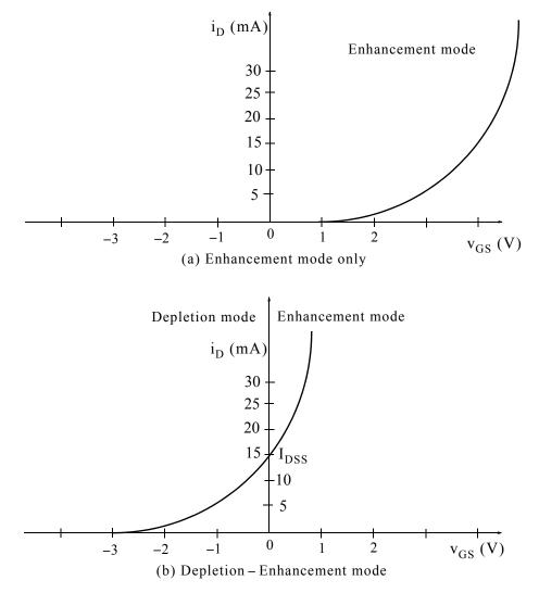
Figure 4.13. Typical n – channel MOSFET  $i_D$  vs  $v_{GS}$  characteristics
