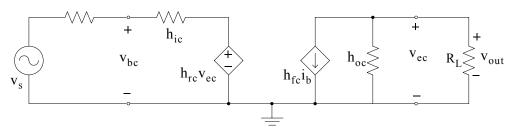
Figure 3.80. Circuit for the computation of voltage gain in a common-collector transistor amplifier
