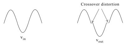
Figure 3.39. Crossover distortion in Class B amplifier
