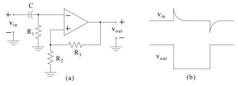
Figure 7.36. Op amp configured as a bistable multivibrator
