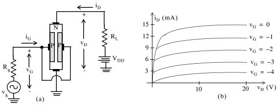
Figure 4.1. Pictorial representation and output volt-ampere characteristics for a typical JFET
