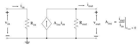
Figure 1.23. Circuit model for current amplifier where  $A_{isc}$  denotes the short circuit current gain The ideal characteristics for the circuit of Figure 1.23 are  $R_{in} \rightarrow 0$  and  $R_{out} \rightarrow \infty$ .
