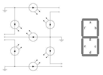
Figure 2.77. LEDs arranged for seven segment display
