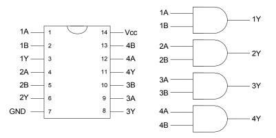
Figure 6.12. The SN7408 Quad 2-input AND gate
