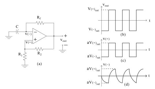
Figure 7.15. An unstable multivibrator using an op amp
