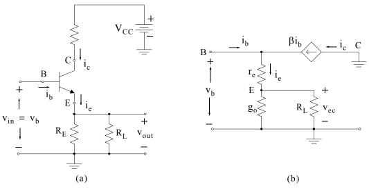
Figure 3.78. Common-collector or emitter-follower transistor circuit and its equivalent
