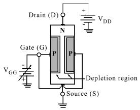
Figure 4.3. JFET operation with adjustable gate bias
