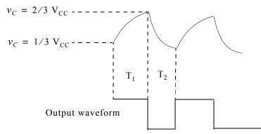
Figure 7.7. Input and output waveforms for the astable multivibrator of Figure 7.6
