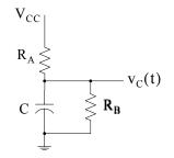
Figure 7.13. Circuit for the discharging interval
