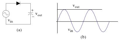
Figure 2.40. Peak rectifier circuit
