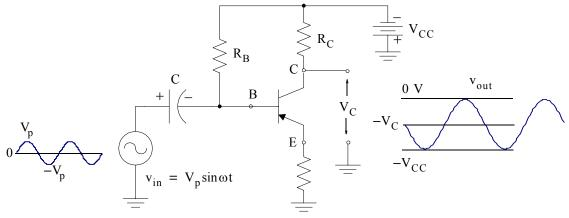
Figure 3.35. Typical Class A amplifier
