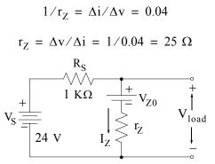
Figure 2.64. Zener diode replaced by its equivalent circuit and the load is disconnected
