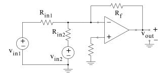
Figure 5.29. Two-input summing op amp circuit
