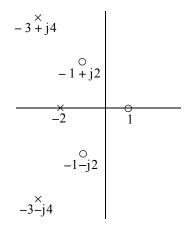
Figure 1.16. Poles and zeros of the transfer function of Example 1.3
