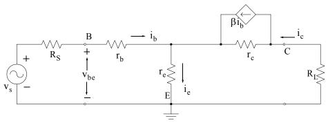
Figure 3.77. T-equivalent model for the common-emitter transistor
