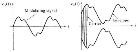
Figure 9.1. Signal and carrier wave that is amplitude-modulated by the signal.
