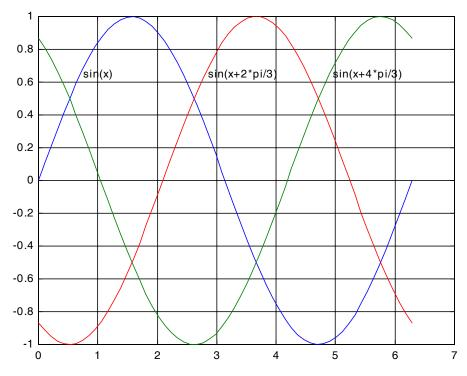
Figure A.4. Three-phase waveforms
