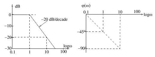
Figure 1.9. Magnitude and phase responses for the low-pass filter of Figure 1.6.
