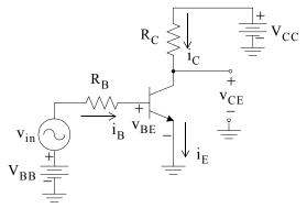
Figure 3.49. Circuit for the derivation of power relations
