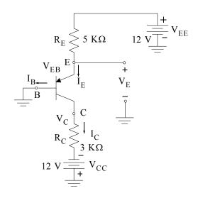
A PNP transistor will still be in the active mode if  $V_C = V_B$ . For this exercise the base is grounded so  $V_B = 0$  and we can let  $V_C = 0$  also. Then,
