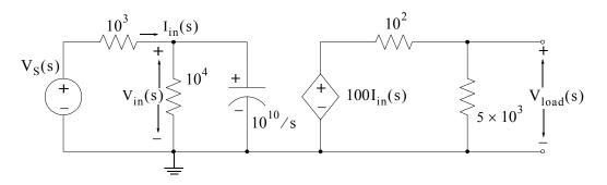
The parallel combination of the  $10^4$  resistor and  $10^{10}/s$  capacitor yields
