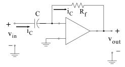
Figure 5.58. Basic differentiator circuit
