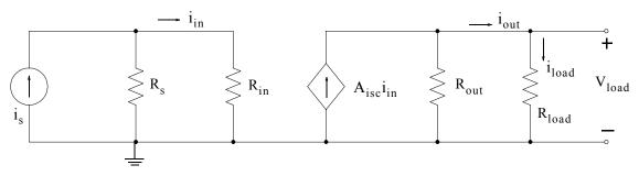
Figure 1.24. Current amplifier for Example 1.6
