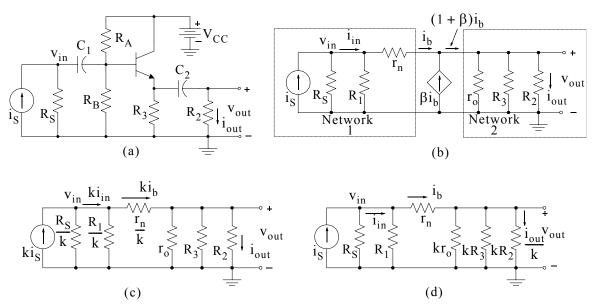
Figure C.14. Simplification of the emitter follower by application of the reduction theorem
