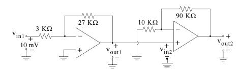
$v_{out1} = -(27/3) \times 10 = -90 \text{ mV}$
