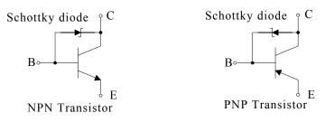
Figure 3.88. NPN and PNP transistors with Schottky diodes
