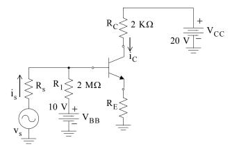
a. With  $\beta$  = 100,  $i_C$  =  $\beta i_B$  = 100 $i_B$  and for  $i_B$  = 2.5, 5.0, 7.5, and 10  $\mu A$  , we get
