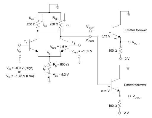
Figure 6.42. The complete ECL circuit
