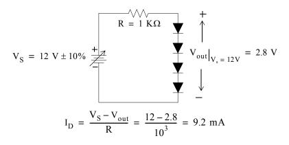
The incremental resistance  $r_D$  per diode is found from  $r_D = nV_T/I_D$  with n = 1.5. Thus, for all four diodes
