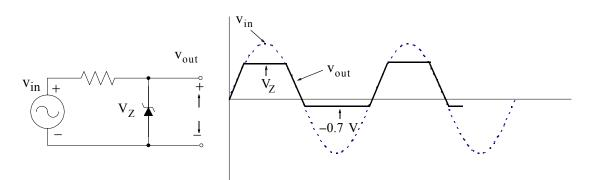
Figure 2.67. Zener limiter with one Zener diode
