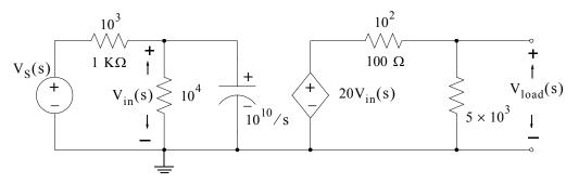
Figure 1.21. The s - domain circuit of Figure 1.20
