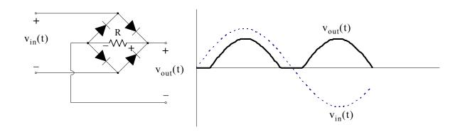
**12**. For the peak rectifier shown below, find the value of the capacitor so that the peak-to-peak ripple will be 1 volt.
