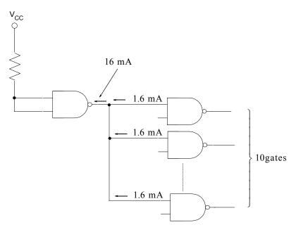
Figure 6.37. An illustration of the input current  $I_{\rm IL}$  for a 2-input NAND gate
