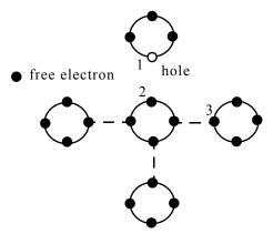
Figure 2.3. Free electron and hole movement at random
