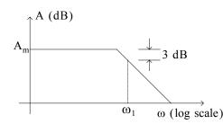
Figure 8.10. Typical logarithmic amplitude characteristics for the transistor amplifier at high frequencies Substitution of (8.23) and (8.24) into (8.28) yields
