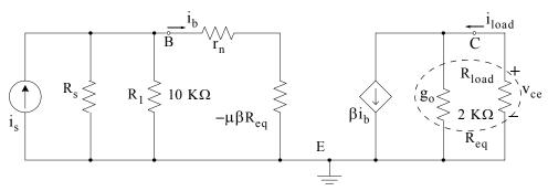
Figure 3.63. The incremental model for the transistor circuit of Figure 3.62
