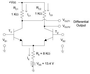
Figure 6.40. Differential circuit for Example 6.1
