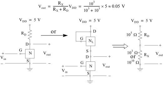
Figure 6.50. Typical NMOS inverter
