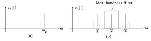
Figure 9.2. Frequency spectra of AM waves
