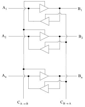
Figure 6.63. Typical bidirectional bus
