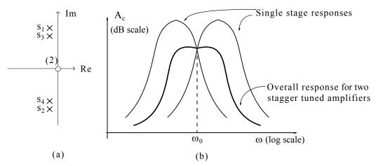
Figure 9.12. Pole-zero pattern and amplitude characteristic for two stagger-tuned amplifiers
