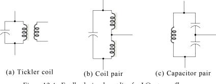
Figure 10.4. Feedback signal coupling for LC type oscillators
