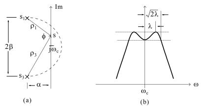
Figure 9.13. Frequency characteristic for two stagger-tuned stages
