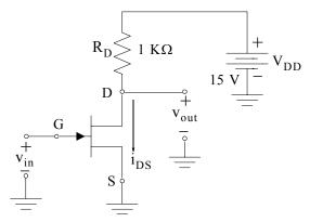
Figure 4.5. Common-source N-channel JFET amplifier for Example 4.1
