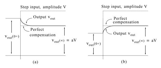
Figure B.3. Overcompensation and undercompensation responses of an attenuator to a step input
