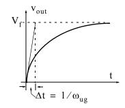
Figure 5.72. Plot for expression  $v_{out} = V_f (1 - e^{-\omega_{ug}t})$
