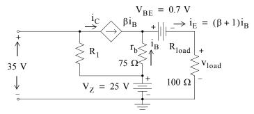
Figure 3.57. The piece-wise linear model for the transistor in Figure 3.55
