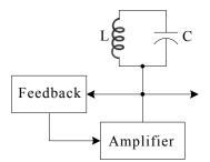
Figure 10.3. Block diagram of a typical LC oscillator
