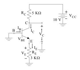
Since the base is grounded,  $V_B = 0$ , the emitter-base junction does not conduct,  $V_{BE} = 0$ ,  $I_B = 0$ ,  $I_E = 0$ , and  $V_E = 0$ . The collector current  $I_C$  is also zero because  $I_C = I_E - I_B = 0$  and thus  $V_C = V_{CC} - R_C I_C = 10V$ . Under those conditions the transistor behaves like an open switch and thus it is operating in the cutoff mode.
