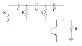
Figure 10.2. Simple form of an RC oscillator
