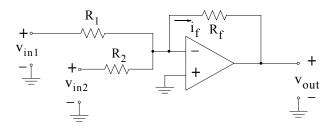
16. As stated earlier in Section 5.16, to make the overall gain of the circuit of Figure 5.67 variable, we replace resistor  $R_1$  with a fixed value resistor  $R_{fix}$  in series with a variable resistor  $R_{var}$  as shown below.
