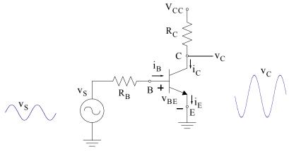
Figure 3.13. Transistor operation in the common-emitter mode
