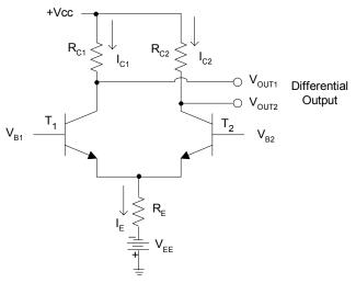
Figure 6.39. Basic differential circuit
