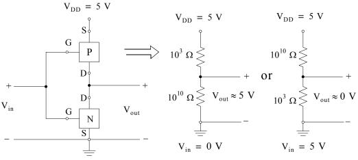
Figure 6.53. Typical CMOS inverter
