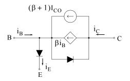
Figure 3.51. An alternative transistor model.
