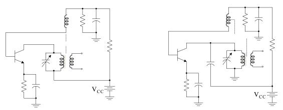
Figure 10.5. Series and shunt fed Armstrong oscillators
