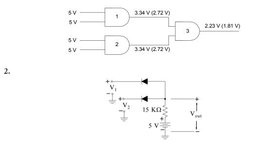
Both diodes are forward-biased for any combination of the inputs since the value of  $V_{CC}$  is greater than 3 V and can be represented as in the circuit below.
