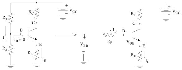
Figure 3.25. NPN transistor with fixed bias
