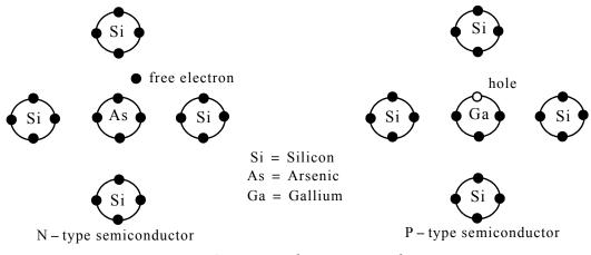
Figure 2.5. N-type and P-type semiconductors
