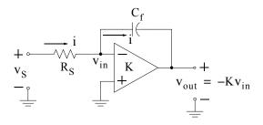
Figure C.19. Amplifier to illustrate the Miller effect
