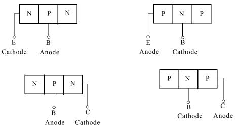
Figure 3.2. Transistors configured as diodes
