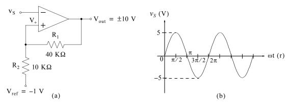
Find and sketch  $V_{+}$ upper and  $V_{+}$ lower.
