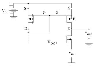
Figure 4.19. Typical CMOS common-gate amplifier
