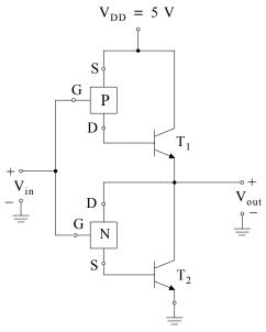
Figure 6.67. Basic BiCMOS inverter circuit.
