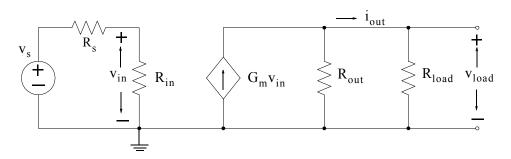
Derive an expression for the overall voltage gain  $A_v = v_{load} / v_s$
