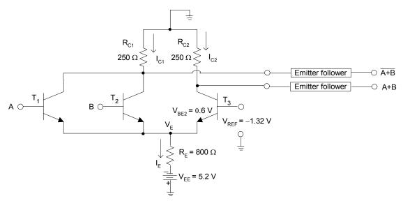
Figure 6.43. Typical 2-input ECL gate
