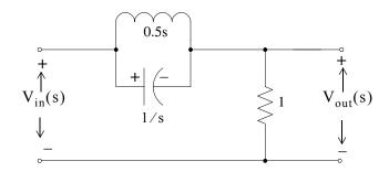
Parallel combination of the inductor and capacitor yields
