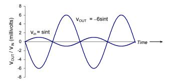
Figure 5.7. Input and output waveforms for the circuit of Example 5.2
