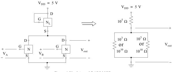
Figure 6.52. 2-input NMOS NOR gate
