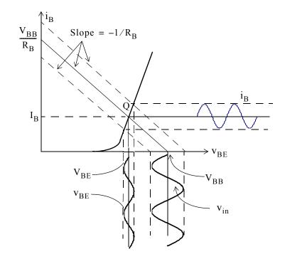
Figure 3.47. Graphical representation of  $v_{\rm BE}$  and  $i_{\rm B}$  when the input voltage  $v_{\rm in}$  is a sinusoid
