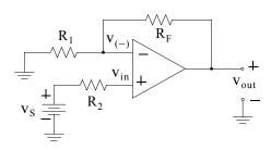
a. The feedback factor  $\beta$  is the portion of the output voltage  $v_{out}$  which appears at the inverting input, and by the voltage division expression
