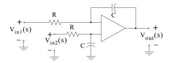
We will apply the superposition principle. With  $V_{in1}(s)$  acting alone and  $V_{in2}(s) = 0$ , the circuit reduces to that shown below.
