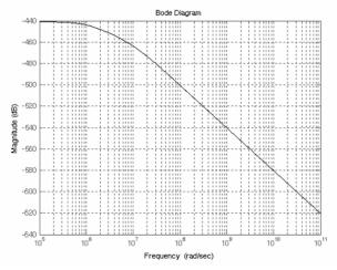
This plot shows a high attenuation of the source voltage  $v_s$  and thus the transresistance circuit model should not be used as a voltage amplifier.
