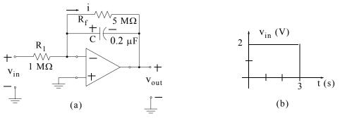
Figure 5.56. Circuit and input waveform for Example 5.18
