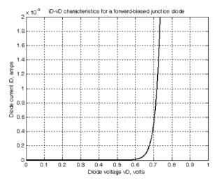
Figure 2.17. Voltage-current characteristics of the diode of Example 2.1
