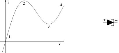
Figure 2.70. Tunnel diode characteristics and symbol
