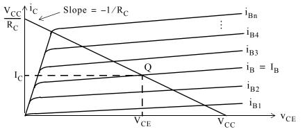
Figure 3.44. Family of curves for different values of  $i_B$
