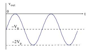
Figure 2.52. Output waveform for the voltage doubler circuit of Figure 2.51
