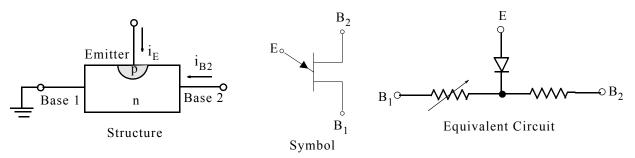
Figure 4.21. Unijunction transistor structure, symbol, and equivalent circuit
