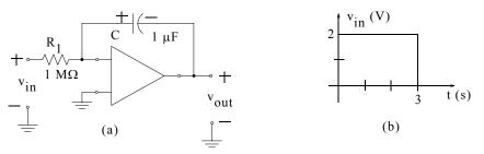
Figure 5.53. Circuit and input waveform for Example 5.17
