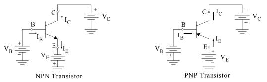
Figure 3.87. Biased bipolar transistors showing the direction of conventional current flow
