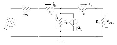
Figure 3.84. T-equivalent model for the common-collector transistor amplifier
