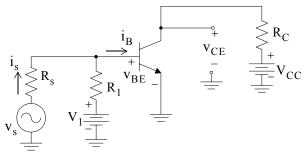
Figure 3.53. Basic transistor amplifier to be analyzed by piece-wise linear methods
