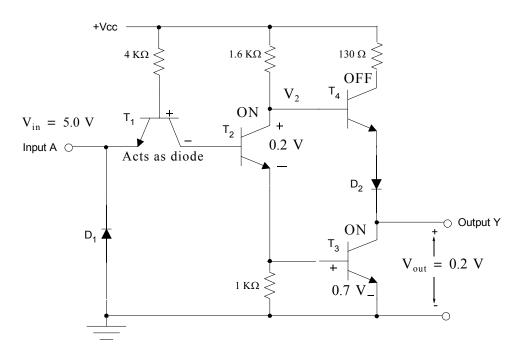
Figure 6.10. Circuit of the SN7404 Inverter for High-to-Low inversion
