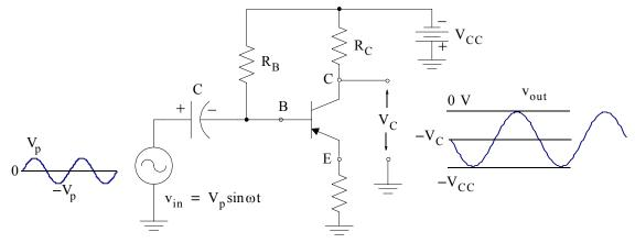
Figure 3.22. The basic PNP transistor amplifier
