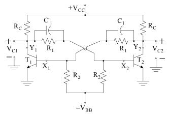
Figure 7.33. Fixed-bias flip-flop circuit including speed-up capacitors
