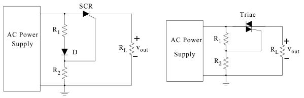
Figure 4.36. Comparison of SCR and Triac circuits
