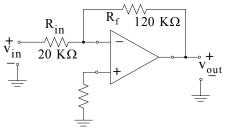
Figure 5.6. Circuit for Example 5.2
