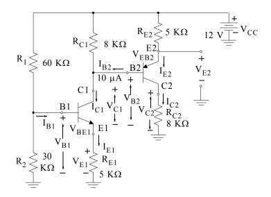
13. For the NPN transistor circuit below,  $\beta = 100$  and the output volt-ampere characteristic curves are approximately horizontal lines.
