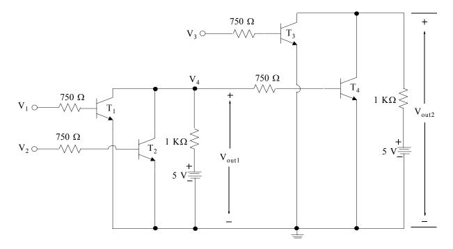
6. For the circuit of Exercise 5, derive an expression for  $V_{out1}$  High level when the driving gate has a fan-out of 2. Hint: Start with an equivalent circuit.
