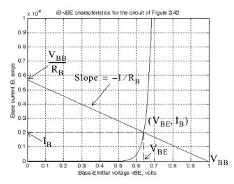
Figure 3.43. Plot showing the intersection of Equations (3.40) and (3.42)
