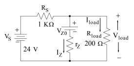
Figure 2.66. Circuit of Example 2.11 with load resistor connected and adjusted to 200  $\Omega$
