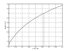
Figure 7.14. Plot for finding the ratio  $R_{\rm A}/R_{\rm B}$  to achieve 50 % duty cycle for the circuit of Figure 7.14
