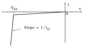
Figure 2.61. Definitions of  $V_{\rm Z0}$  and  $r_{\rm Z}$
