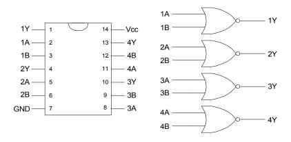
Figure 6.24. The TTL SN7402 Quad 2-input NOR gate
