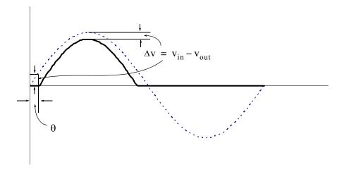
Figure 2.31. Waveforms for the derivation of conduction angle  $\theta$  for a half-wave rectifier
