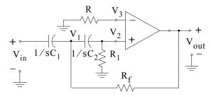
Figure 5.46. The s - domain equivalent circuit of Figure 5.49
