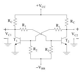
Figure 7.22. Fixed-bias flip-flop circuit
