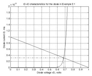
Figure 2.18. Curves for determining voltage and current in the diode of Example 2.1
