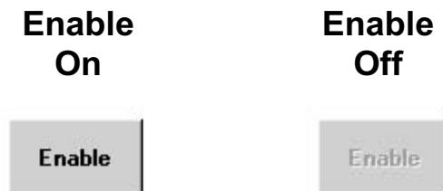
**Figure 10.11** Enable property can deactivate a control.
