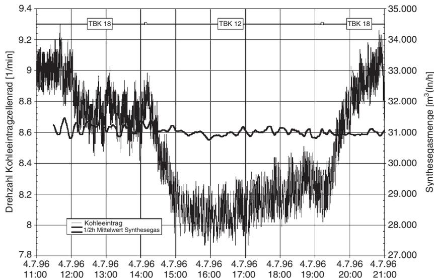
Fig. 8.9. Constant gas throughput with different coal qualities
