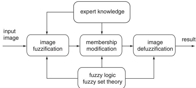
**Fig. 8.10.** General structure of fuzzy image processing
