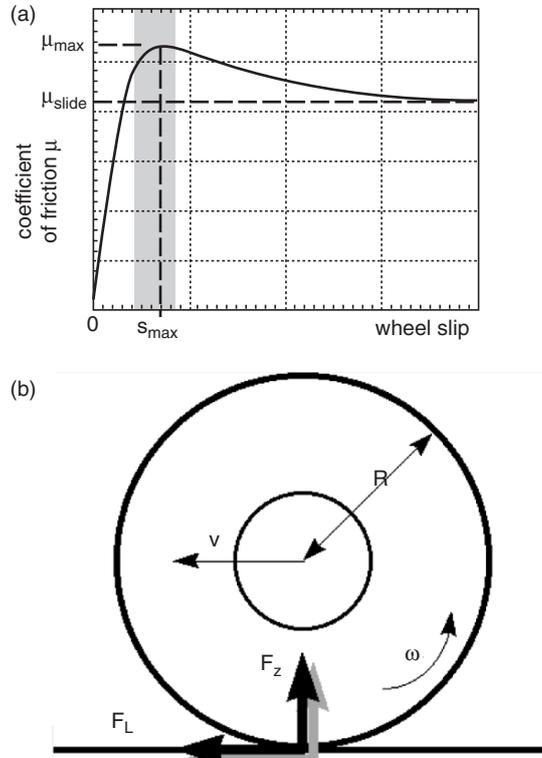
**Fig. 8.80.** (a) Friction characteristics; (b) Wheel model
