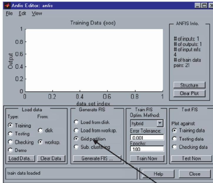
Generating initial FIS matrix using grid partition.
