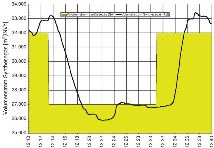
Fig. 8.7. Change of load with fuzzy control
