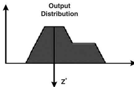
Fig. 6.4. Defuzzification using the mean of maximum
