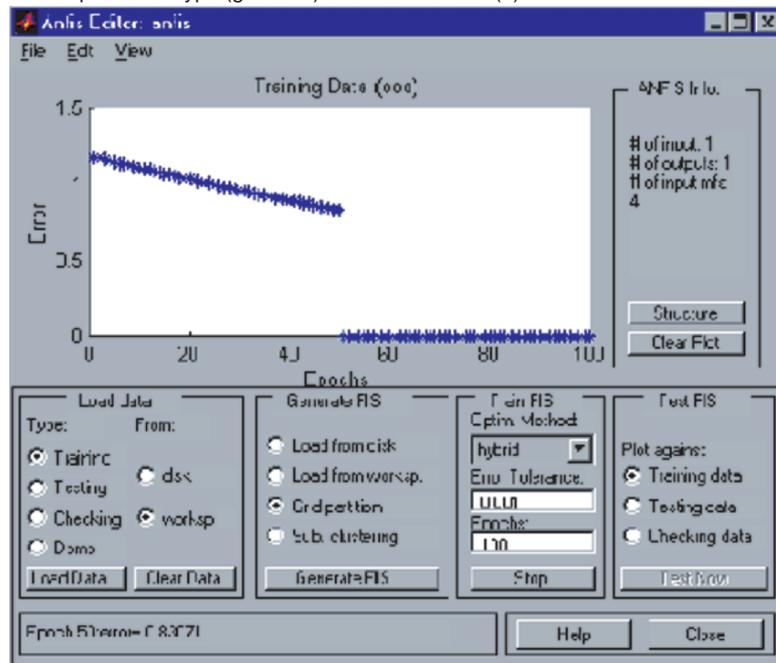
Training when error tolerance is chosen to be 0.001 and number of epochs is limited to 100.
