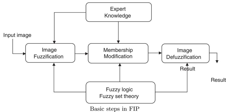
The main power of fuzzy image processing is in the middle step (modification of membership values). After the image data are transformed from gray-level plane to the membership plane (fuzzification), appropriate fuzzy techniques modify the membership values. This can be a fuzzy clustering; a fuzzy rule-based approach, a fuzzy integration approach and so on.
