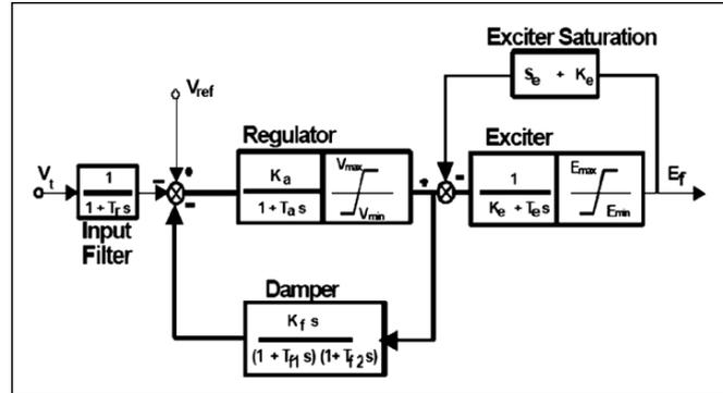
Fig. 9.28. AVR model type II of IEEE [4]: RT-IEEE2
