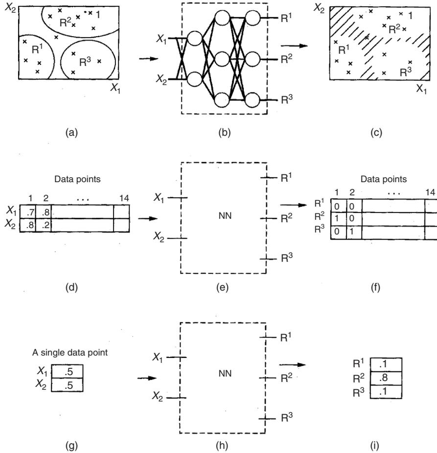
Fig. 4.11. Generation of membership functions using neural network
