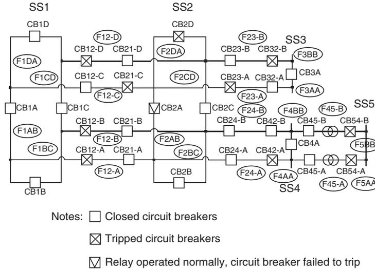
Fig. 8.119. Operating relays and tripped circuit breakers
