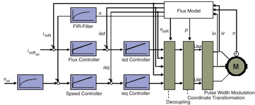
Fig. 8.29. Field-oriented control of AC induction motors
