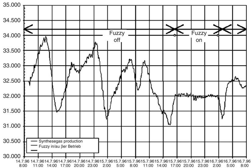
Fig. 8.6. Throughput control with and without fuzzy control
