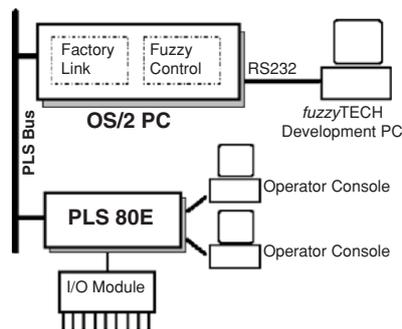
Fig. 8.4. Integration of fuzzy logic into DCS
