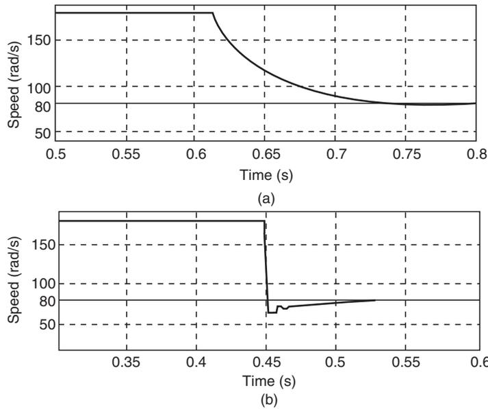
**Fig. 9.6.** Speed change from 180 to 80 rad s<sup>-1</sup>: (a) without feeding and (b) feeding the phase with decreasing inductance
