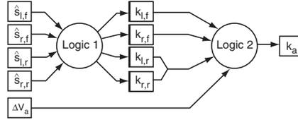
Fig. 8.83. Structure of the fuzzy estimator
