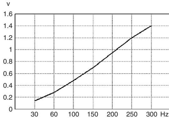
Fig. 9.47. The frequency response of F/V converter
