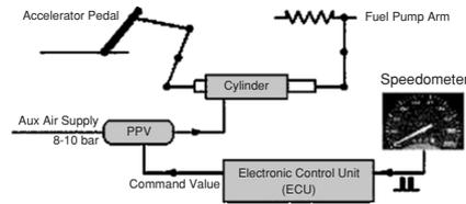
**Fig. 8.35.** Mechanical design of the speed limiter
