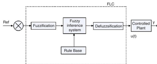
Fig. 8.130. Block diagram of fuzzy logic controller
