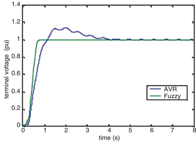
**Fig. 9.32.** One machine analysis (terminal voltage  $V_t$ )
