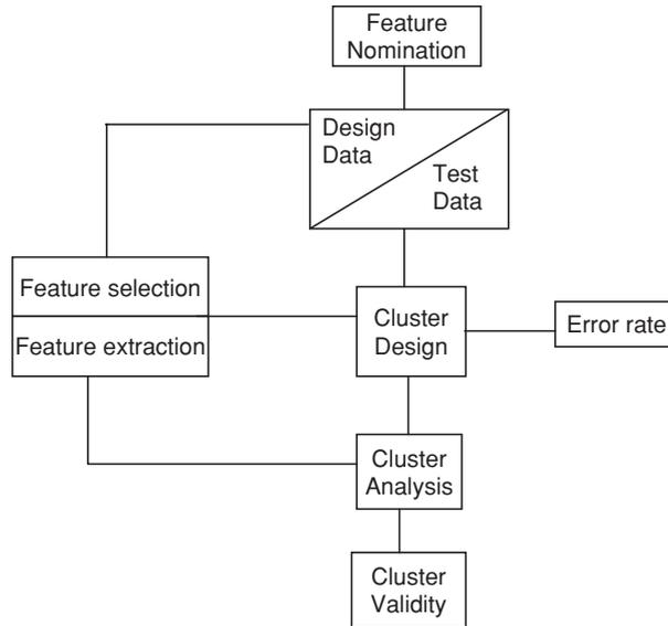
**Fig. 8.135.** Block diagram of fuzzy pattern recognition
