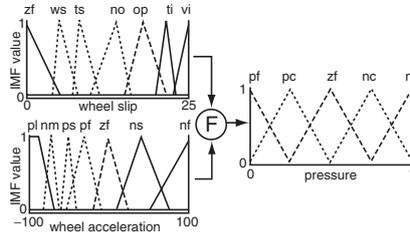
Fig. 8.87. Structure of the fuzzy ABS controller
