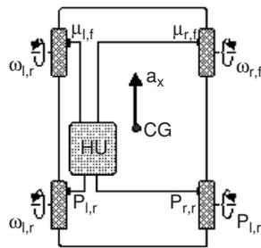
**Fig. 8.81.** Sensors and actuators of the experimental car
