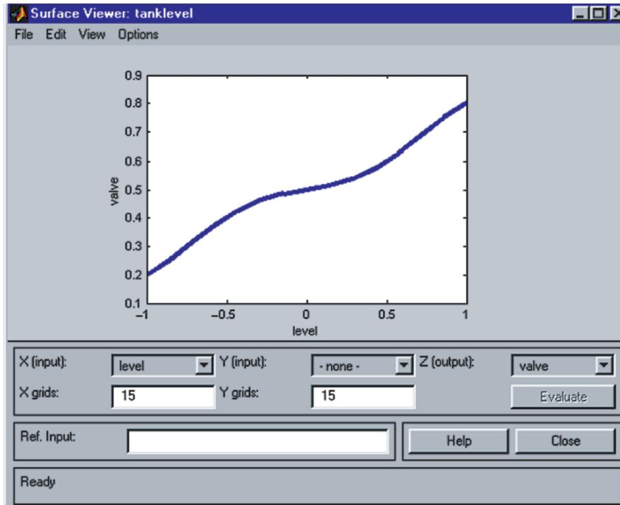
*Step 7:* Save the file to the workspace as `tanklevel` and go to the command window and enter the command `tanklevel`.
