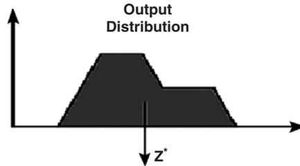
Fig. 6.3. Defuzzification using the center of mass
