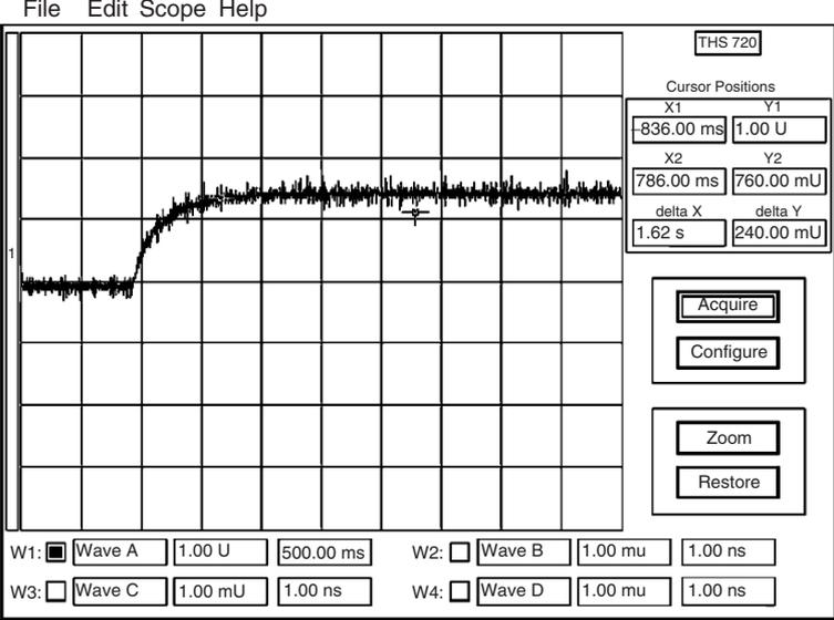
Fig. 9.48. The unit step response to no load
