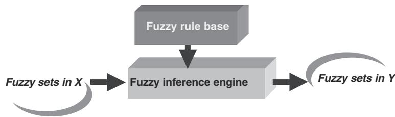
**Fig. 1.4.** Configuration of a pure fuzzy system
