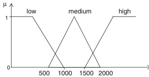
**Fig. 4.6.** Membership for fuzzy variable “speed” in rpm
