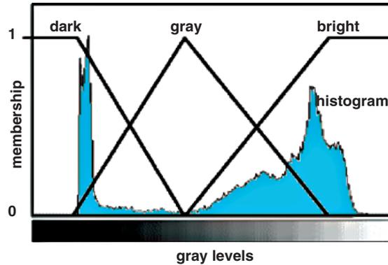
Fig. 8.14. Histogram fuzzification with three membership functions
