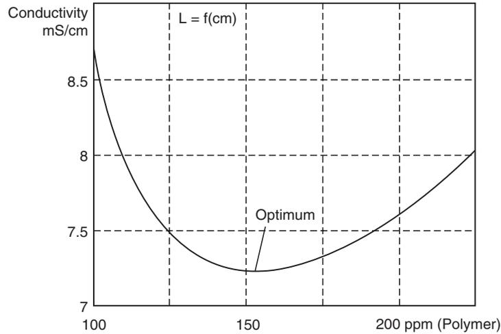
**Fig. 8.54.** Thick slurry conductivity over polymer proportion
