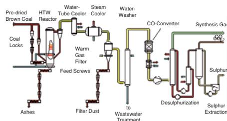
Fig. 8.2. Process diagram of HTW plant
