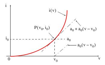
Figure 6.35. Second approximation of i(v)
