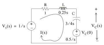
Figure B.2. Transformed Circuit for Example B.1
