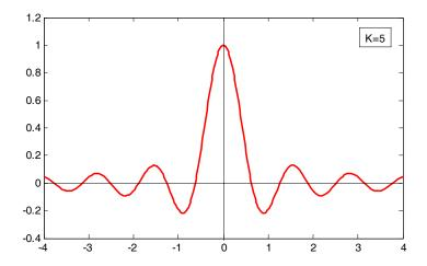
Figure 6.27. Line spectrum of (6.109) for k = 5
