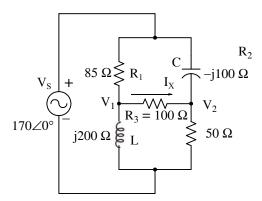
Figure 4.3. Circuit for Example 4.18
