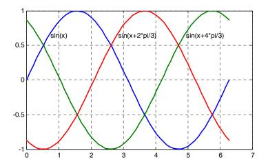
Figure 1.4. Three-phase waveforms
