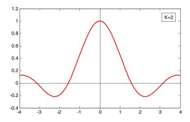
Figure 6.26. Line spectrum of (6.109) for k=2
