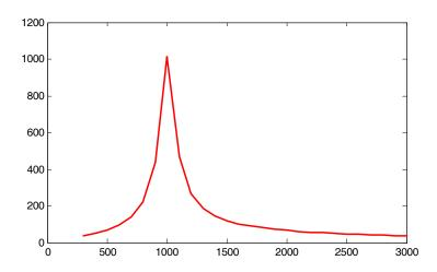
Figure 1.2. Plot of impedance |z| versus frequency  $\omega$  for Example 1.10
