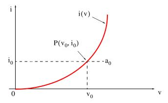
Figure 6.34. First approximation of i(v)
