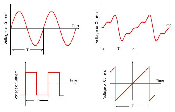
Figure 3.1. Examples of alternating voltages and currents
