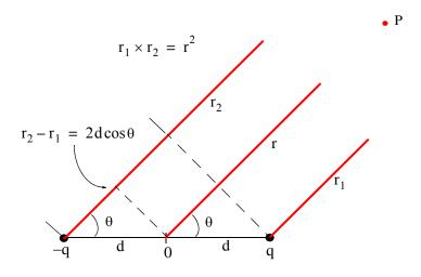
Figure 15.4. Derivation of the voltage developed by a dipole
