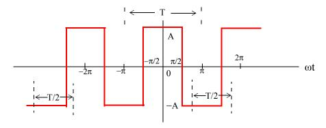
Figure 6.10. Square waveform with ordinate shifted by  $\pi/2$
