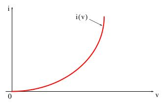
Figure 6.32. Current-voltage (i-v) characteristics for a typical semiconductor diode
