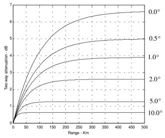
Figure 8.15. Attenuation versus range; frequency is 10 GHz.
