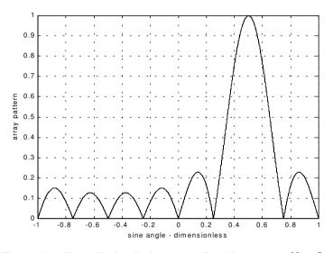
Figure 10.6a. Normalized radiation pattern for a linear array.  ${\it N}=8$  ,  $d=\lambda/2$  , and  $\beta_0=30^\circ$  .
