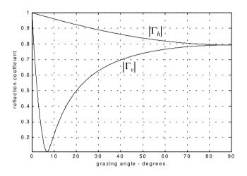
Figure 8.6. Reflection coefficient magnitude.
