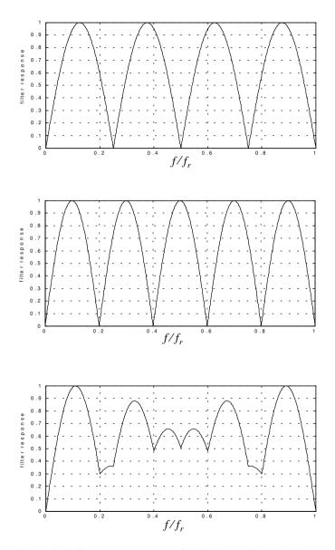
Figure 9.16. Frequency responses of a single canceler. Top plot corresponds to  $T_1$ , middle plot corresponds to  $T_2$ , bottom plot corresponds to stagger ratio  $T_1/T_2 = 4/3$ . This plot can be reproduced using MATLAB program "fig9\_16.m" given in Listing 9.4 in Section 9.14.
