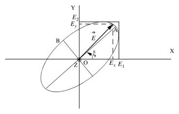
Figure 2.7. Polarization ellipse in the general case.
