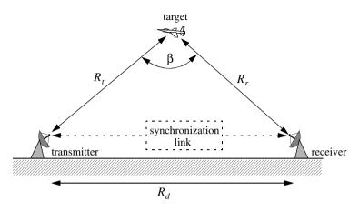
Figure 1.30. Bistatic radar geometry.
