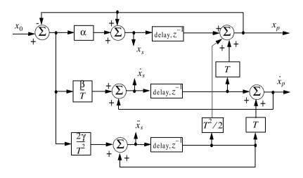
Figure 11.21. An implementation for an  $\alpha\beta\gamma$  tracker.
