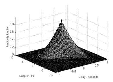
Figure 6.5c. Up-chirp LFM 3-D ambiguity plot. Pulse width is 1 second; and bandwidth is 10 Hz.
