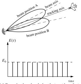
Figure 11.4. Error signal produced when the target is on the tracking axis for conical scan.
