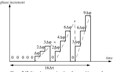
Figure 7.17. Stepwise approximation of an up-chirp waveform, using a Frank code of 16 elements.
