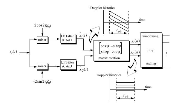
Figure 12.13. Signal processing block diagram for the *kth* range bin.
