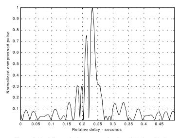
Figure 7.10c. Mismatched compressed pulse; 10% time dilation.
