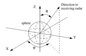
Figure 2.8. Direction of antenna receiving backscattered waves.
