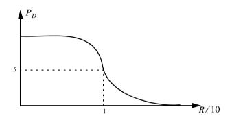
The cumulative probability of detection is given in Eq. (4.95), where the probability of detection of the first frame is selected to be very small. Thus, we can arbitrarily choose frame 1 to be at R = 16Km. Note that selecting a different starting point for frame 1 would have a negligible effect on the cumulative probability (we only need  $P_{D_1}$  to be very small). Below is a range listing for frames 1 through 9, where frame 9 corresponds to R = 8Km.
