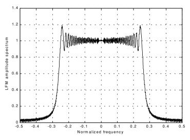
Figure 5.8. Typical spectrum for an LFM waveform.
