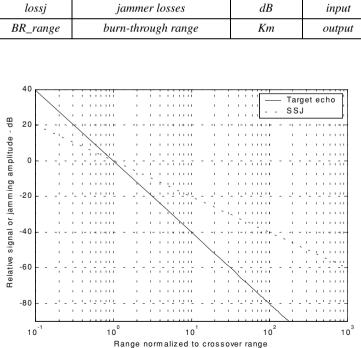
Figure 1.25. Target and jammer echo signals. Plots were generated using the program "*ssj\_req.m*".
