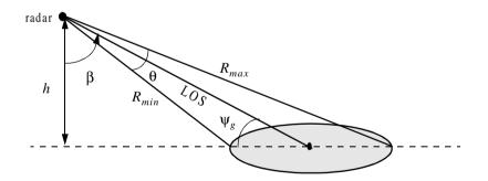
Figure 12.4. Definition of minimum and maximum range.
