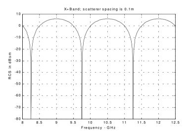
Figure 2.4. Illustration of RCS dependency on frequency.
