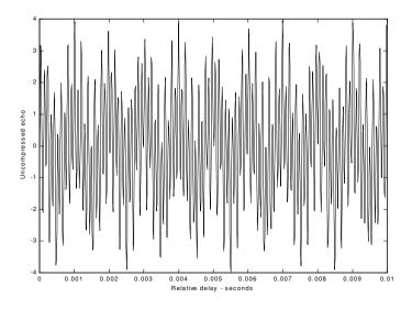
Figure 7.8. Uncompressed echo signal. Three targets are unresolved.
