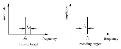
Figure 1.14. Spectra of radar received signal.
