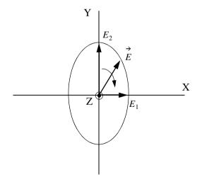
Figure 2.6. Electric field components along the x and y directions. The positive z direction is out of the page.
