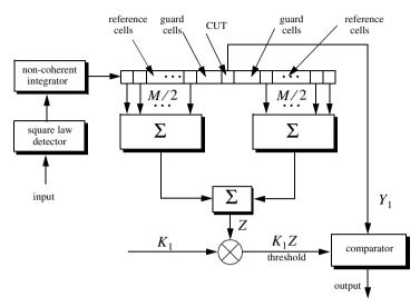
Figure 4.18. Conventional CA-CFAR with non-coherent integration.
