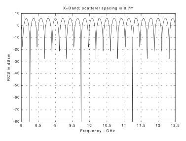
Figure 2.5. Illustration of RCS dependency on frequency.
