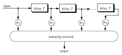
Figure 9.19. N-stage tapped delay line filter.
