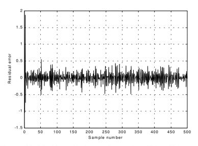
Figure 11.25a-2. Position residual (error). Large gain coefficients. Noise present. The error settles down quickly. The variation is due to noise.
