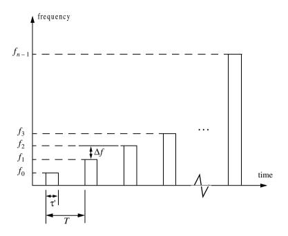
Figure 5.9. Stepped frequency waveform burst.
