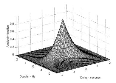
Figure 6.2c. Single pulse 3-D ambiguity plot. Pulse width is 2 seconds.
