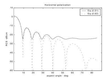
Figure 2.20b. Backscattered RCS for a rectangular flat plate.
