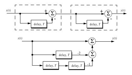
Figure 9.12. Two configurations for a double delay line canceler.
