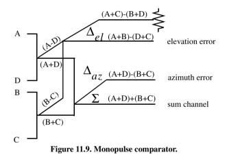
To generate the elevation difference beam, one can use the beam difference (A-D) or (B-C). However, by first forming the sum patterns (A+B) and (D+C) and then computing the difference (A+B)-(D+C), we achieve a stronger elevation difference signal,  $\Delta_{el}$ . Similarly, by first forming the sum patterns (A+D) and (B+C) and then computing the difference (A+D)-(B+C), a stronger azimuth difference signal,  $\Delta_{az}$ , is produced.
