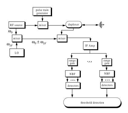
Figure 3.7. Pulsed radar block diagram.
