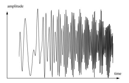
Figure 7.2a. Composite echo signal for two unresolved targets.
