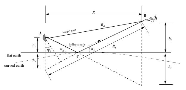
Figure 8.9. Geometry for multipath propagation.
