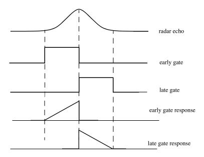
Figure 11.16. Illustration of split-range gate.
