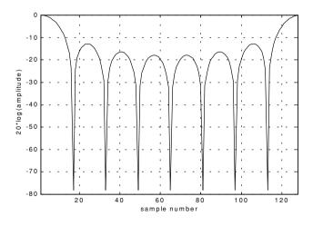
Figure 13.2. Normalized amplitude spectrum for rectangular window.
