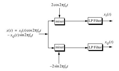
Figure 5.1. Extraction of quadrature components.
