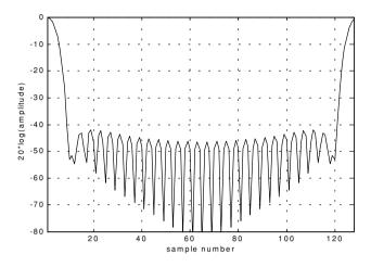
Figure 13.3. Normalized amplitude spectrum for Hamming window.
