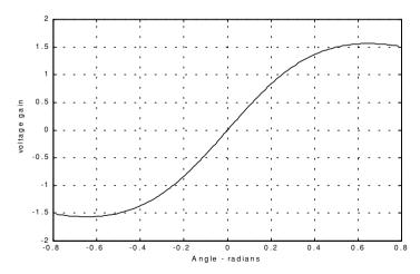
Figure 11.13b. Difference-to-sum ratio corresponding to Fig. 11.12a.
