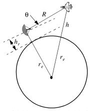
Figure 8.4. Measuring target height for 4/3 earth.
