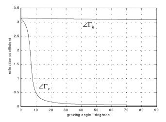
Figure 8.7. Reflection coefficient phase.
