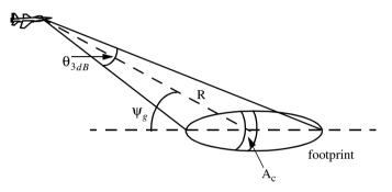
Figure 9.4. Airborne radar in the look-down mode.
