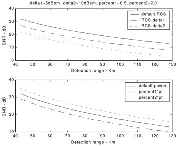
Figure 1.18. Typical outputs generated by the function *"radar\_eq.m"*. Plots correspond to parameters from Example 1.4.
