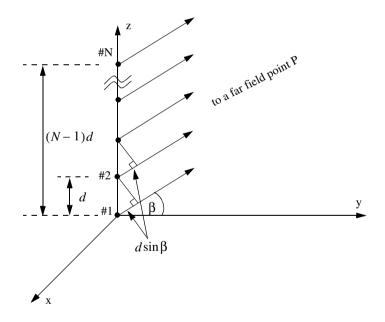
Figure 10.4. Linear array of equally spaced elements.
