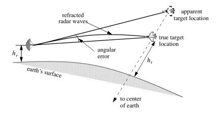
Figure 8.2. Refraction high altitude effect on electromagnetic waves.
