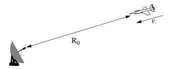
Figure 1.13. Closing target with velocity v.
