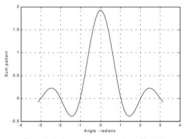
Figure 11.11b. Sum pattern corresponding to Fig. 11.11a.
