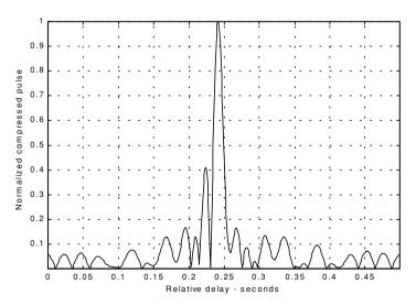
Figure 7.10b. Mismatched compressed pulse; 5% Doppler shift.
