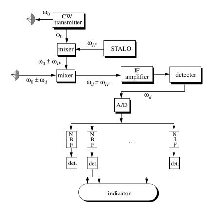
Figure 3.1. CW radar block diagram.
