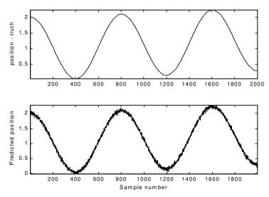
Figure 11.30a. True and predicted positions. Aggressive maneuvering. Plot produced using the function *"kalman\_filter.m"*.
