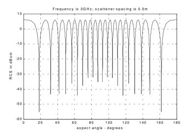
Figure 2.2. Illustration of RCS dependency on aspect angle.
