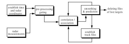
Figure. 11.17. Simplified block diagram of TWS data processing.
