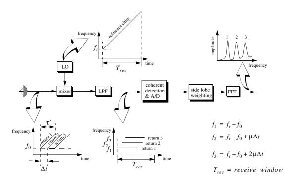
Figure 7.7. Stretch processing block diagram.
