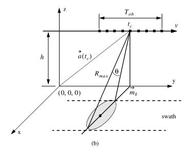
Figure 12.3. Side looking SAR geometry.
