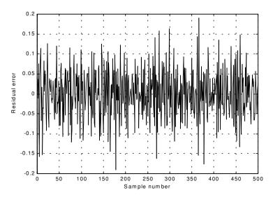
Figure 11.27b. Position residual (error). Small gain coefficients. Noise present. The error stays fairly large; however, its average is around zero. The variation is due to noise.
