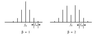
Figure 3.4. Amplitude line spectra sketch for FM signal.
