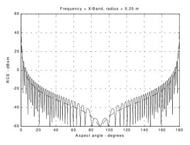
Figure 2.13. Backscattered RCS for a circular flat plate. Solid line corresponds to Eq. (2.37). Dashed line corresponds to Eq. (2.36).
