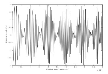
Figure 7.5. Uncompressed echo signal. Scatterers are unresolved.
