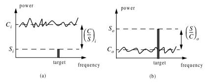
Figure 9.18. Illustration of SCV. (a) MTI input. (b) MTI output.
