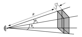
Figure 9.6. Definition of a resolution volume.
