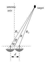
Figure 11.14. Single coordinate phase comparison monopulse antenna.
