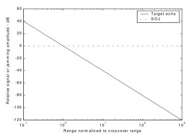
Figure 1.26. Target and jammer echo signals. Plots were generated using the program "soj\_req.m".
