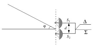
Figure 11.15. Single coordinate phase monopulse antenna, with sum and difference channels.
