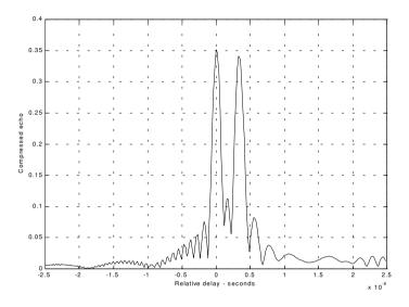
Figure 7.6. Compressed echo signal. Scatterers are resolved.
