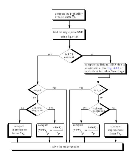
Figure 4.16. Solving the radar equation.
