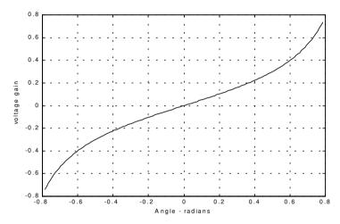
Figure 11.13a. Difference-to-sum ratio corresponding to Fig. 11.11a.
