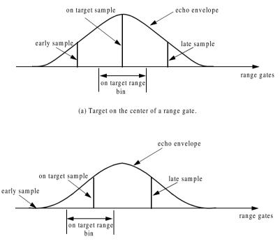
(b) Target on the boundary between two range gates.
