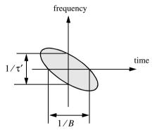
Figure 6.14. Ambiguity contour plot associated with an up-chirp LFM waveform. For an exact plot see Fig. 6.5b.
