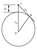
Figure 8.5. Measuring the distance to the horizon.
