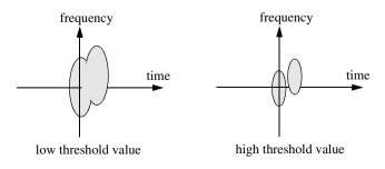
Figure 6.10. Effect of threshold value on resolution.
