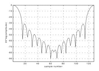
Figure 13.4. Normalized amplitude spectrum for Hanning window.
