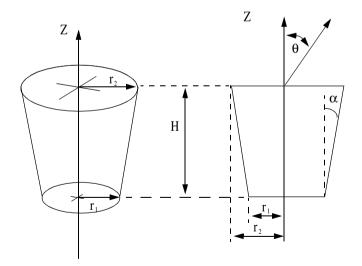
Figure 2.15. Definition of half cone angle.
