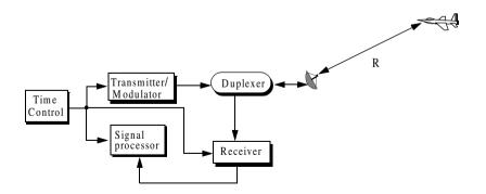
Figure 1.5. A simplified pulsed radar block diagram.
