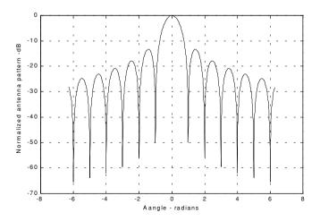
Figure 1.31. Normalized (sin x / x) antenna pattern.
