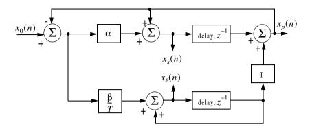
Figure 11.20. An implementation for an  $\alpha\beta$  tracker.
