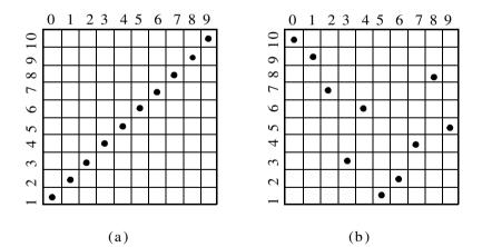
Figure 7.12. Frequency assignment for a burst of N subpulses. (a) SFW (stepped LFM); (b) Costas code of length Nc = 10.
