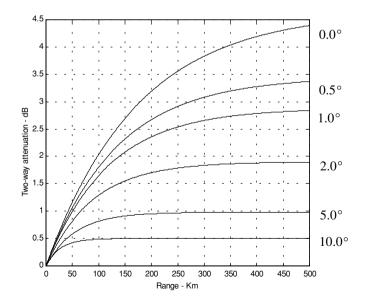
Figure 8.14. Attenuation versus range; frequency is 3 GHz.
