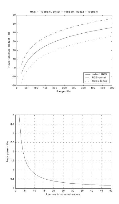
Figure 1.24. Typical outputs generated by the function *"power\_aperture\_req.m"*. Plots correspond to parameters from Example 1.6.
