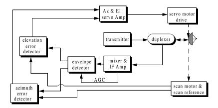
Figure 11.3. Simplified conical scan radar system.
