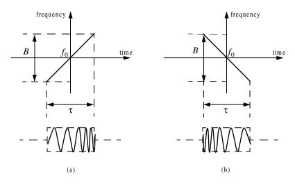
Figure 5.6. Typical LFM waveforms. (a) up-chirp; (b) down-chirp.
