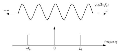
Figure 5.2. Amplitude spectrum for a continuous sine wave.
