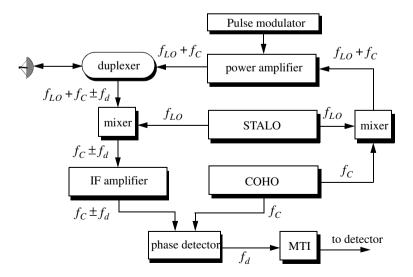
Figure 9.9. Coherent MTI radar block diagram.
