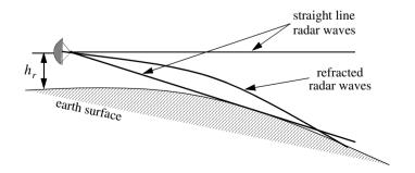
Figure 8.3. Refraction low altitude effect on electromagnetic waves.
