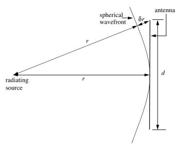
Figure 10.1. Construction for far field criterion.
