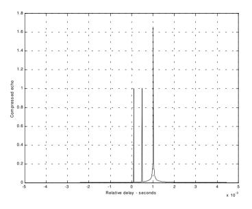
Figure 7.9. Compressed echo signal. Three targets are resolved.
