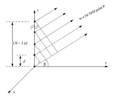
Figure 12.1. Geometry of real or synthetic array.
