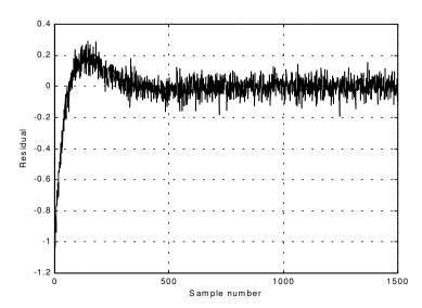
Figure 11.25b-2. Position residual (error). Small gain coefficients. Noise present. The error requires more time before settling down. The variation is due to noise.
