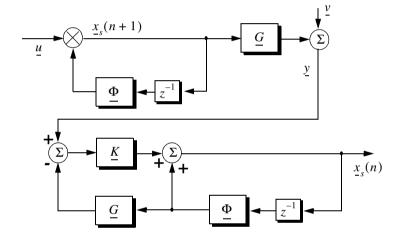
Figure 11.28. Structure of the Kalman filter.
