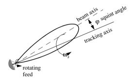
Figure 11.2. Conical scan beam.
