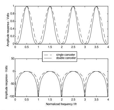
Figure 9.13. Normalized frequency responses for single and double cancelers.
