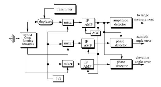
Figure 11.10. Simplified amplitude comparison monopulse radar block diagram.
