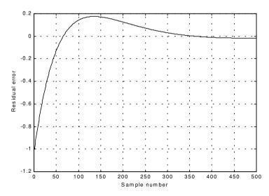
Figure 11.24b-2. Position residual (error). Small gain coefficients. No noise. It takes the filter longer time for the error to settle down.
