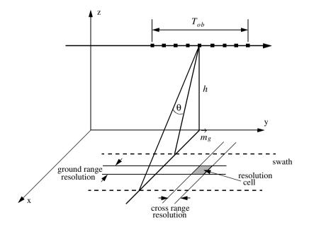
Figure 12.6. Definition of a resolution cell.
