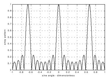
Figure 10.7a. Normalized radiation pattern for a linear array.  ${\it N}=8$  ,  $d=1.5\lambda$  , and  $\beta_0=0^\circ$  .
