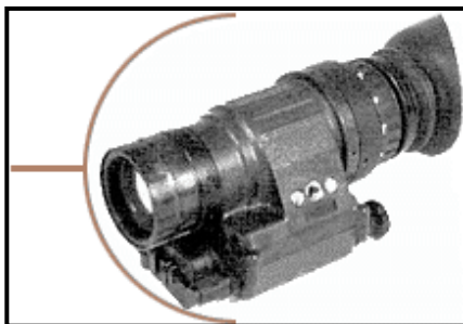
Figure B-4. AN/PVS-14 monocular night vision device.
