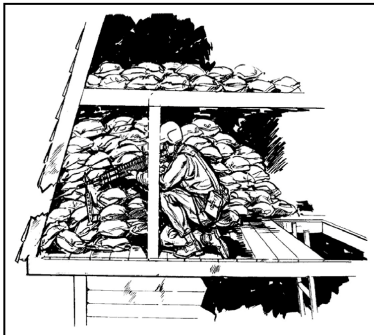
Figure 3-60. Firing platform built under roof.
