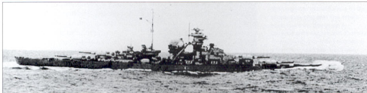
One of the last photographs taken of Bismarck . Shot from Prinz Eugen , she can be seen to be down by the bows having shipped a considerable amount of water through the hole caused by a direct hit from Prince of Wales .
