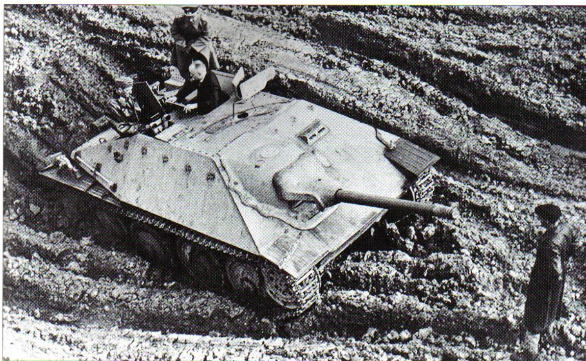
Overhead view of Sturmgeschütz 38(t) Fgst.Nr.321003 under test. The remote-controlled machine gun has longer sides on the armour shield (similar to those used on the Sturmgeschütz Ausf. G). Note the periscope mounted behind the SF 14Z scissors periscope. The machine pistol port to the right of the driver's visor is just visible. (BMM)
