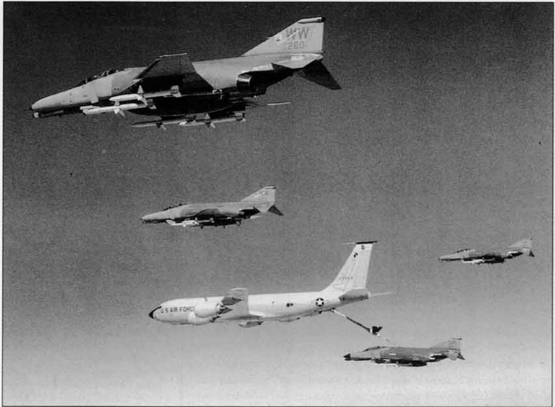
One of four HARM-carrying F-4G 'Wild Weasel' aircraft is seen taking on fuel from a Boeing KC-135R Stratotanker, one of the two primary types of tanker aircraft operated by the US Air Force for the support of strategic as well as tactical aircraft in the air campaign against Iraq (DoD via Robert F Dorri)
