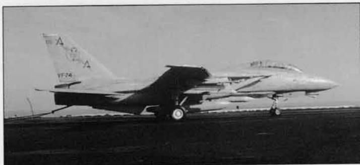
Brought to a rapid halt after catching the arrester wire, this Grumman F-14A (Plus) Tomcat is identified by its markings as a machine of the VF-74 of the USS Saratoga's CVW-17 wing
