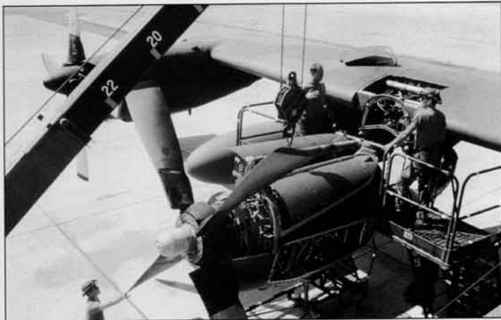
Ground crew prepare to change the Allison T56 turboprop engine in the starboard inner position of a Lockheed C-130 Hercules, the workhorse for the tactical airlift role in Operations 'Desert Shield' and 'Desert Storm'
