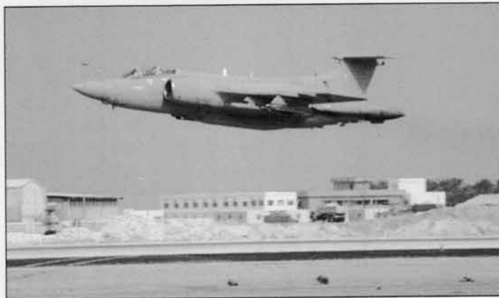
The BAe Buccaneer S 2B aircraft provided by Nos 12 and 208 Squadrons as well as No 237 Operational Conversion Unit were initially deployed to use their AVQ-23E 'Pave Spike' laser designating pods to 'illuminate' targets for the laser-guided bombs dropped by Tornado GR 1 aircraft, but from 21 February themselves dropped 48 such bombs ( Crown Copyright (RAF) via MARS )
