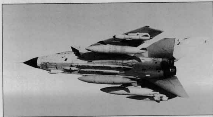
The Tornado F 3 air-superiority fighter's counterparts were the Tornado GR 1 long-range interdictor and, as seen here, the Tornado GR 1A reconnaissance type. Provided by No 2 Squadron at Laarbruch in Germany, the latter has a horizon-to-horizon IR system in place of the interdictor's two 27 mm cannon, and in addition to two drop tanks carries under the outboard wing pylons a Marconi Sky Shadow ECM pod and a BOZ-107 chaff/flare dispenser pod respectively (DPR (RAF), Crown Copyright)
