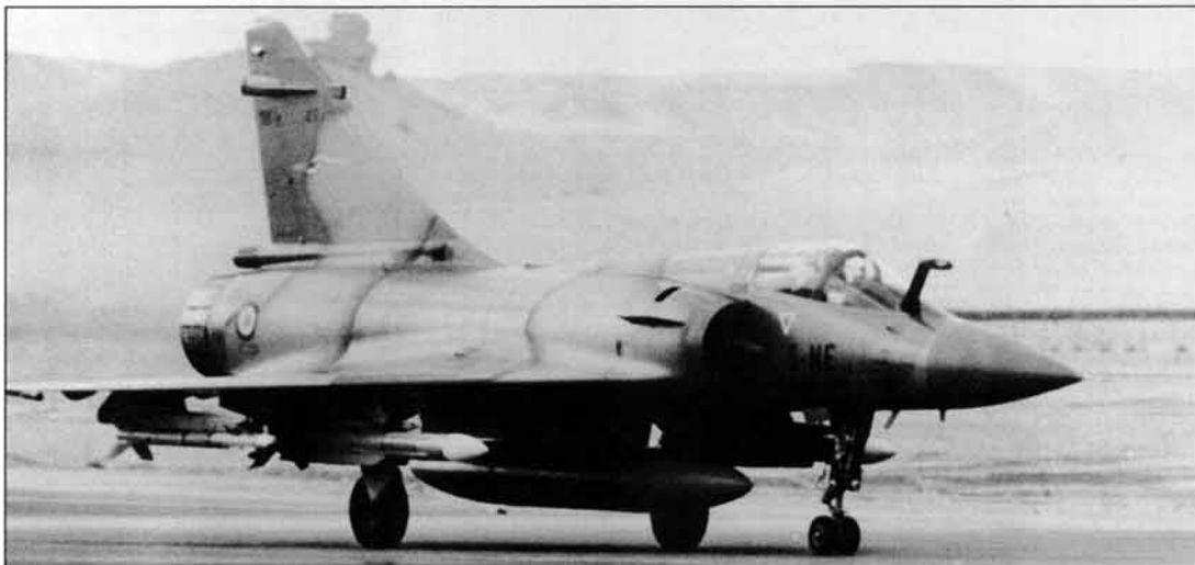
Carrying two examples each of the Super 530 medium- and Magic short-range AAMs under its wing, this aircraft preparing to take-off on a combat air patrol is a Dassault Mirage 2000C of the French air force's EC 5 unit
