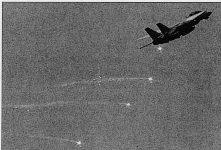
A Grumman F-14A Tomcat fighter of the US Navy fires a spread of flares at it climbs over Iraqi territory, the flares being designed to decoy IR-guided missiles that would otherwise home on the fighter's hot exhausts
