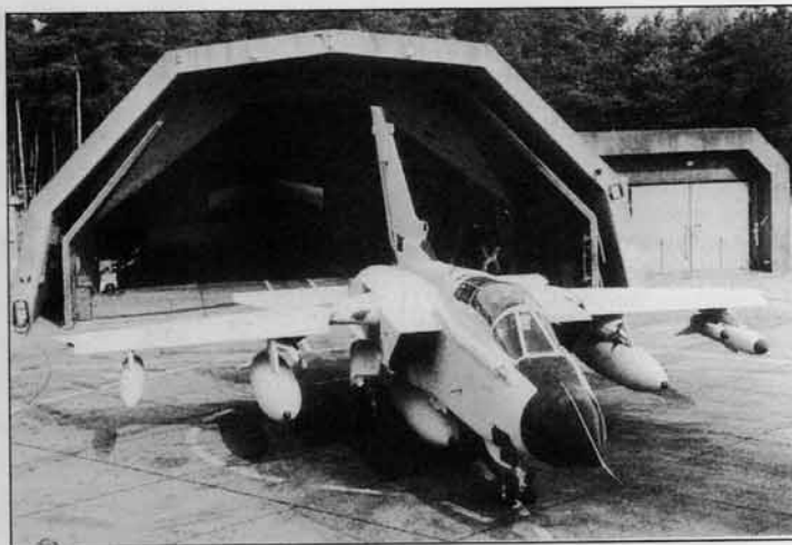
Carrying the Marconi Sky Shadow jammer and BOZ-107 chaff/flare dispenser pods under the outboard wing pylons, this Panavia Tornado GR 1 of No 14 Squadron is leaving its hardened aircraft shelter at RAF Brüggen, Germany, for the flight to Bahrain/Muharraq, where it became part of No 15 (Composite) Squadron (PRM)
