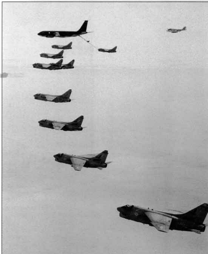
With a single Grumman A-6E Intruder in the background, eight Vought A-7E Corsair II attack aircraft wait to take on fuel from a Boeing KC-135 once the ninth aeroplane has topped off its tanks
