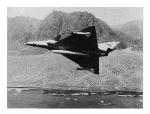
The Kfir C-2, an Israeli redesign of the Dassault Mirage V, is the result of Israel's desire to become self-sufficient in jet fighters. Powered by the 'embargo-proof American General Electric J79 turbojet engine, and with many refinements which improve its range, performance and capabilities over those of the original French design, it is a potent fighter-bomber and 'dog-fighter'. In 1982 the Kfir carried the main burden of close air support missions. (IAI)
