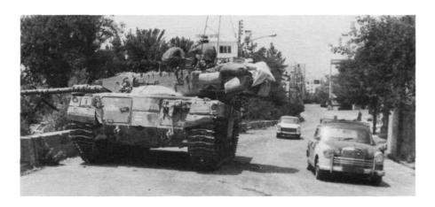
Merkava in the hills near Aley; the tank is seen here from the rear, with its gun traversed to 'nine o'clock'. Note the large hatches in the rear hull, which allow both rapid loading with palletised ammunition, and also access for the crew, for casualty evacuation cases, or for any other soldier who needs a well-protected ride in the front line of battle. (Author's photo)
