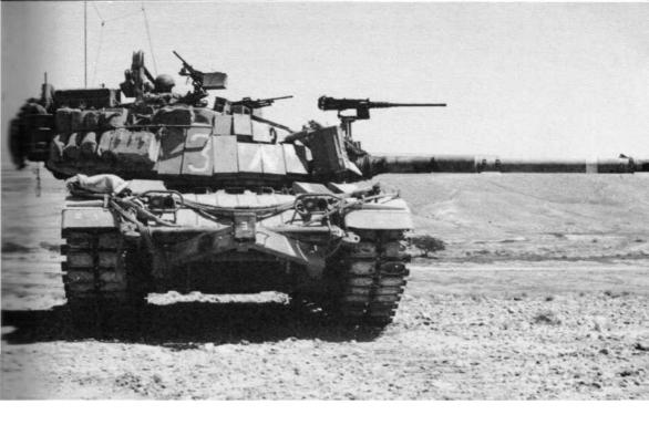
One transitional response to the threat of anti-tank weapons such as the man-portable 'Sagger', which did such execution in 1973, is the 'Blazer' reactive armour system of externally-mounted explosive blocks, as fitted to this IDF M60 tank. A drawback to reactive armour systems is the threat they pose to exposed turret crew members and nearby friendly infantry. (Christopher Foss)
