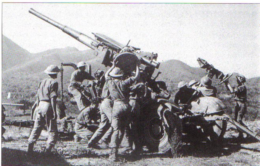
Italy, 1943: bringing a 3.7in anti-aircraft gun into action. The heavy 3.7 proved a versatile weapon on its mobile mounting; like the German 8.8cm Flak, it was also capable of use against ground targets, firing up to 25 rounds a minute out to a range of 20,600 yards.
