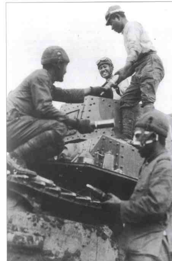
Crewmen of a Type 89B medium tank of the 13th Tank Regiment in China pass ammunition for the 57mm main gun up to the turret hatch. Three of them wear the light summer version of the crash helmet, and the men on the turret have goggles. The man at right foreground appears to have a bandaged face wound. (US National Archives)
