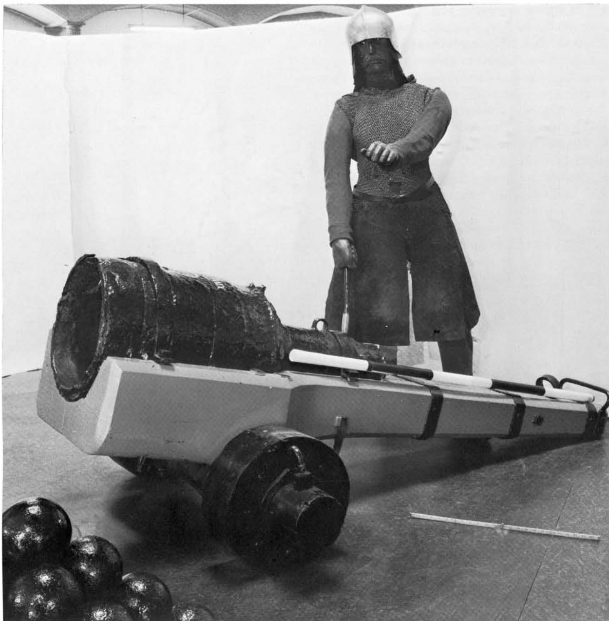
Early fifteenth century bombard of wrought iron with 15-in. calibre, firing a stone shot weighing about 160 pounds. The carriage is modern
