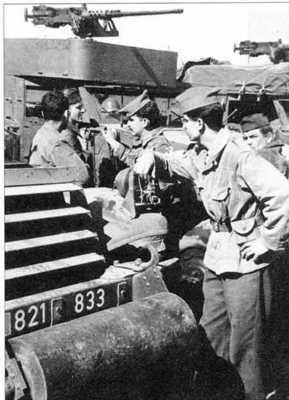
French motorised and mechanised units – here the 2e RZ, 1957 – used many types of US vehicles supplied since 1943. This M3 half-track served in large numbers, as did the M8 armoured car, Dodge Weapons Carrier and 6x6 patrol vehicles, and GMC 2½ ton trucks. (Courtesy Jean-Luc Delauve)
