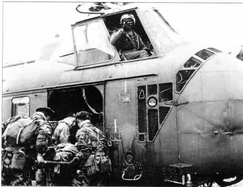
A 2e REP casualty is evacuated in a Sikorsky S-55 (H-19). By 1958 some 40 of the similar but larger S-58 (H-34), with space for 12 infantry, were already available for tactical transport and escort – gunship versions were fitted with dual 12.7mm MGs and a 20mm cannon.
