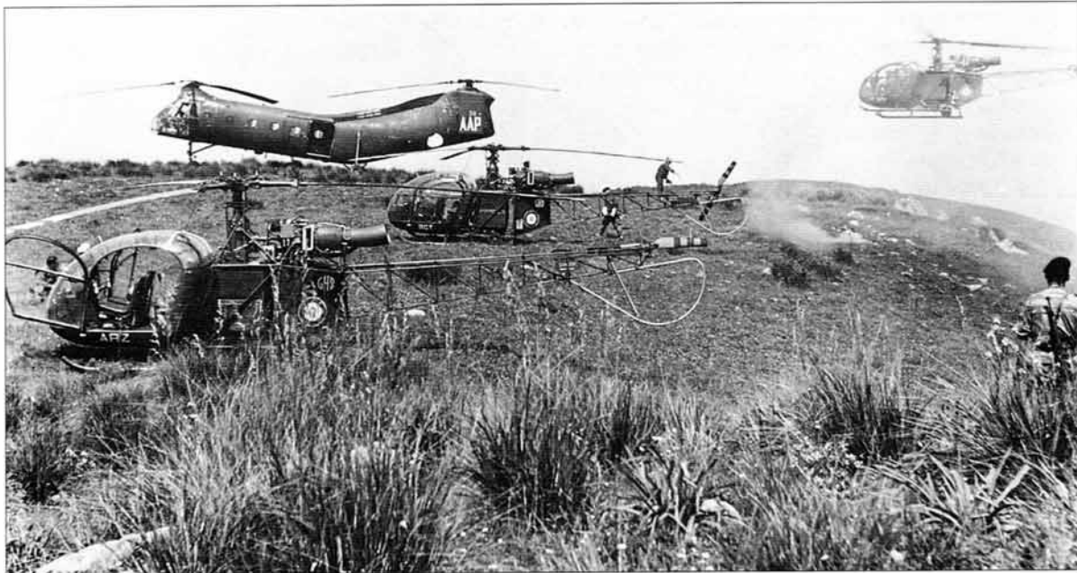
Sud Alouette IIs and a Vertol H-21 'banana' heavy troop carrier during a para operation in the ZEC. The first dozen H-21s, with a 20-man capacity, arrived in late 1957. During 1958 the 'ventilos' were often task-grouped in Helicopter Intervention Detachments comprising four H-21s or six H-34s, a command Alouette, and an H-34 'Pirate' gunship. (Courtesy Jim Worden)
