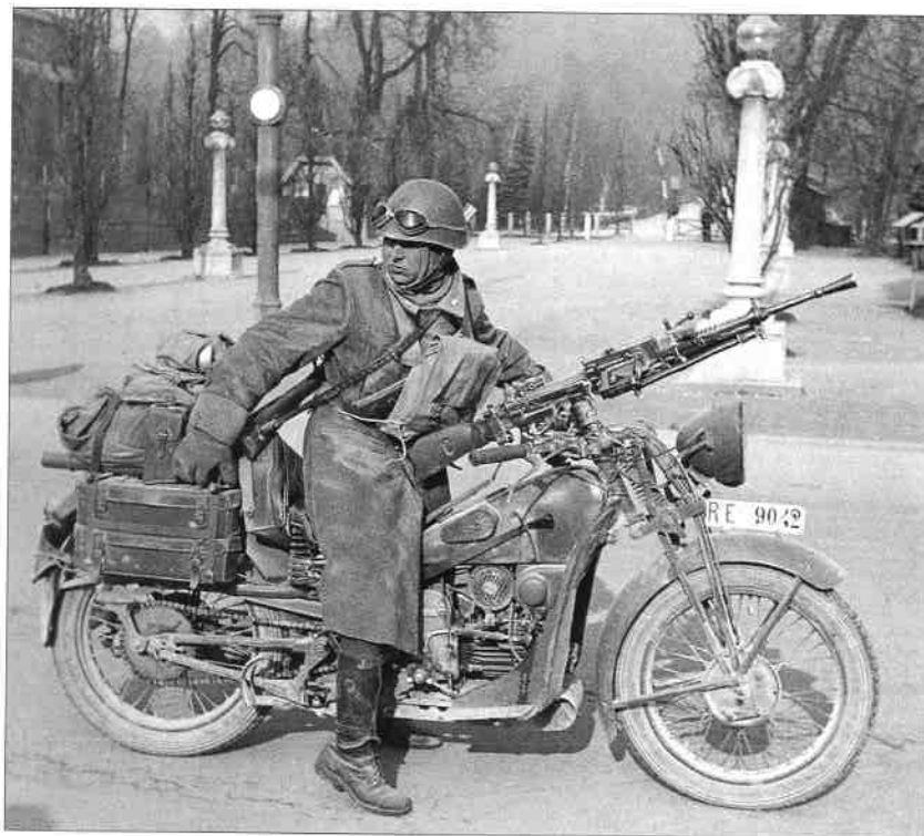
A motorcyclist pauses during the advance into Yugoslavia; his greatcoat is the M1934 model issued to mounted troops, with a larger shawl collar, bigger chest pockets and more flared skirts to allow for riding. His machine is a Moto Guzzi GT17 solo with the Breda 30 light machine gun mounted on the handlebars – a combination in widespread use. (Modern History Museum, Ljubljana)
