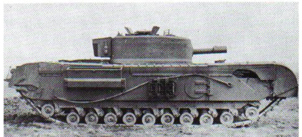
The Mark VIII was very similar to the Mark V, which also mounted the 95mm howitzer, but can
