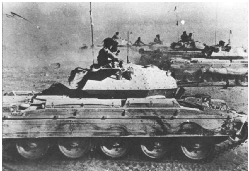
The Mark VI A15 Cruiser Tank 'Crusader' weighed 19 tons and carried a crew of five. It was a fast and good-looking tank but possessed serious faults. It mounted two 7.92mm Besa machine-guns but only a 2-pdr gun with no high-explosive capability and which had already proven grossly inadequate against German armour. Despite a top speed of 26 mph its frontal armour of 40mm was wholly insufficient to protect it against German anti-tank guns and it was mechanically unreliable. (TM 2226/C1)
