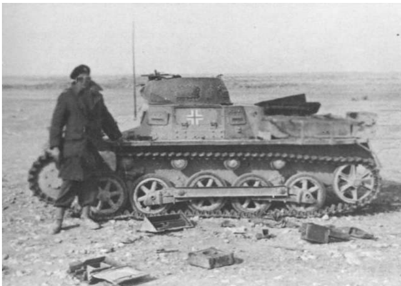
On inspecting this knocked-out Panzer I, this Digger could be forgiven for wondering why so much fuss was being made about the dreaded German panzer forces. The first German tank to go into mass production in 1934, it was obsolete when production stopped two years later. With a two-man crew and a machine-gun armament, its inadequacies did not prevent it seeing extensive front-line service up until 1941. (TM 1335/B5)
