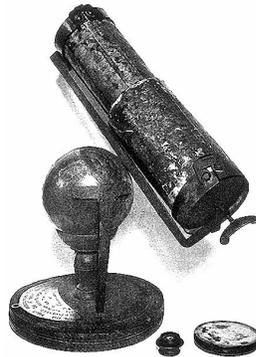
Figure 4.10: Newton's first reflective telescope.
