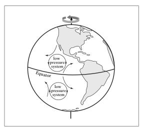
The Coriolis effect is only significant over large distances. A hurricane is born when a low-pressure patch of air draws air in from higher and lower latitudes. Because of the Coriolis effect, in the northern hemisphere the air from the south moves east, and the air from the north moves west, causing a clockwise rotation.
