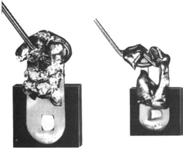
**Figure 3-8** *Inferior wire to lug solder joint*
