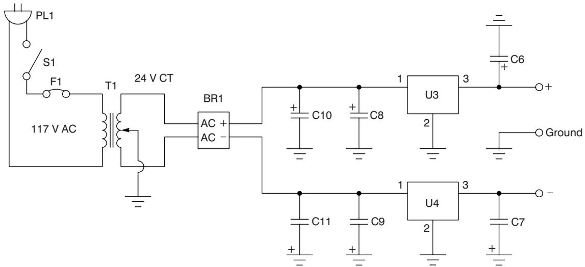
Figure 19-4 Dual voltage power supply
