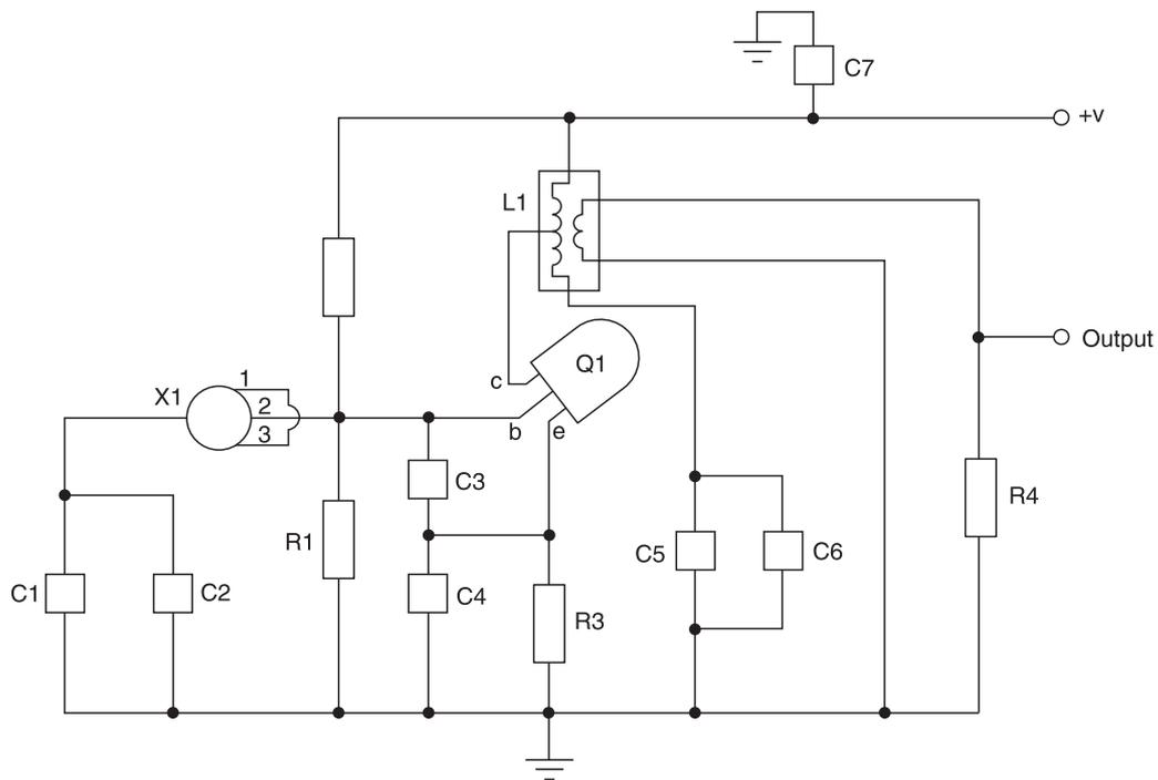
Figure 2-9 Ceramic resonator VFO pictorial circuit diagram
