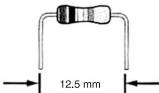
(b) Leads bent down and parallel spaced to match board holes
