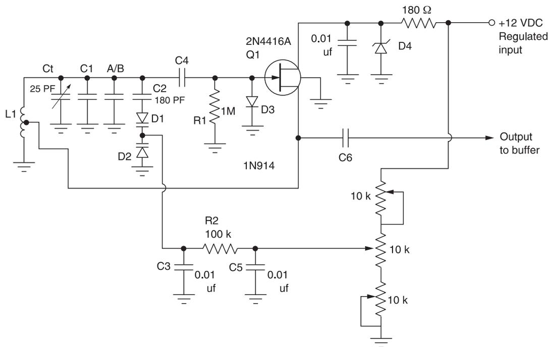
Figure 2-10 Voltage controlled oscillator (VCO) circuit
