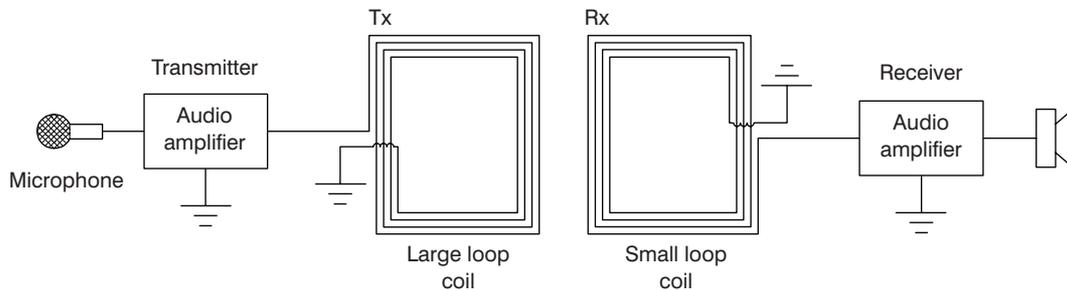
Figure 15-1 Induction loop communications system block diagram
