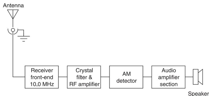
Figure 10-3 10 MHz WWV receiver block diagram
