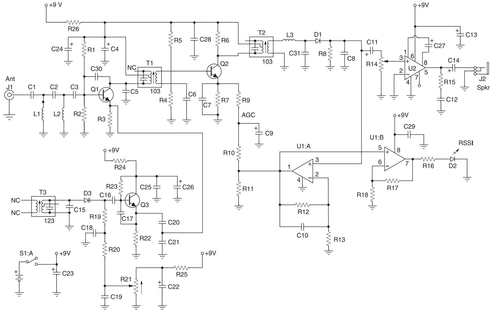
Figure 8-3 Shortwave receiver schematic. Courtesy of Ramsey Electronics
