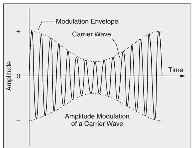
Figure 4-1 *Amplitude modulation*
