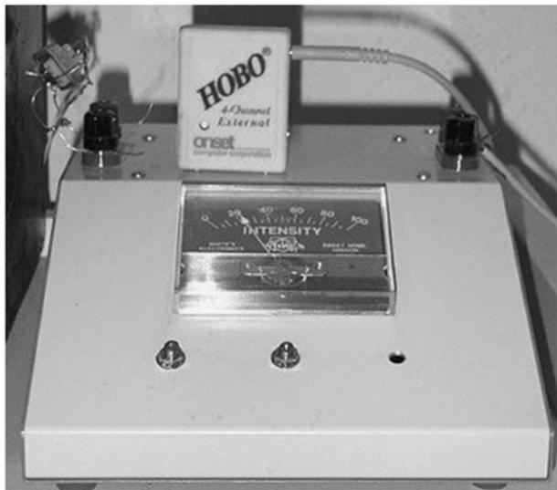
Figure 19-1 Sudden ionospheric disturbance receiver
