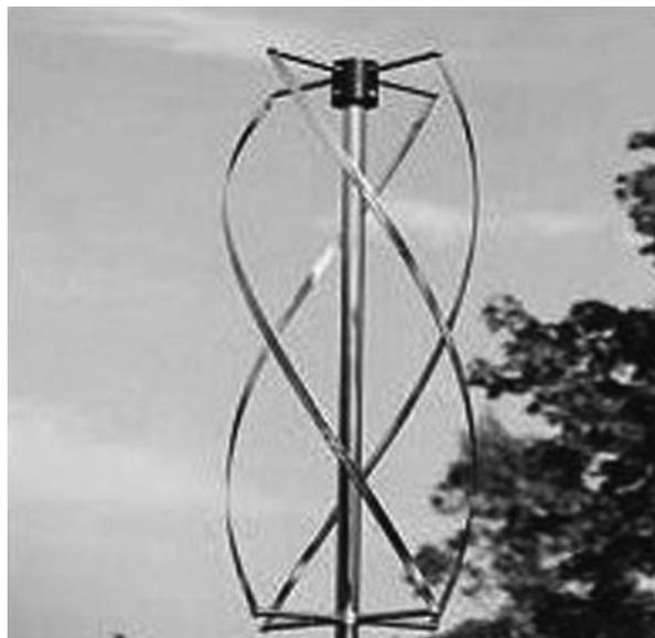
Figure 23-7 Quadrifilar antenna
