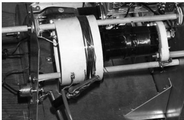
**Figure 7-4** Doerle coil assembly
