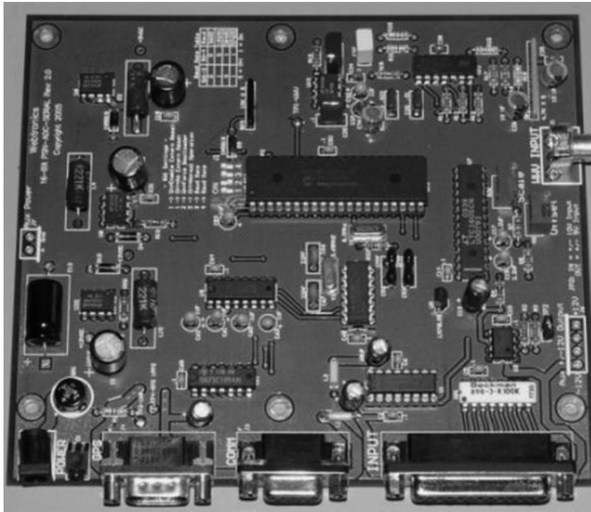
Figure 24-5 16-bit analog to digital converter
