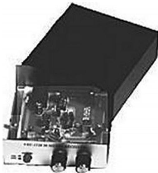
Figure 9-1 80/40 meter code receiver
