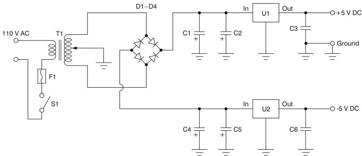
Figure 21-4 ULF receiver power supply
