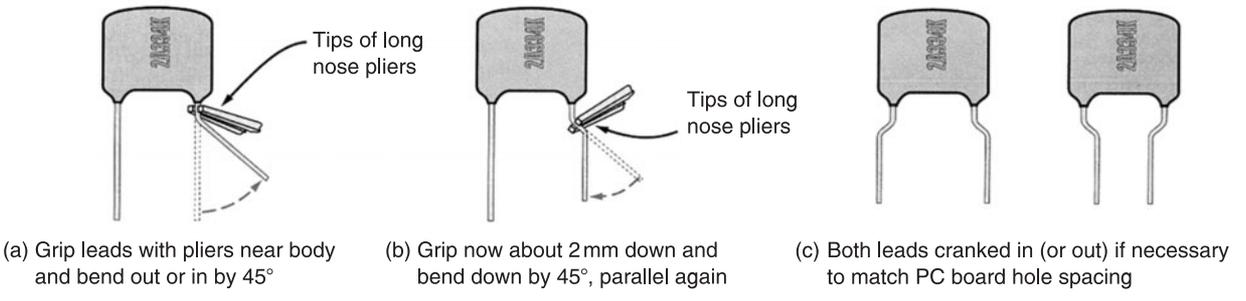
Figure 3-2 "Dressing" capacitor component leads
