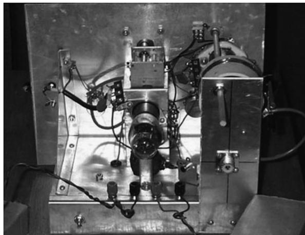
Figure 7-2 *Doerle receiver – inside view*
