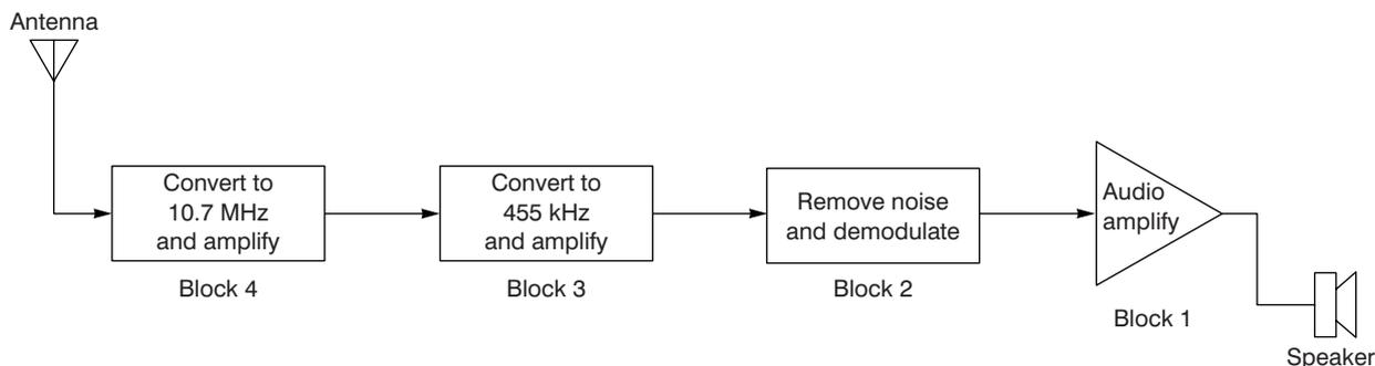
Figure 12-2 *1/2 meter amateur radio receiver block diagram*
