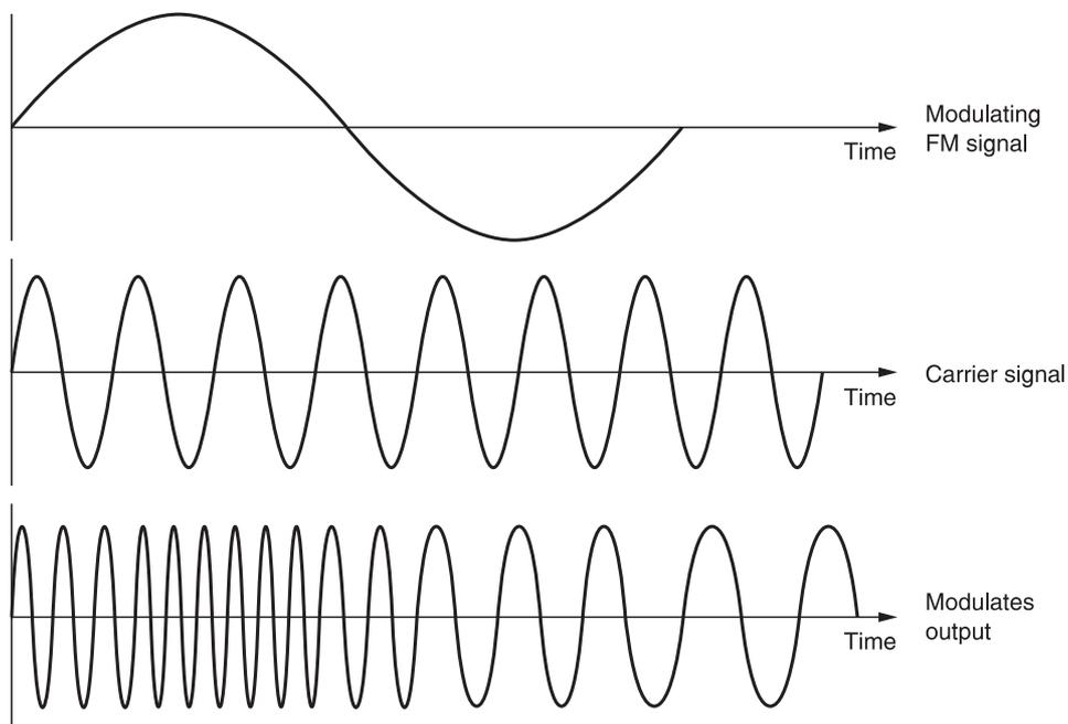
Figure 1-4 *FM modulation waveform*
