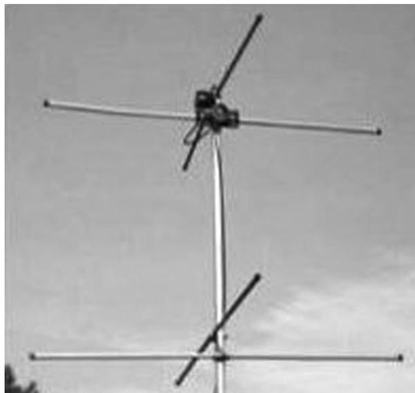
Figure 23-6 VHF turnstile antenna
