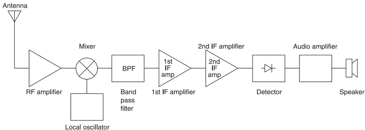
Figure 1-5 AM radio block diagram
