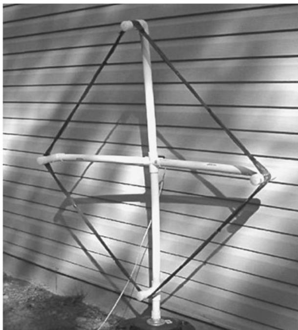
Figure 19-5 Loop antenna
