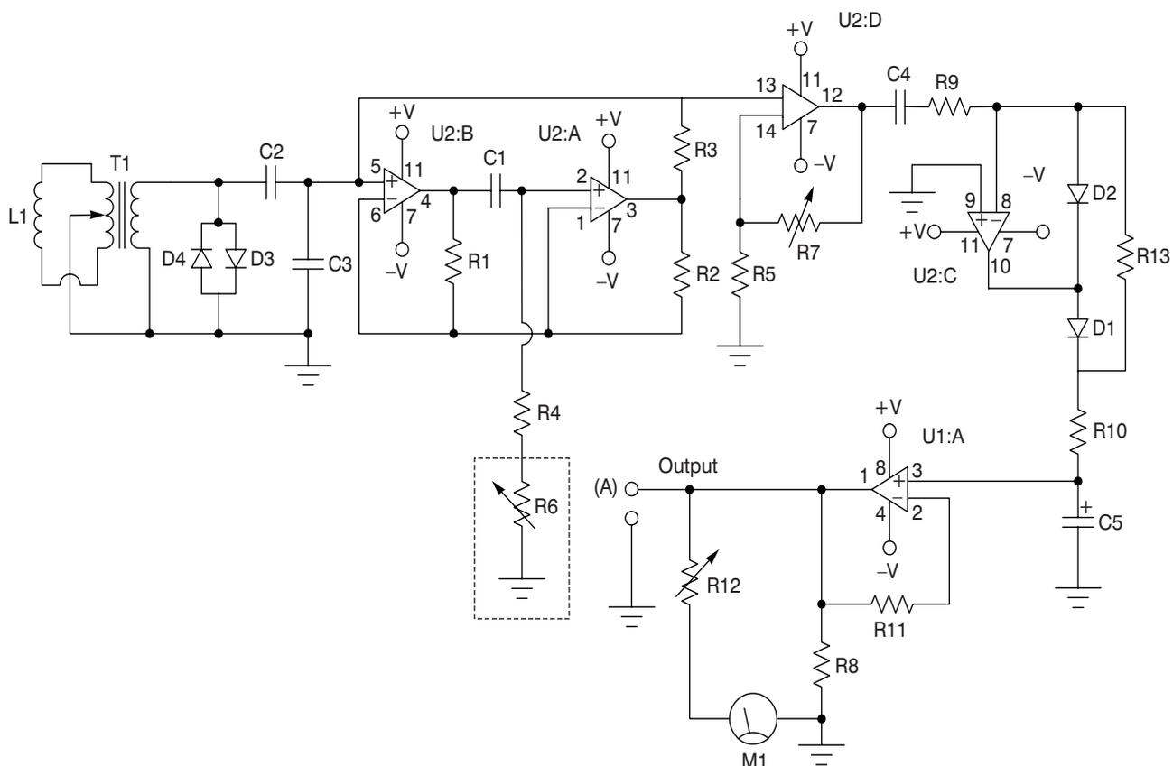
Figure 19-2 Sudden ionospheric disturbance receiver
