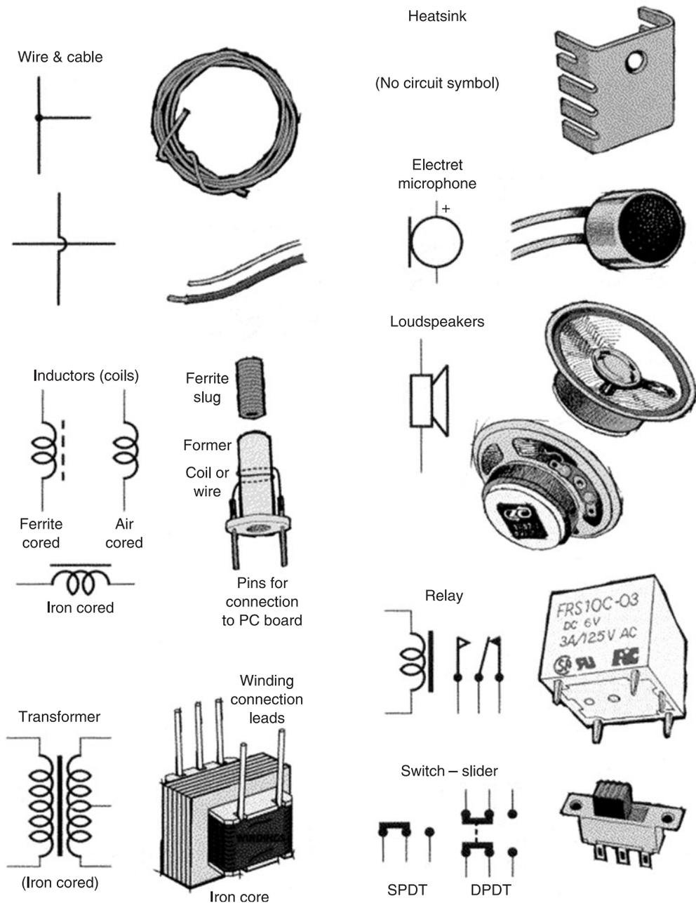
Figure 2-3 *Electronic components 3*
