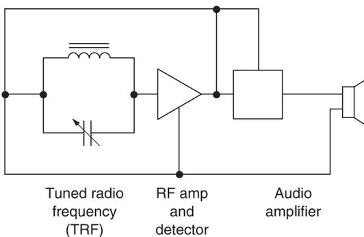
Figure 5-4 TRF AM radio block diagram
