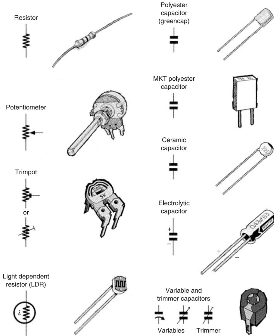
Figure 2-1 *Electronic components 1*
