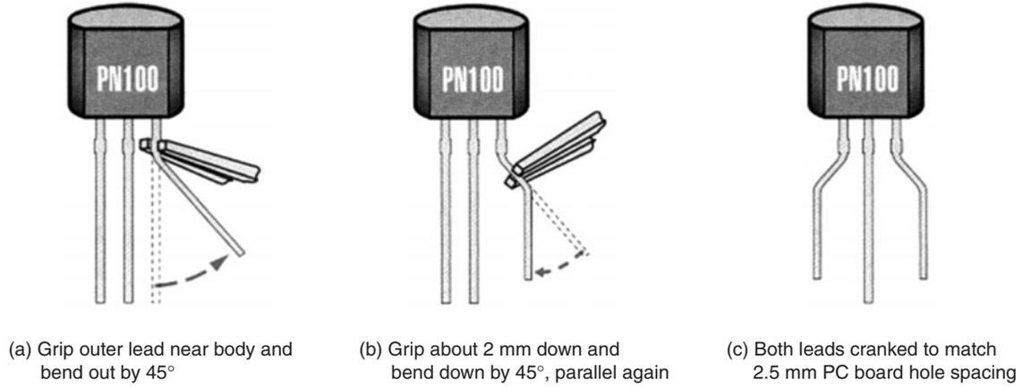
Figure 3-4 "Dressing" TO-92 transistor leads
