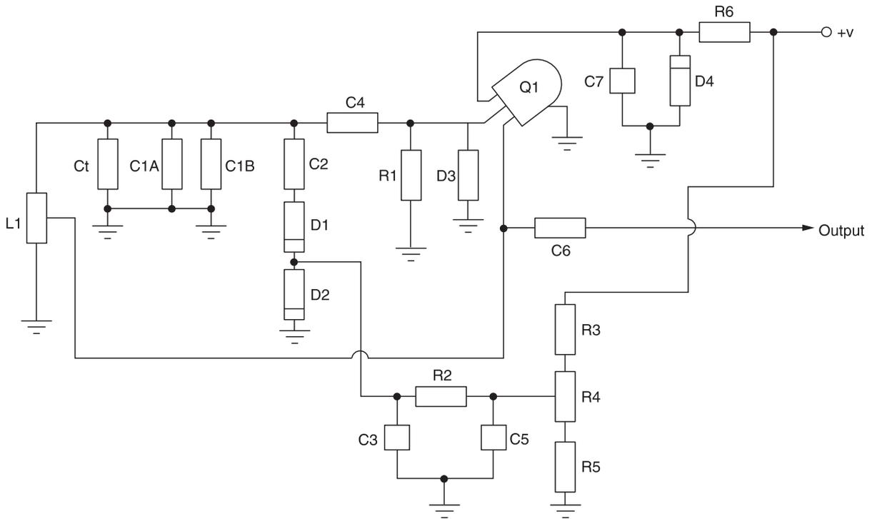
Figure 2-11 Voltage controlled oscillator (VCO) pictorial diagram
