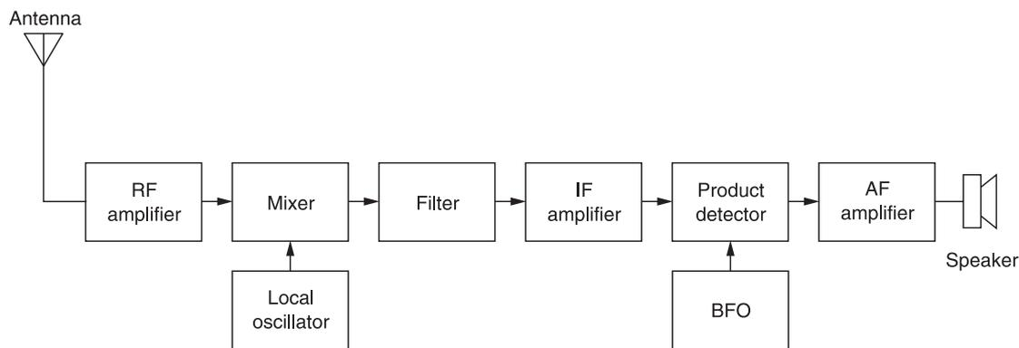
Figure 1-8 SSB shortwave receiver block diagram
