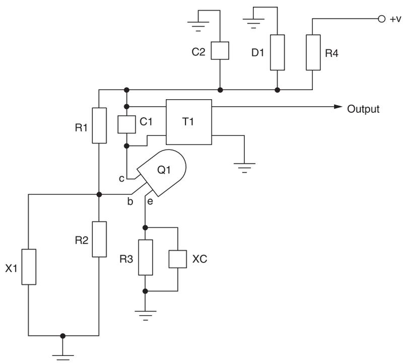
Figure 2-7 Crystal oscillator pictorial diagram
