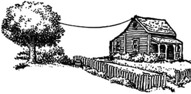
Figure 17-3 *Horizontal long-wire antenna*
