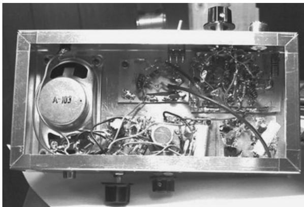
Figure 10-2 WWV time code received – inside view
