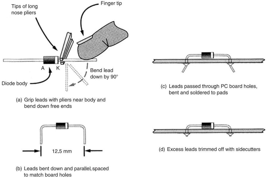
Figure 3-3 Preparing diode leads for horizontal mounting
