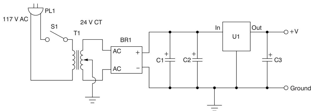
Figure 18-9 Magnetometer power supply
