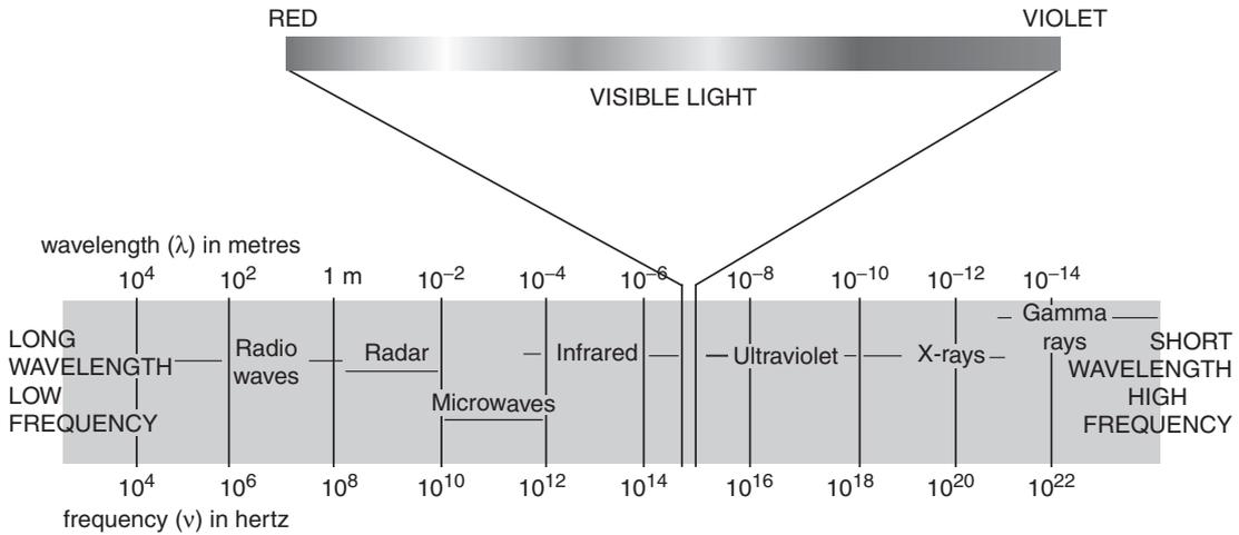
Figure 1-1 *Electromagnetic spectrum*
