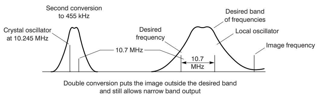
Figure 12-3 Single vs. double conversion receiver
