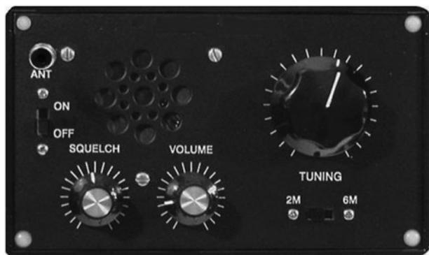
Figure 12-1 6N2 meter amateur radio receiver
