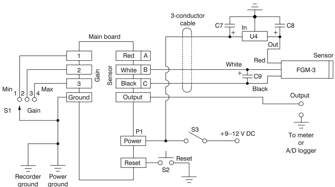
Figure 18-5 Magnetometer connection diagram
