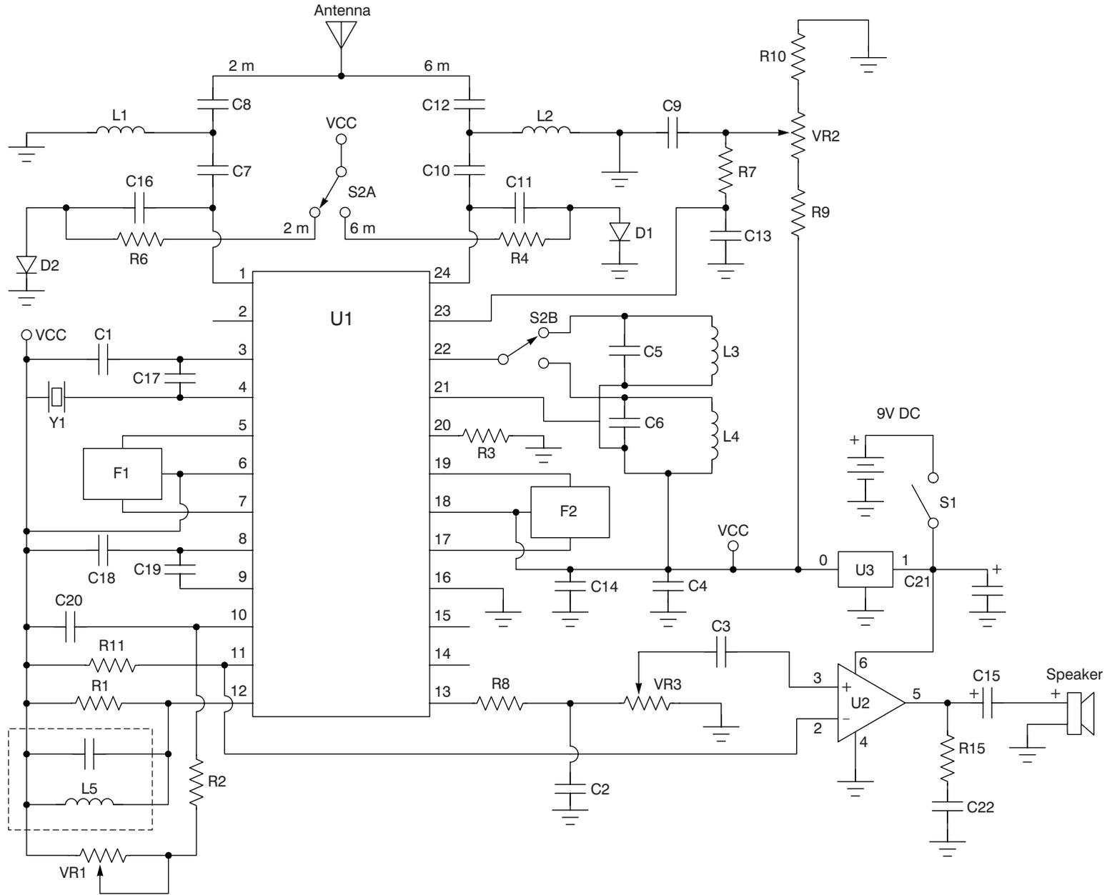
Figure 12-5 VHF public service receiver schematic. Courtesy of Elenco Electronics
