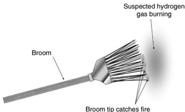
Figure 12-4 Identifying a hydrogen fire with a broom.
