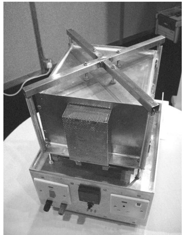
Figure 10-3 1-kW solid oxide fuel cell stack.
