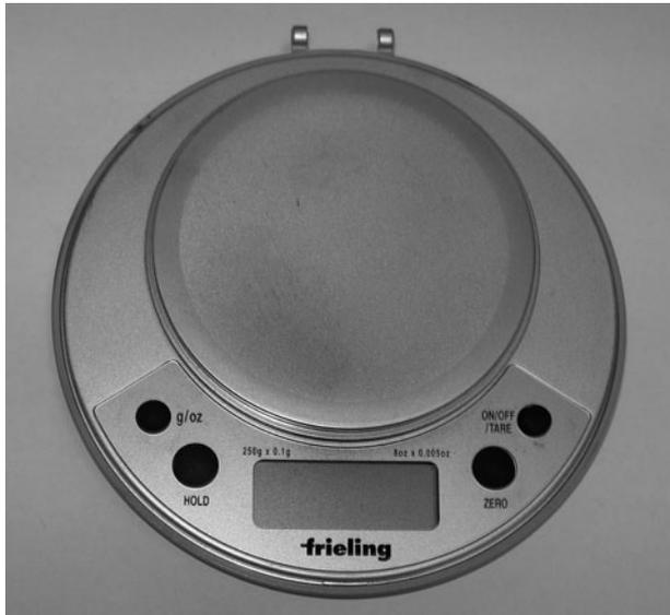
Figure 11-14 Fine scales for carefully measuring chemical quantities.
