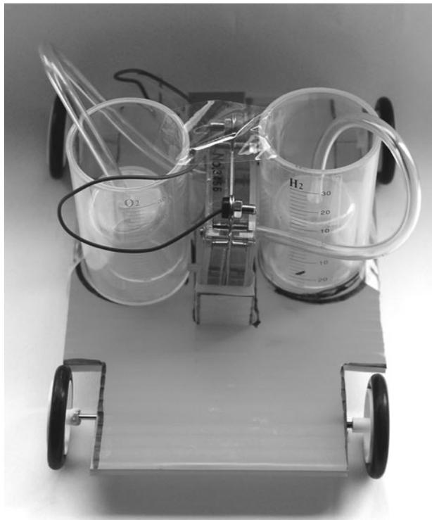
Figure 13-29 *Simple fuel cell car complete (front view).*
