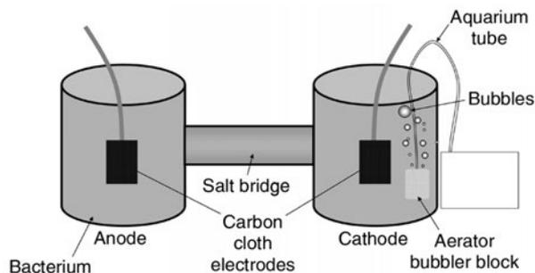
Figure 9-5 *Diagram of the microbial fuel cell.*
