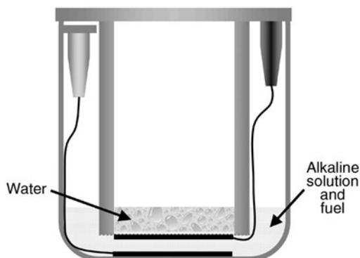
Figure 6-27 *The water blocks oxygen.*
