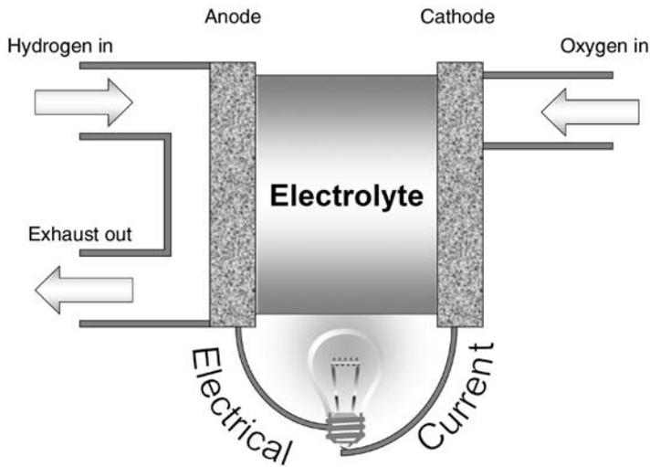
Figure 6-4 Diagrammatic representation of an alkaline fuel cell.
