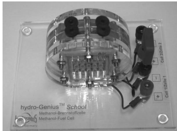
Figure 8-25 DMFC fuel cell suitable for experimentation.
