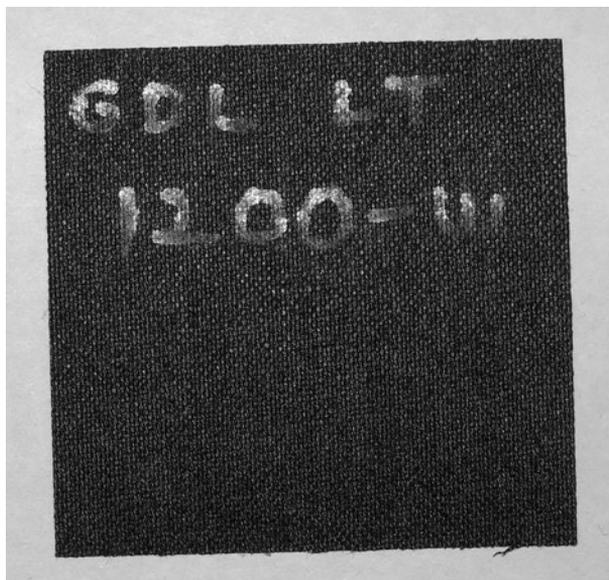
Figure 11-12 A sample of e-Tek gas diffusion layer.
