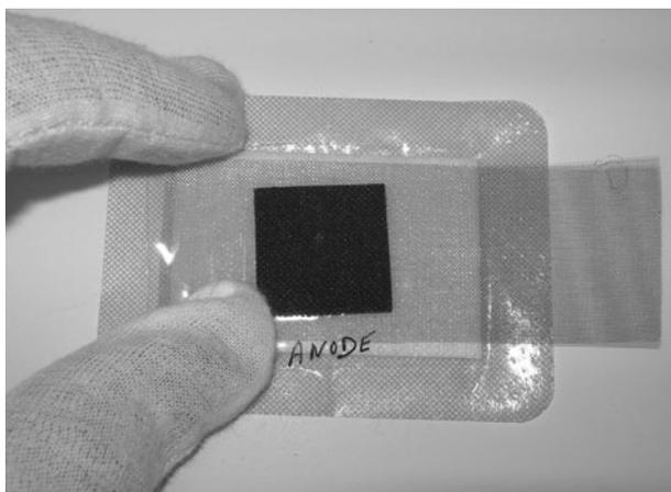
Figure 8-18 Laying the MEA on the wire mesh.
