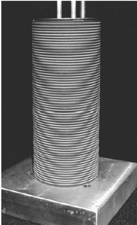
Figure 10-1 Solid oxide fuel cell stack.
