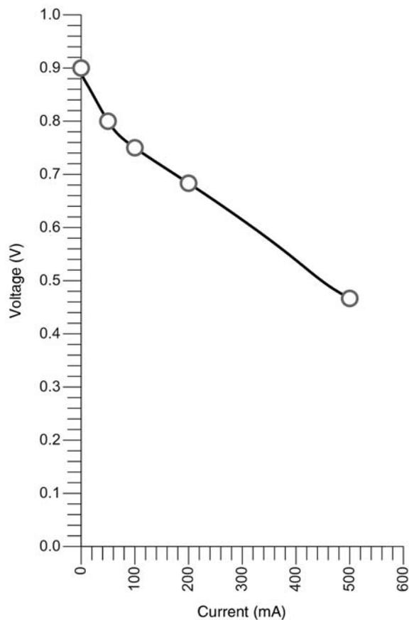
Figure 6-21 Completed graph plotting IV characteristic of the alkaline fuel cell.
