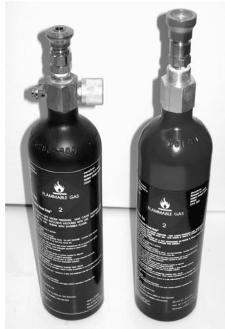
Figure 4-21 Example 1 of metal hydride cylinders.
