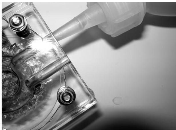
Figure 8-5 *Closeup of filling the methanol fuel cell.*
