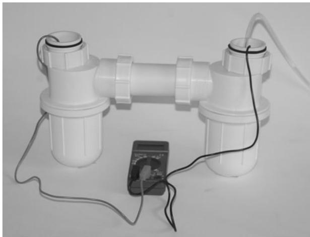
Figure 9-4 *The completed microbial fuel cell.*
