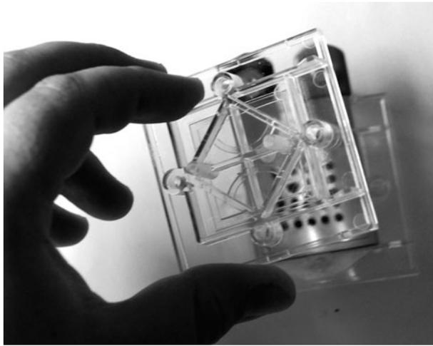
Figure 7-17 Removing the end plate.
