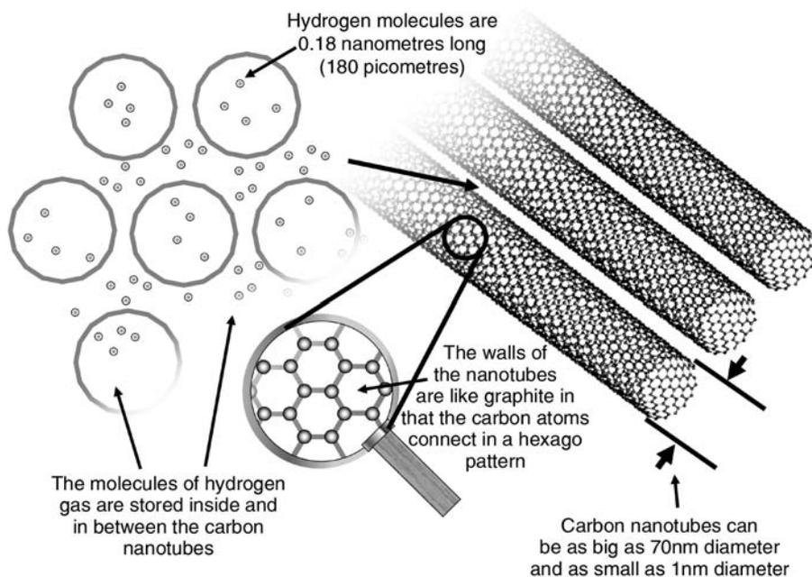
Figure 4-7 *Hydrogen storage in carbon nanotubes.*
