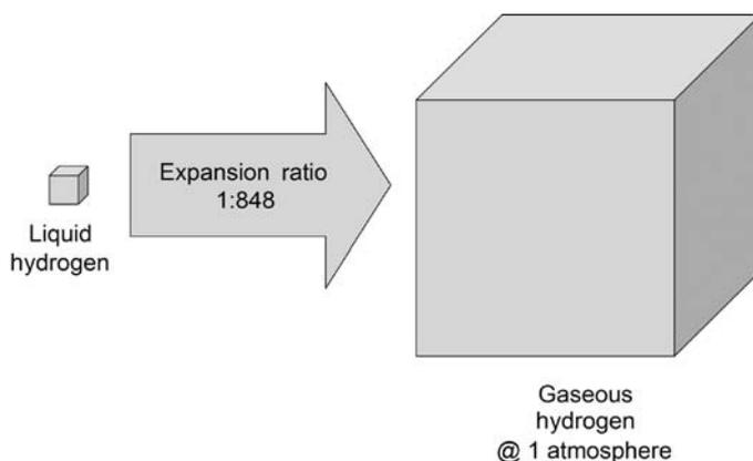
Figure 2-3 The expansion ratio of hydrogen.
