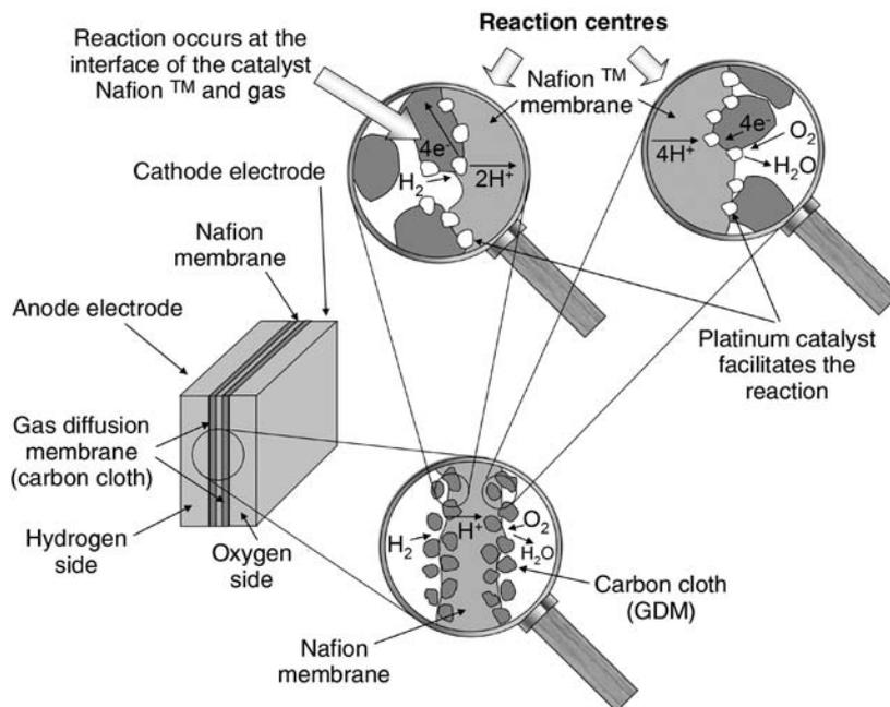
Figure 7-7 What goes on in the middle of the PEM membrane!
