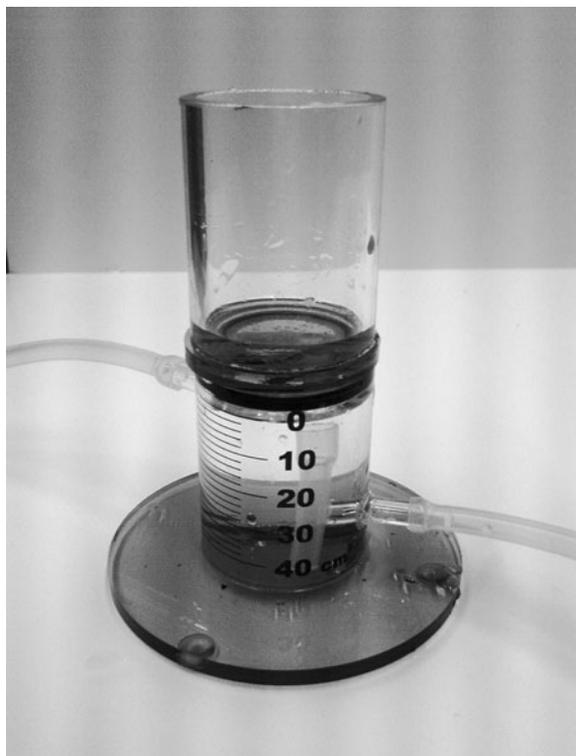
Figure 4-1 Empty hydrogen storage tank.
