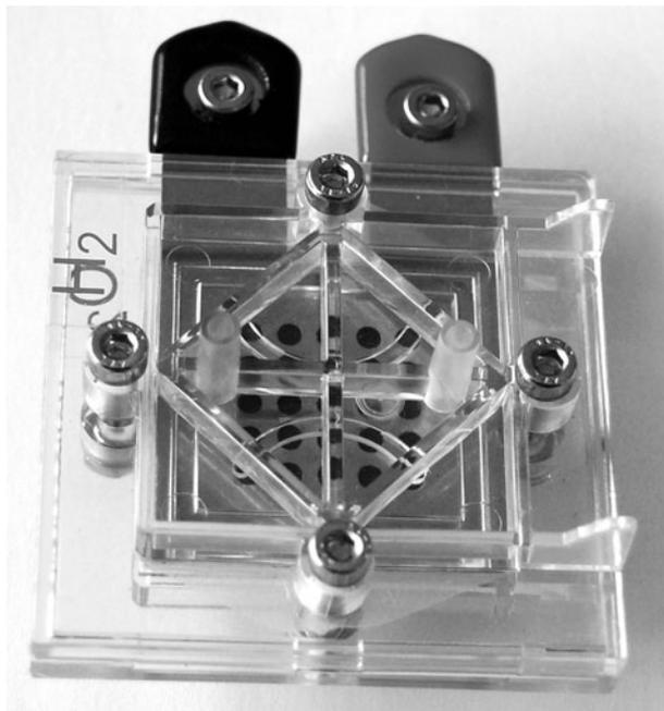
Figure 7-14 *The complete dismantlable fuel cell.*
