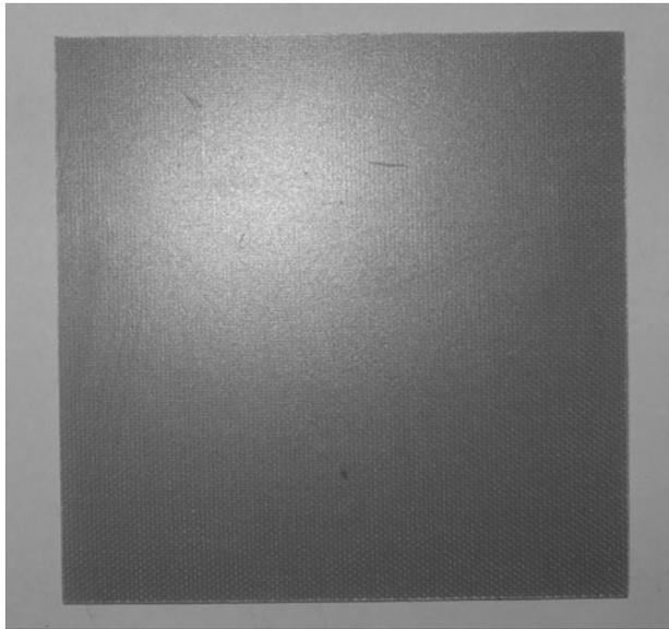
**Figure 11-1** *Fiberglass sheet suitable for end-plate fabrication.*
