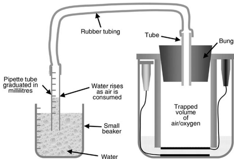
Figure 6-29 The oxygen consumption measurement apparatus.
