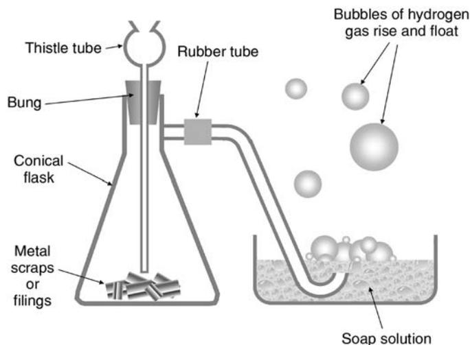
Figure 14-5 *Making hydrogen bubbles.*
