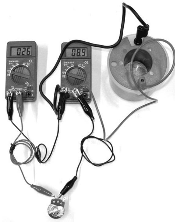
Figure 6-18 The alkaline fuel cell measurement setup.
