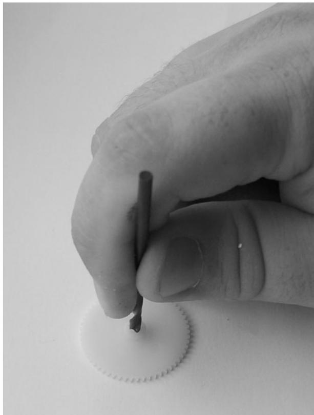
Figure 13-26 Use a small drill to enlarge the axle hole.
