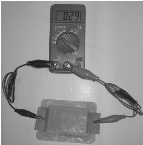
Figure 8-23 The Band-Aid fuel cell connected to a meter.
