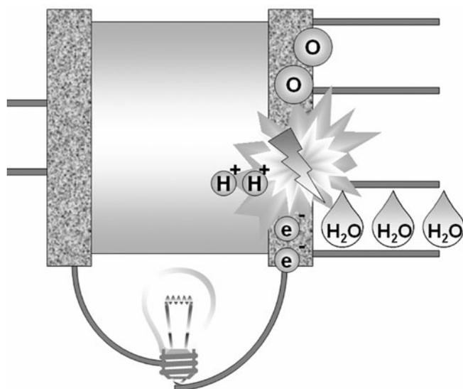
Figure 7-6 *The electrons, protons, and oxygen combine to form water.*
