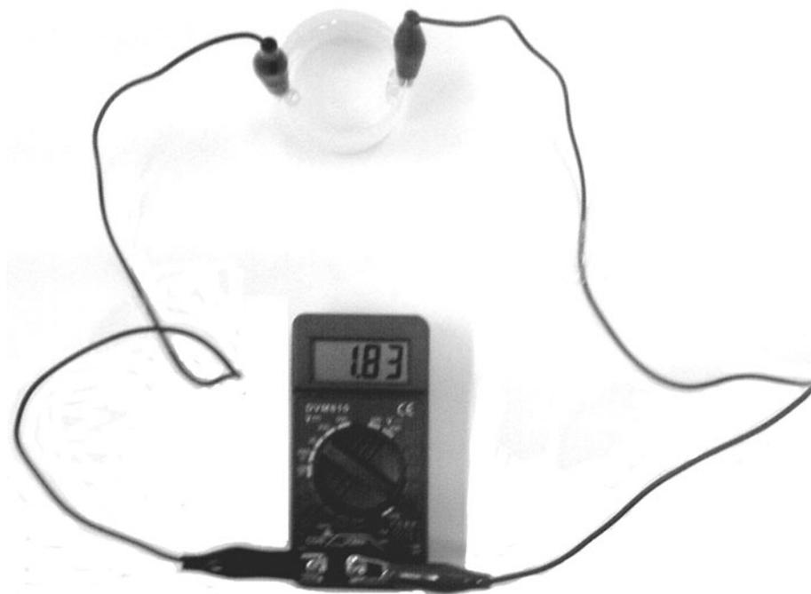
Figure 5-8 The platinum fuel cell generating electricity.
