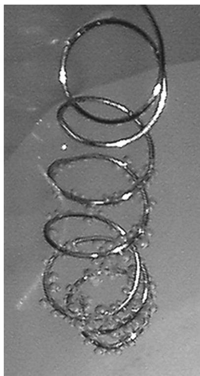
Figure 5-9a Close-up of the the oxygen electrode.
