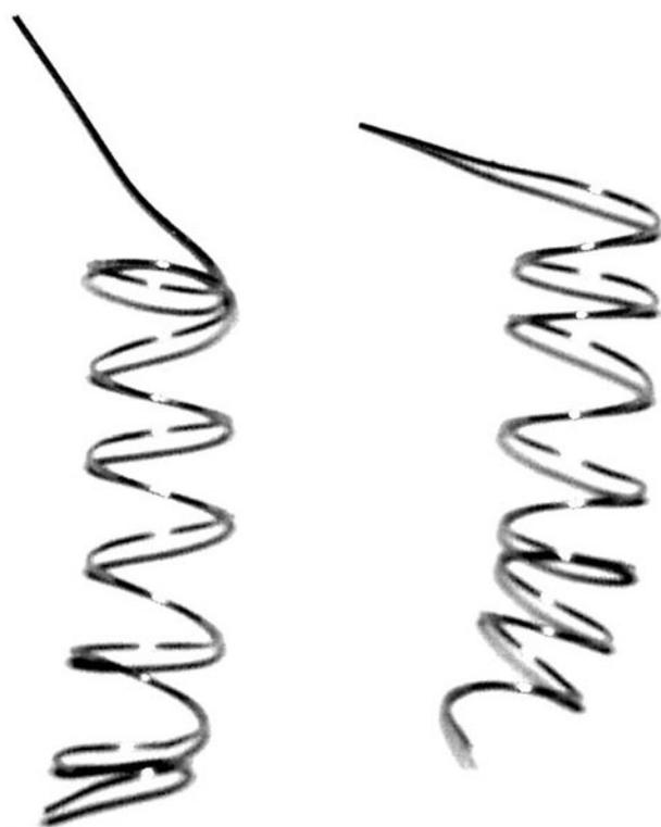
Figure 5-2 Two small coils of platinum wire.
