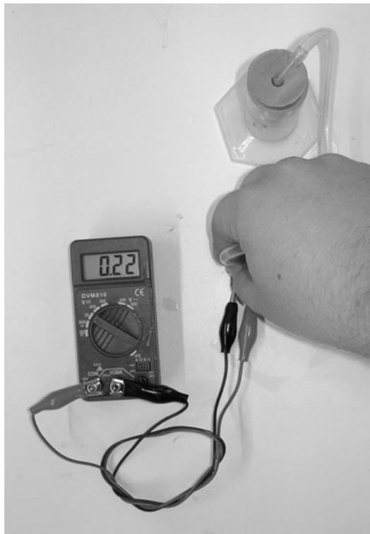
Figure 7-33 Use a multimeter to check power is being produced.
