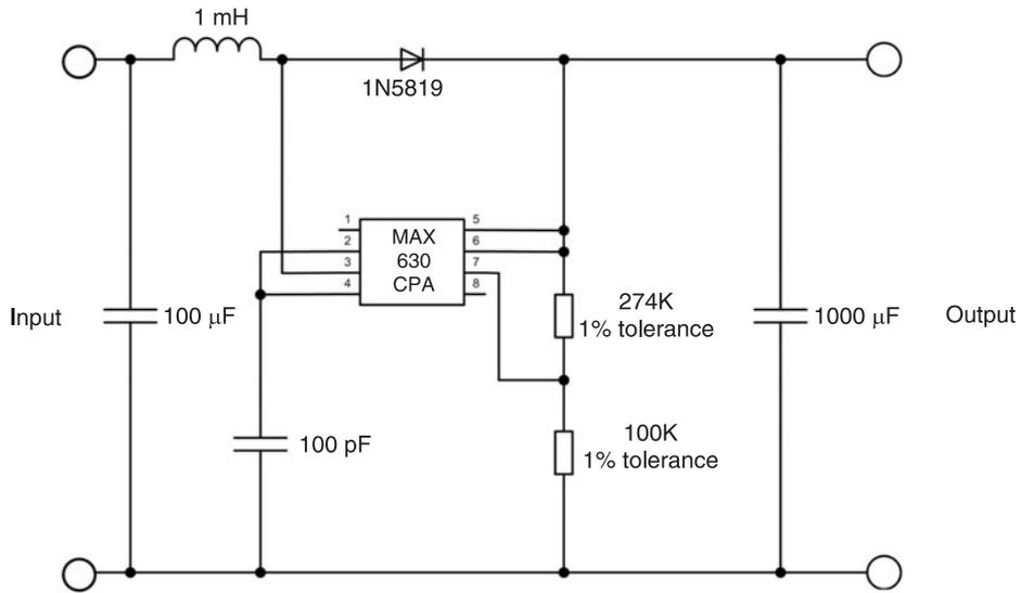
Figure 13-45 DC-DC converter board schematic.
