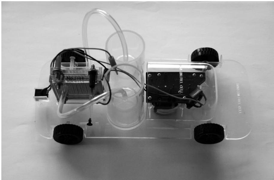
Figure 13-38 The complete "intelligent" fuel cell car.
