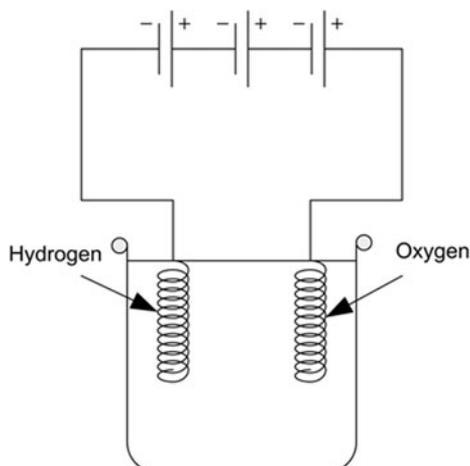
Figure 5-5 Schematic for generating hydrogen and oxygen.
