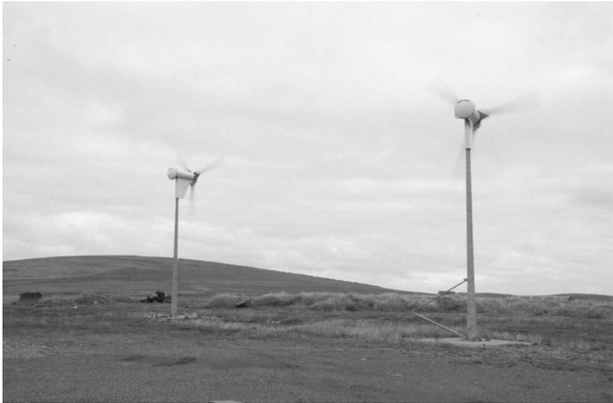
Figure 3-12 Two 6-kW proven wind turbines.
