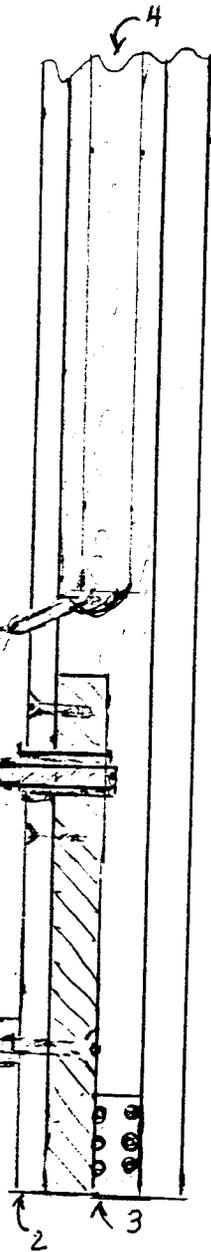
11) Are six U shaped pieces of 1/32" thick copper clips. These clips are secured 1/2" from the end of each blade measuring 3/8" wide with the open end on the inner side. These clips serve as contacts and should be shaped on the outer surface to form a curved radius measuring 4-5/16 inches.
