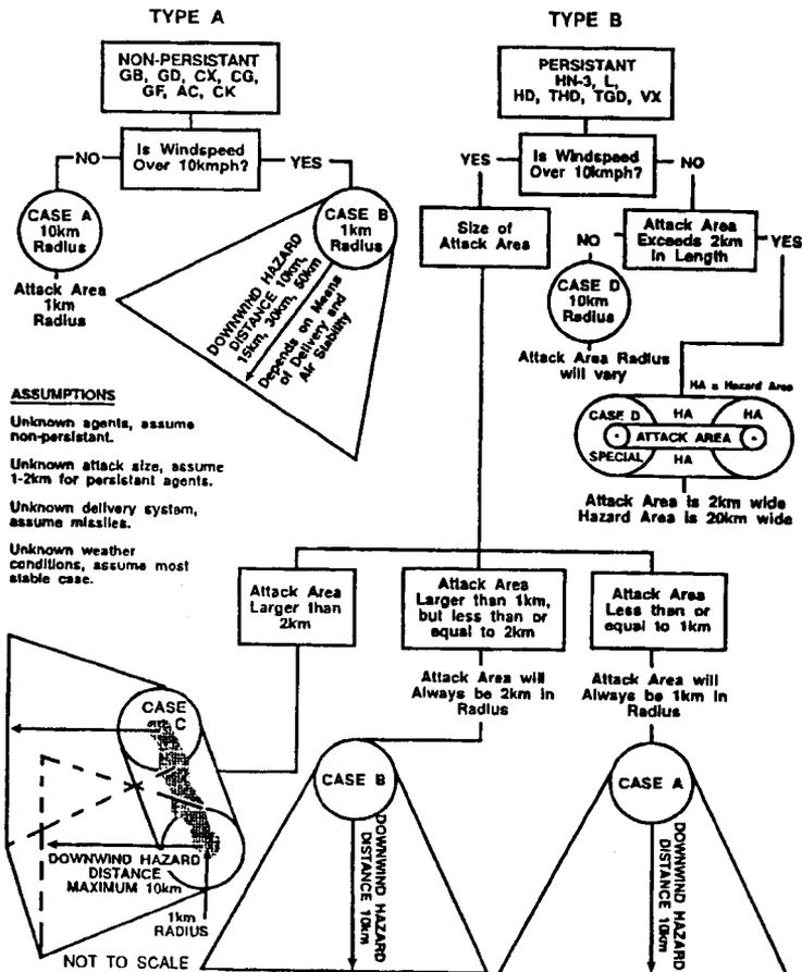
Figure 2-1. Flow chart. Chemical Hazard Prediction
