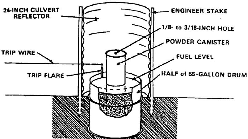
*Figure 7-6. Cutaway showing composition of a Husch flare.*
