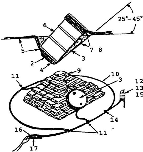
**Figure 7-3. Fougasse made with a 55-gallon container.**
