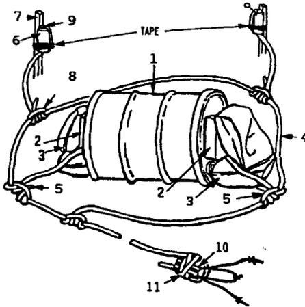
**Figure 7-2. Example of a horizontal flame mine.**
