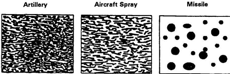
*Figure 1-1. Heavy liquid contamination on M9 paper.*
