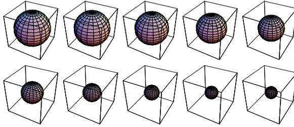
Figure 5.5: Monopole fluctuations of a liquid drop
