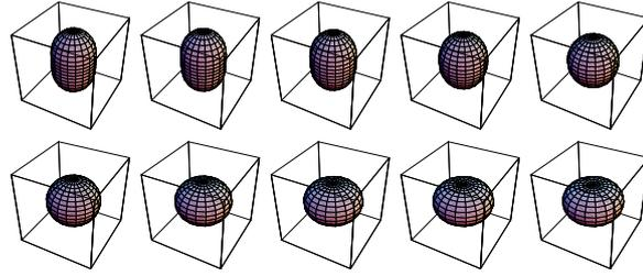
Figure 5.7: Quadrupole fluctuations of a liquid drop
