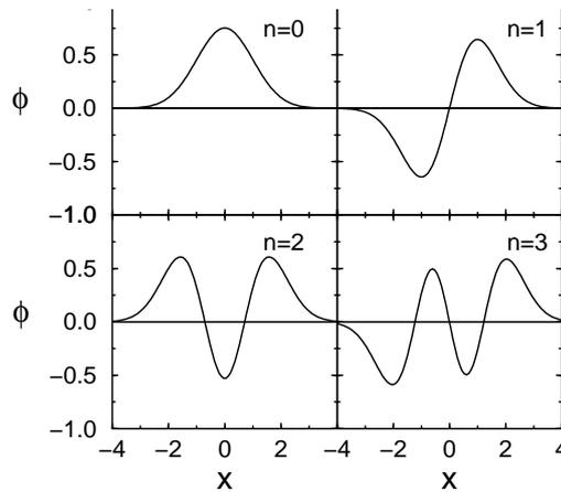
Figure 8.2: The first four harmonic oscillator wave functions
