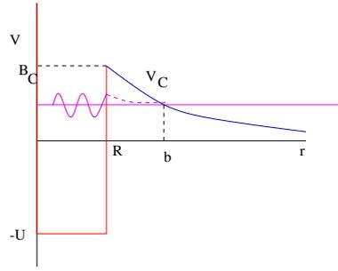
Figure 5.12: The potential energy for alpha decay
