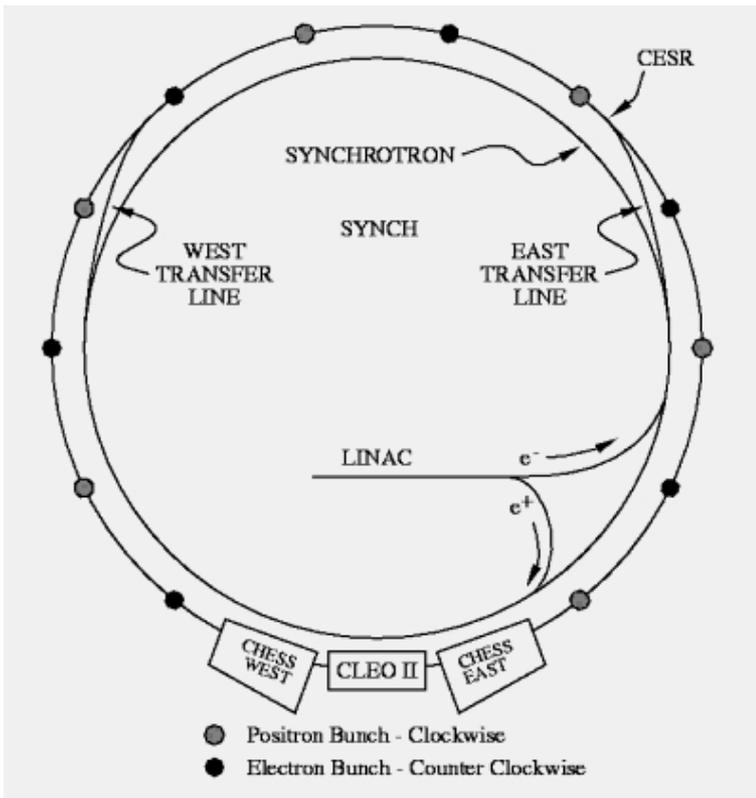
Figure 3.10: A picture of the Cornell accelerator
