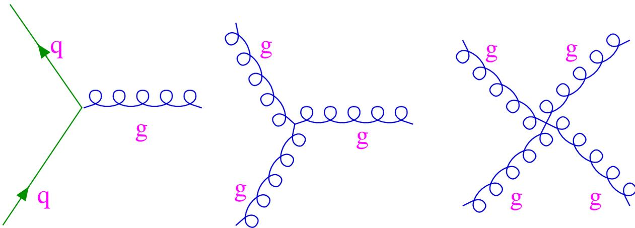
Figure 9.11: The basic building blocks for QCD feynman diagrams
