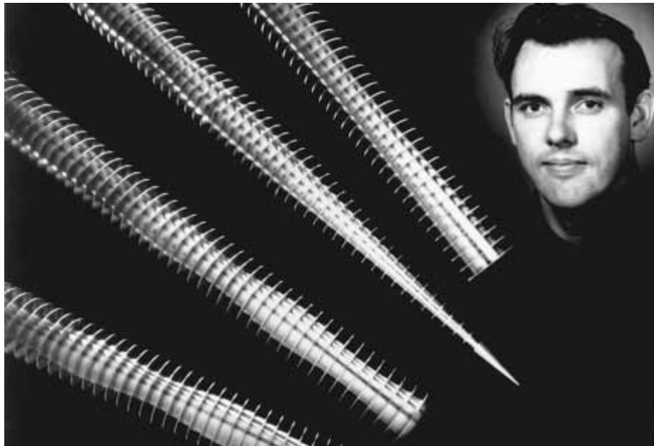
Figure 1-10 George Hockham with the metal waveguides he made to model waveguide transmission in fibers. Courtesy BNR Europe
