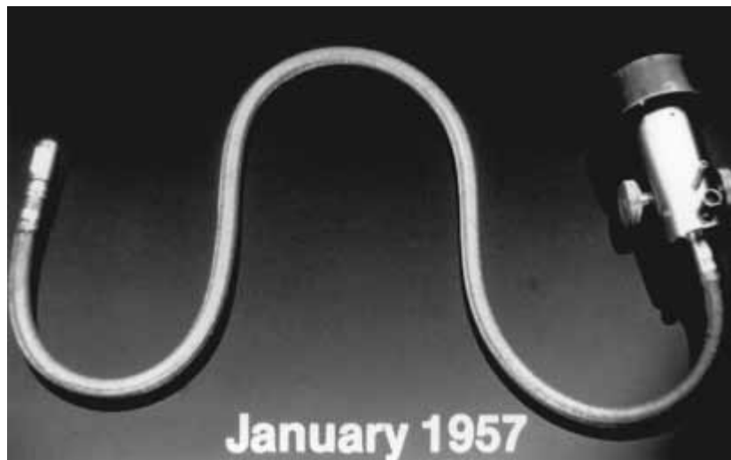
Figure 1-8 Prototype fiber optic endoscope made by Lawrence Curtiss, Wilbur Peters, and Basil Hirschowitz at the University of Michigan. Courtesy Basil Hirschowitz
