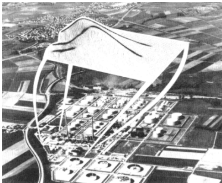
Figure 2.1 Remote Sensing Using Lasers. With lasers it is now possible to detect minute traces of chemicals from a distance. In environmental and energy programs the new techniques can be used to detect pollutants in the atmosphere sensitively and rapidly, to study aerosols and smog, to measure turbulence and wind velocity, and to monitor the stratospheric ozone layer. The techniques can also be employed to study combustion in a furnace or in engines while they operate. The illustration shows a blown-up three-dimensional map of the concentration of ethylene glycol that has leaked to the atmosphere from an oil refinery in Germany. The map is superimposed on an aerial photograph of the refinery. (The long arrows illustrate the points on the ground that correspond to the corners of the map.) The gas leak was mapped with a laser 0.5 kilometer away from the plant. The sensitivity of the measurement is 20 parts in 10^9 . The peaks in the map reveal two sources of escaping gas. The gas is not coming from the two smokestacks that can be seen in the photo, however: the sources were pinpointed to be two leaks in separate buildings. (Photo courtesy of Max-Planck-Institute for Quantum Optics, Garching, Federal Republic of Germany.)
