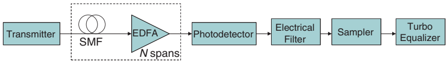
Fig. 7.13 System description for study of chromatic dispersion compensation based on LDPC-coded turbo equalization
