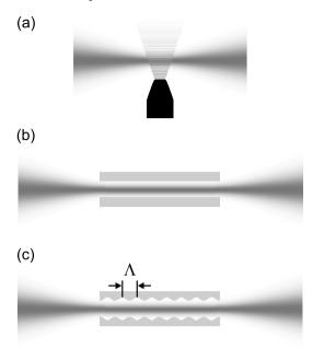
**Fig. 8.1.** Geometries for high-harmonic generation from atoms (schematically, not to scale). (a) The laser pulse interacts with the atoms of a gas jet (a geometry used by many authors), (b) the atoms in a hollow gas capillary [230, 231] enabling phase matching or (c) with the atoms in a modulated capillary [232] allowing for quasi phase-matching. Λ is the modulation period [269].
