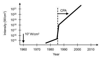
Fig. 1.2. Development of the maximum available focused laser intensity I versus year (schematically). A focused ruby laser in 1960 (see arrow) led to approximately ten million  $W/cm^2$ . The birth of chirped-pulse amplification (CPA) in 1985 is indicated. Thereafter, the intensity has increased approximately exponentially for nearly two decades. Further increase is expected in the future.
