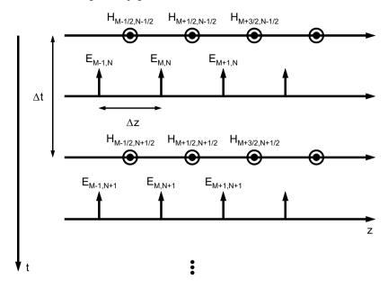
**Fig. 6.1.** Illustration of the one-dimensional finite-difference time-domain (FDTD) discretization and iteration scheme. The spatial step size is  $\Delta z$ , the temporal step size  $\Delta t$ , M and N are integers. The electric field E is parallel to the x-direction, the magnetic field H parallel to y (pointing out of the plane), and the wave is propagating along z.
