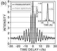
**Fig. 7.2.** Experiment: (a) measured laser spectrum, (b) measured interferometric autocorrelation. The gray curve in (b) is the autocorrelation computed from the laser spectrum under the assumption of a constant spectral phase (no chirp). The inset in (b) depicts a 4.8-fs full width at half-maximum real-time intensity profile computed under the same assumption. Figure reprinted from Ref. [54] by permission of O. D. Mücke.
