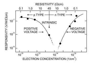
**Fig. 7.25.** Measured responsitivity of eight different germanium photon-drag photodetectors (dots) versus electron concentration under open-circuit conditions. The LHS corresponds to p-type material, the RHS to n-type. Reprinted from Ref. [222] by permission of the American Institute of Physics.
