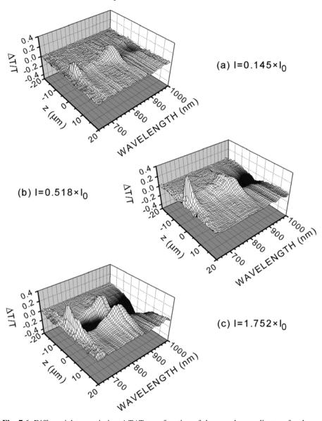
**Fig. 7.6.** Differential transmission  $\Delta T/T$  as a function of the sample coordinate z for three different incident intensities I (referring to z=0). (a)  $I=0.145\times I_0$ , (b)  $I=0.518\times I_0$ , (c)  $I=1.752\times I_0$ . Figure reprinted from Ref. [54] by permission of O. D. Mücke.
