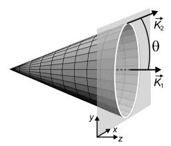
Fig. 7.26. Illustration of the emission characteristics of conical second-harmonic generation (SHG) in an isotropic material. The SHG wavevector  $K_2$  includes an angle  $\theta$  with the fundamental wavevector  $K_1$  (central axis). The depicted angle of  $\theta = 0.35$  (20 degrees) corresponds to  $c(2\omega_0) = 0.94 c(\omega_0)$ . To lowest order, conical SHG is a fifth-order process.
