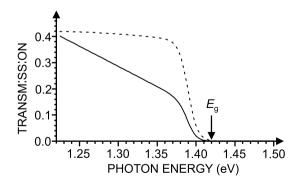
**Fig. 7.24.** Measured transmission spectra of bulk,  $l=350\,\mu m$  thick GaAs with (full) and without (dashed) midinfrared excitation at  $\hbar\omega_0=0.2\,e V$  (equivalent to 6.2 μm wavelength) for an intensity of  $I=3\times10^9~W/cm^2$  corresponding to  $\langle E_{\rm kin}\rangle\approx\hbar\omega_0$ . [269], schematically after Ref. [88].
