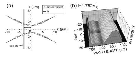
**Fig. 7.5.** (a) Scheme of the z-scan experiment (the measured radii are fitted with the formula  $r(z) = r_{\rm HWHM} \sqrt{1 + (z/z_{\rm R})^2}$  with  $r_{\rm HWHM} = 0.97 \, \mu \rm m$  and Rayleigh length  $z_{\rm R} = 2.9 \, \mu \rm m$ , see Sect. 6.3), (b) transmitted light intensity on a logarithmic scale versus sample position z for an intensity of  $I = 1.752 \times I_0$  (referring to z = 0). Figure reprinted from Ref. [54] by permission of O. D. Mücke.
