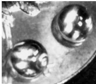
FIGURE 15 Zeonex aspherical lenses made for a \text{NA} = 1.0 miniature microscope cut in this two-axis mode.
