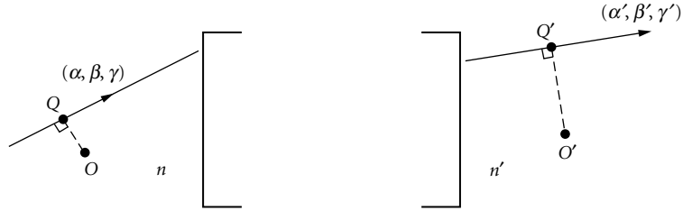
FIGURE 1 Geometrical interpretation of the angle characteristic function for constant object and image space indices. There is, in general, a single ray with directions (\alpha, \beta, \gamma) in object space and (\alpha', \beta', \gamma') in image space. Point O is the coordinate origin in object space, and O' is that in image space. From the origins, perpendiculars to the ray are constructed, which intersect the ray at Q and Q' . The angle characteristic function T(\alpha, \beta; \alpha', \beta') is the path length from Q to Q' .
