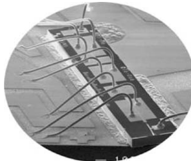
FIGURE 24 Tunable sampled-grating distributed Bragg reflector (SG-DBR) laser with integrated semiconductor optical amplifier and electroabsorption modulator.
