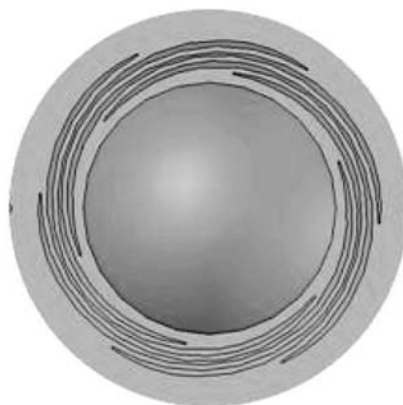
FIGURE 7 Model self-centering lens spring for lens alignment.
