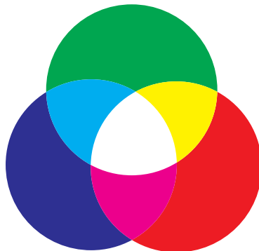
FIGURE 2 Additive color mixing. Simulated overlap of projected red, green, and blue lights. The additive combination of red and green is seen as yellow, red and blue as purple, green and blue as cyan, and red, green, and blue as white.
