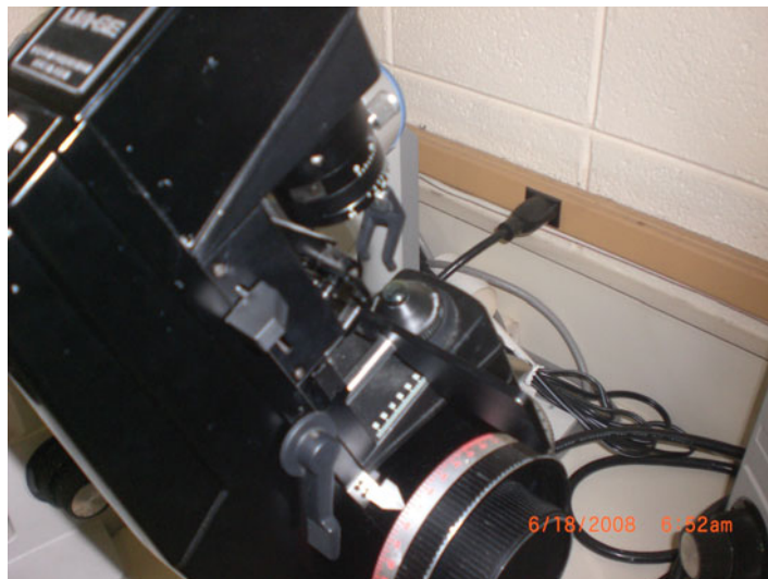
FIGURE 2 Determination of back surface power via the use of a lensometer.
