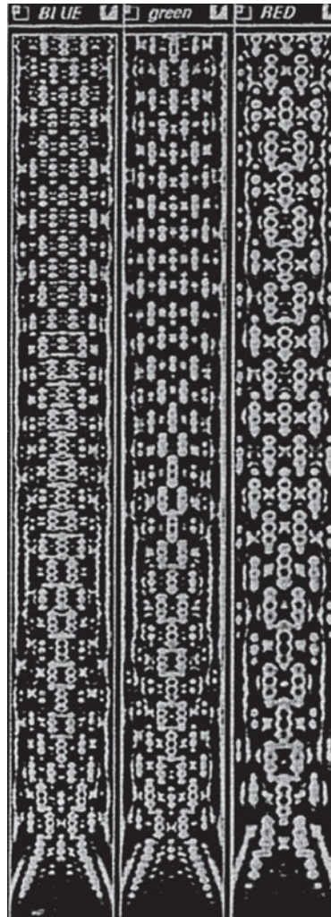
FIGURE 10 Computed figure showing the magnitude of the optical standing wave within a retinal rod at three different wavelengths (475, 505, and 714 nm). White areas are standing wave peaks, dark areas standing wave nulls. (From Ref. 26.)
