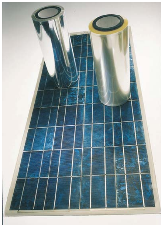
Fig. 10.18 Aspect of the hybrid coated solar cell modules with very high barrier properties (Reproduced by permission of Royal Society of Chemistry) [52]
