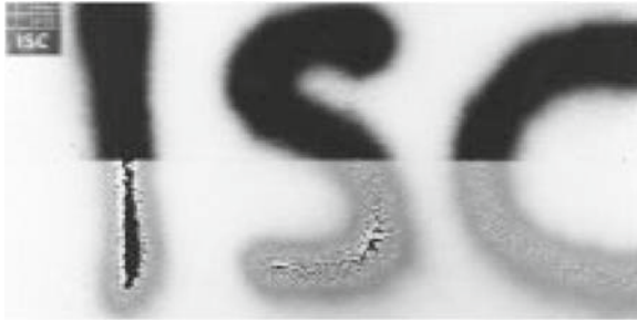
Fig. 10.19 Anti-graffiti effect of an oleophobic organic–inorganic coating on glass towards acrylic spray paint. Top , uncoated glass surface; bottom , hybrid coated (Reprinted with permission from Elsevier) [53]
