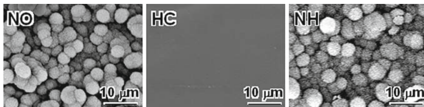
Fig. 16.5 SEM pictures of the MPS-HEMA hybrids prepared with different catalysts before and after soaking in SBF for 7 days
