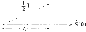
Fig. 12.53 Relative time delay, in a long fiber, of a pulse with polarization vector \hat{\mathbf{S}} .
