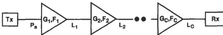
Fig. 14.8 Amplifier cascade. F_i is the noise figure of the i th amplifier. G_i is the optical gain, L_i is the postamplifier loss (splitting and transmission), and P_i is the average optical power at the input of the first amplifier.
