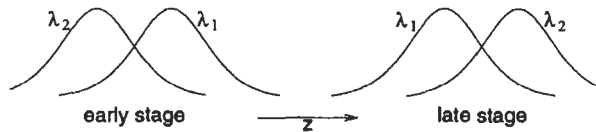
Fig. 12.32 Two stages of a soliton–soliton collision. Because of the anomalous group velocity dispersion, the shorter wavelength soliton ( \lambda_2 ) gradually overtakes and passes through the longer wavelength one ( \lambda_1 ).
