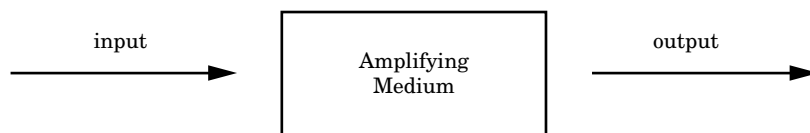
Figure 4.8 All lasers consist of an energized substance that increases or amplifies the intensity of light passing through it. That substance can be a solid, a liquid, or a gas.
