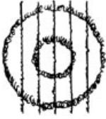
Figure 10.16: Diffraction pattern of two circular holes.
