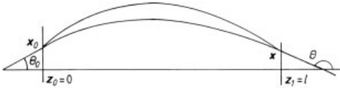
Figure 8.8: Imaging a small surface segment F_0 orthogonal to the optic axis at z_0 = 0 onto a surface segment F_1 at z_1 = l .
