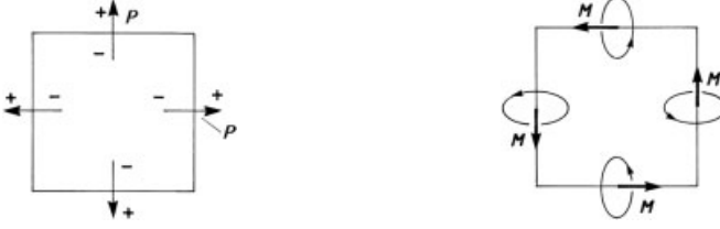
Figure 2.4: (Left) Charges are expelled out of a volume element of the medium due to polarization. (Right) Representation of the magnetic dipole moments by a ring current.
