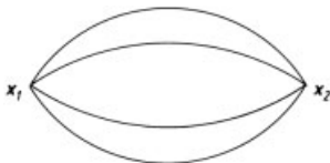
Figure 8.1: Two points are called conjugated if all the rays emitted from one point within a cone of non-vanishing cone angle meet again at the opposite point.
