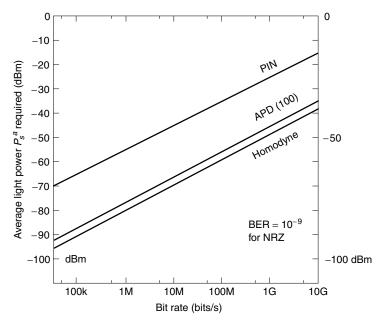
**Figure 16.30** Input average light power  $P_{\rm S}^{\rm a}$  versus bit rate (bits/s) for NRZ code. For the value of the RZ code add 3 dB. The PIN photodiode and APD are thermal noise limited but the homodyne is quantum limited.
