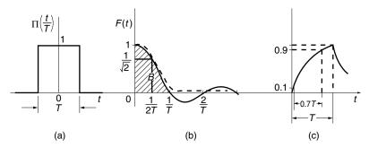
**Figure 16.29** Relationship between NRZ pulse, its Fourier transform, and the output of an amplifier with B=1/2T. (a) NRZ pulse in the time domain. (b) NRZ pulse in the frequency domain. (c) Output from an amplifier with B=1/2T.
