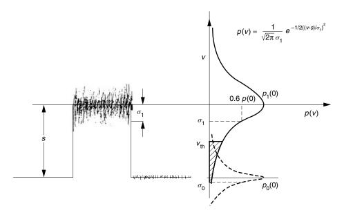
Figure 16.23 Pulse with Gaussian noise in "1." The noise in "0" is suppressed for clarity.
