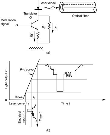
**Figure 16.2** Modulation of laser light by an electrical signal. (a) Circuit for modulating a laser diode. (b) Light output versus injection current (*P–I* curve).
