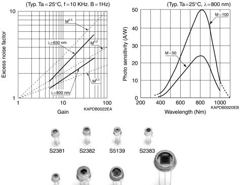
Figure 16.21 APD characteristics. (From Hamamatsu Photonics catalogue [19].)
