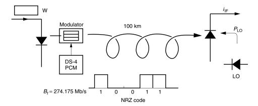
Figure 16.32 Layout of Example 16.5.
