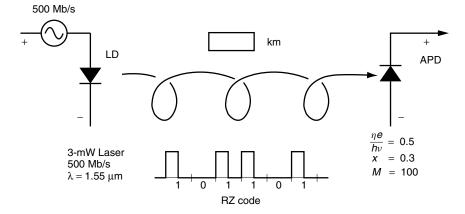
Figure 16.31 Layout of a digital system design.
