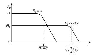
Figure 16.16 Transimpedance coupling.
