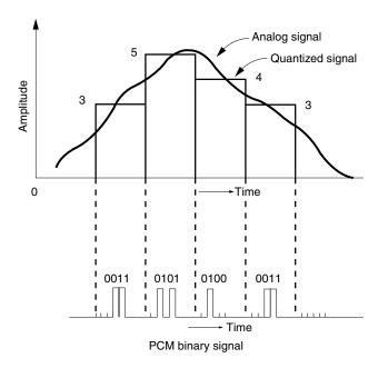
Figure 16.3 Principle of pulse code modulation (PCM).
