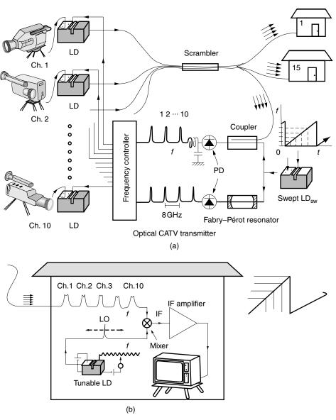
**Figure 16.8** An example of wavelength division multiplexing (WDM) used for sending TV channels. (a) Channel space locking by the reference pulse method. (After S. Yamazaki et al. [17].) (b) Optical heterodyne receiver at home.
