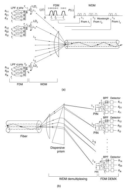
Figure 16.9 (a) WDM combined with FDM. (b) Demultiplexing of WDM combined with FDM.
