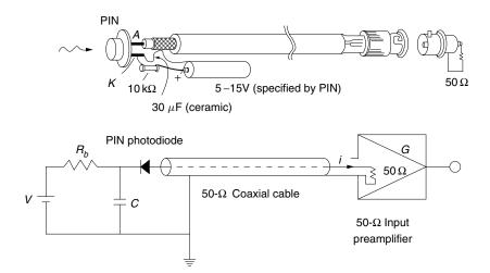
**Figure 16.14** PIN photodiode connected to a  $50-\Omega$  input preamplifier.
