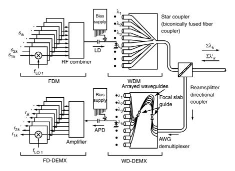
Figure 16.10 Bidirectional WDM combined with FDM.
