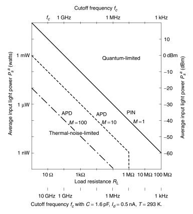
**Figure 16.22** Borderline between quantum-limited and thermal-noise-limited cases of PIN and APD photodiodes.
