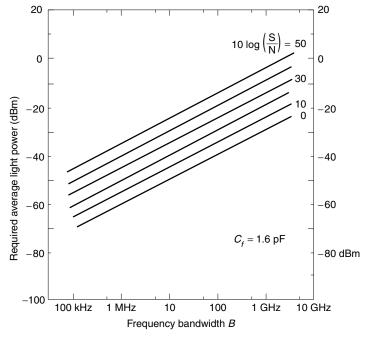
**Figure 16.25** Required average light power of a PIN photodiode as a function of frequency bandwidth B with S/N as a parameter. The modulation is analog and the S/N is thermal noise limited.  $C_f = 1.6 \text{ pF}$ .
