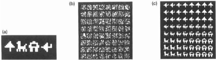
Fig. 7.53. (a) Input patterns. (b) Initial memory matrix space with random noise. (c) Final memory matrix representing a feature map.
