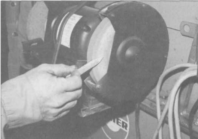
7.24 As with traditional torch cutting, soapstone is useful to mark your cut lines because it won't burn off. With the reduced heat of plasma, you could also use a marker pen. Sharpen the soapstone before drawing.
