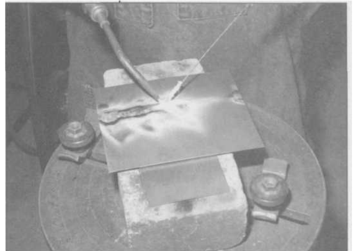
3.35 You should start with very clean metal when brazing, although the flux is designed to surface clean as you go, leaving some minor slag afterwards. You will have to keep the torch further away from the seam than with welding, to keep from overheating the brass.
