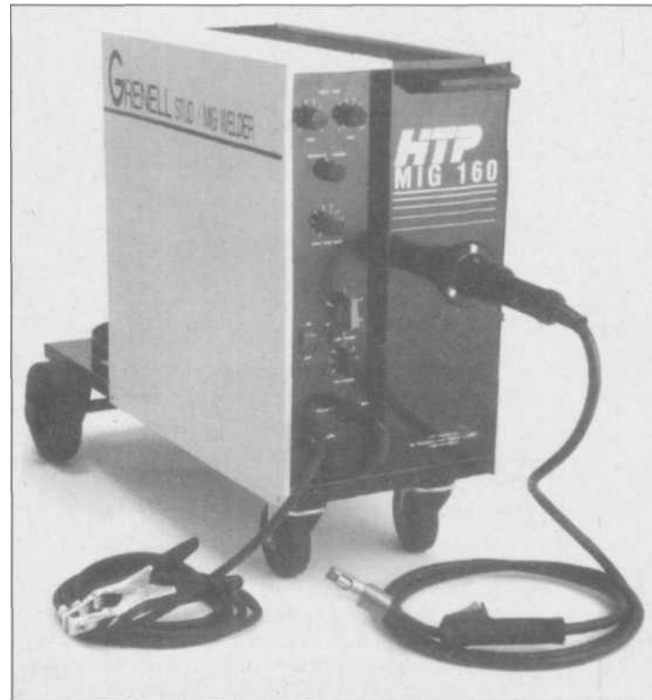
5.22 Above the 140-ampere range, you are into the 220V category of MIG welders, with more features and higher duty capacities. This is HTP's MIG 160 , which can weld up to 5/16-inch steel, has eight heat settings, and is suitable for street rod shops, muffler shops, or farm use.
