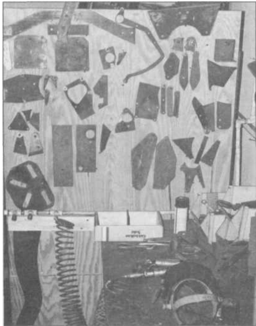
3.49 Wherever you find a flamecutter, chances are you'll find a wall of metal templates nearby, used to easily and precisely duplicate commonly used shapes such as suspension mounting brackets. At lower left is a shape used to make a head for an engine stand.
