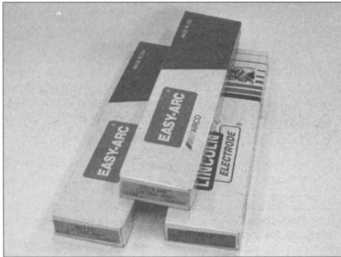
4.26 You'll find a wide variety of electrodes at your welding supply store, but there are only a few rods you will use in normal home/shop projects on mild steel. Don't buy much more than you will need for the next project.
