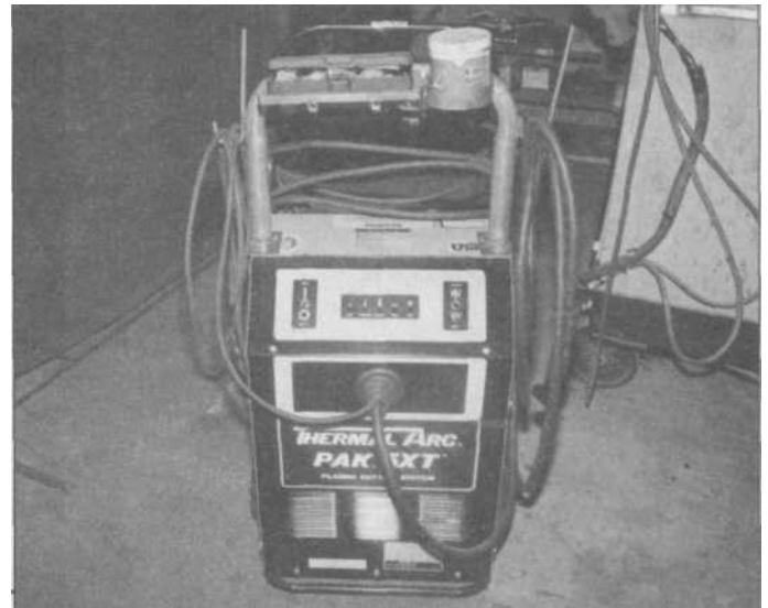
7.18 Hot rodders never leave anything alone. Rugged Thermal Dynamics 50-amp plasma cutter used in a rod shop has been modified with the addition of a tubing rack and box on top to hold nozzle dip and plasma consumables.
