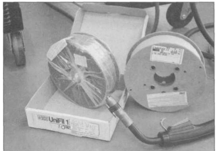
5.36 Your welding supply store will have a variety of MIG electrode wires to choose from. The E70S-6 wire at left is one of the most popular. At right is L-TECs Easy-Grind for body work.
