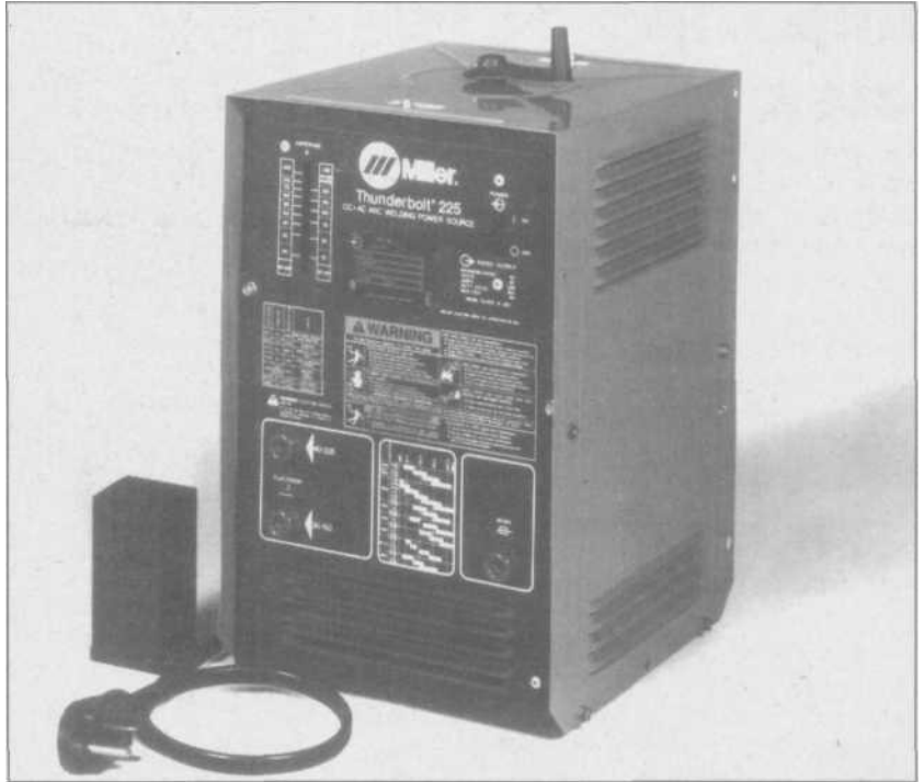
4.3 Another popular AC 220V welding machine for non-industrial use is this Miller Thunderbolt 225. The crank handle on top changes the output amperage, which is read on a scale at the top left of the front panel.
