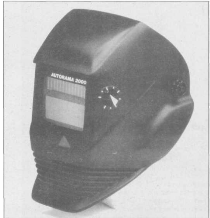
8.6 This Darth Vaderish design from ESAB is the Aurorama 2000, which is one of a modern breed of welding helmet with an automatically-darkening lens. The lens is powered by solar cells, and turns dark as soon as the welding arc begins. These are considered by many weldors to be much easier to use than flipping a helmet up and down to set up each weld.
