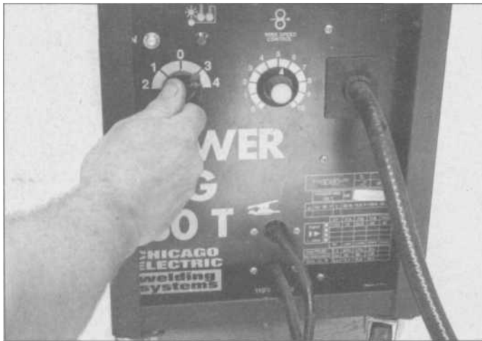
5.40 The basic MIG units have only a few power settings.
