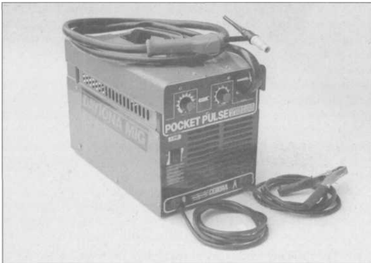
6.10 There are only a few small, more-portable TIG units, like this 100-amp "pulse-TIG" from Daytona MIG. It is a 220V, DC-only machine, but is said to be suitable for steel, stainless-steel and chrome-moly up to 3/16-inch thick.
