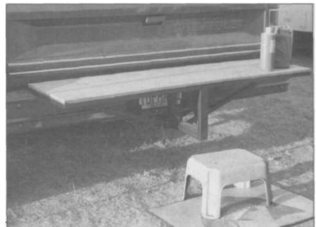
5.61 You'll find many uses for your welder once you get used to using it. This example of a typical home project is a plywood-covered rear bumper extension for a truck. It's used for carrying extra camping gear, and used as a tailgate for working or cooking when camping. Its also a wide step when stepping out of a camper shell on the truck.
