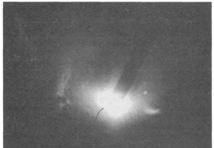
4.12 This is what you will see through your helmet and welding lens. The arc is intensely bright, but the lens cuts this down to just a bright glow around the arc itself, here you can just about see where the shielding gas cloud forms around the arc.
