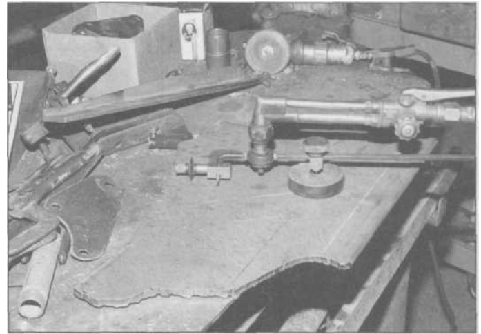
3.56 The same tool can be used, with different attachments, to cut a perfect circle of any size from a few inches to two feet in diameter. Removing as much of the human element of hand control makes for better parts that require less grinding to finish.
