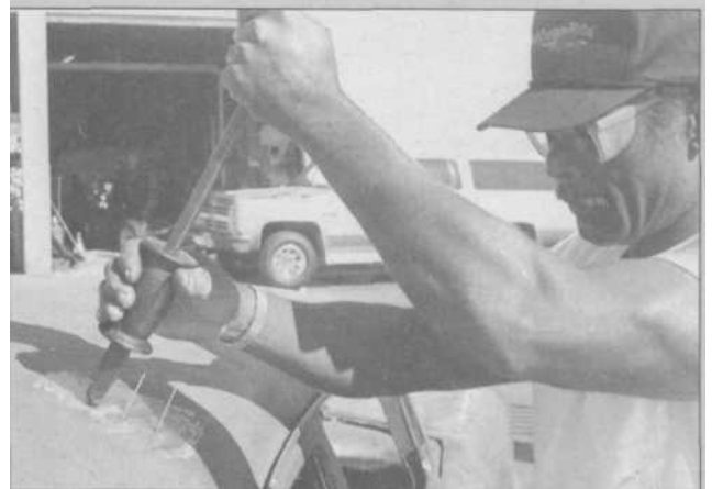
8.36 The studs are spot-welded in place, and a special slide hammer is used to pull out the dent or crease. Studs hold 500 pounds of pull.
