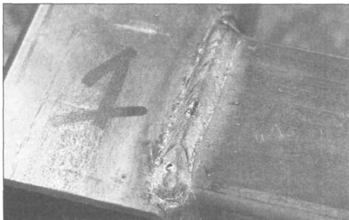
Small heat-affected zone on MIG weld
