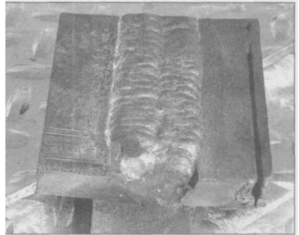
4.24 This sample weld shows how large plates are joined by multiple passes with large rods. Compare this front view (right) where the weld passes began, to the cutaway photo (left) which illustrates how integrated and free of contaminants even such a large weld can be.
