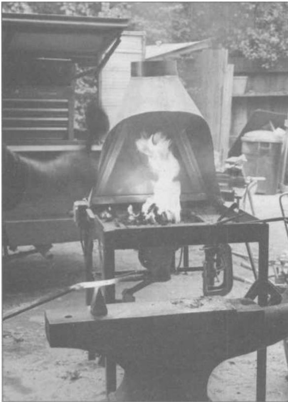
1.2 Metal cutting in the old days was no easier. A white-hot piece of metal was laid over a hardy (like a wedge or chisel point) in the big anvil, and struck hard with a hammer, chopping the softened piece off. Final shaping of most items was by hand with stones and files.
