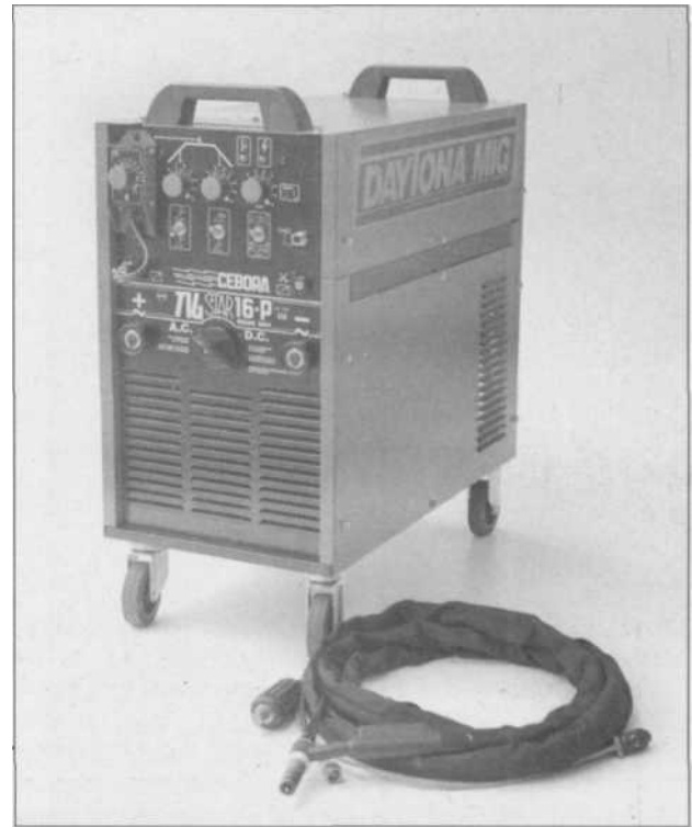
6.11 Mid-size TIG machines are in the 160-250 amp range, though this fairly-portable Daytona MIG unit is 130-amp, 220V. Mid-range machines offer options like slope control and post-flow. This one has square-wave technology, and AC/DC operation.
