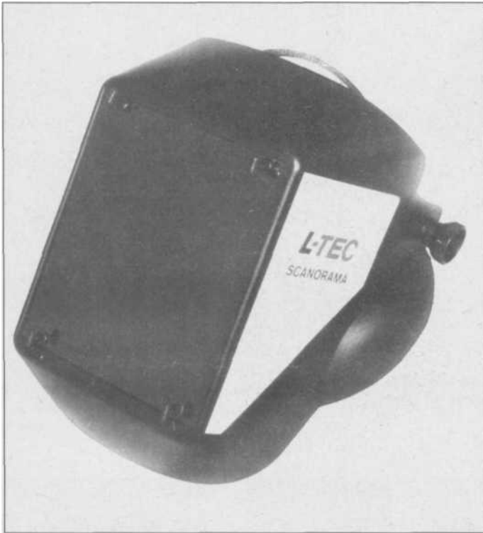
8.5 The Scanorama helmet was designed for MIG and TIG-welding applications, with a large shade 5 filter disc surrounding the welding lens. You can see most details through this area, but your skin is still protected from radiation. You look through the darker portion when welding.
