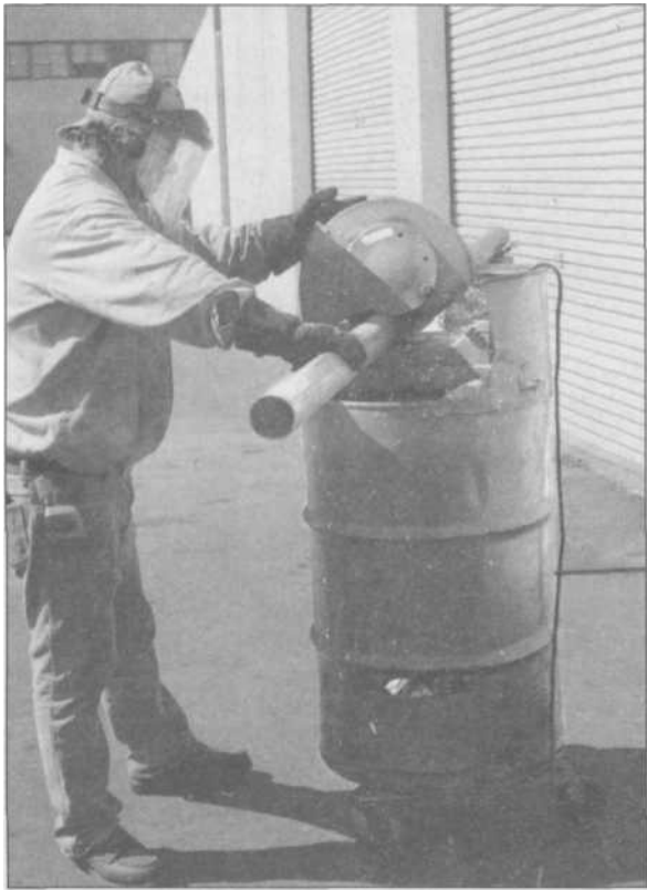
8.17 A "Radiac" or cutoff saw with an abrasive blade is very fast and secure when cutting large amounts of tubing. The work is held in a moveable vise so angle-cuts can be made. This one is cleverly mounted on a 55-gallon drum to capture all the sparks and debris.
