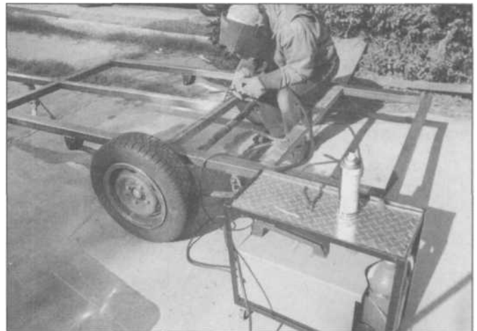
2.21 Typical home/shop projects such as a utility trailer, race-car trailer, metals rack, shop cart, engine stand, hoist and much more can be built at home with either MIG (shown) or an AC arc welder.
