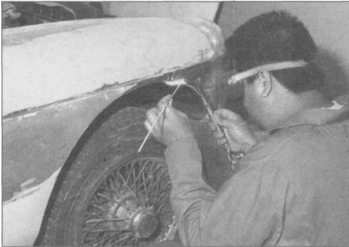
3.32 Brazing with a gas torch has many uses, such as repairing castings and antique-car sheet metal. Here a flux-coated rod is being used. Brazing is not a fusion process, so it is used where higher, melting-point heat might damage the work, or surrounding materials.
