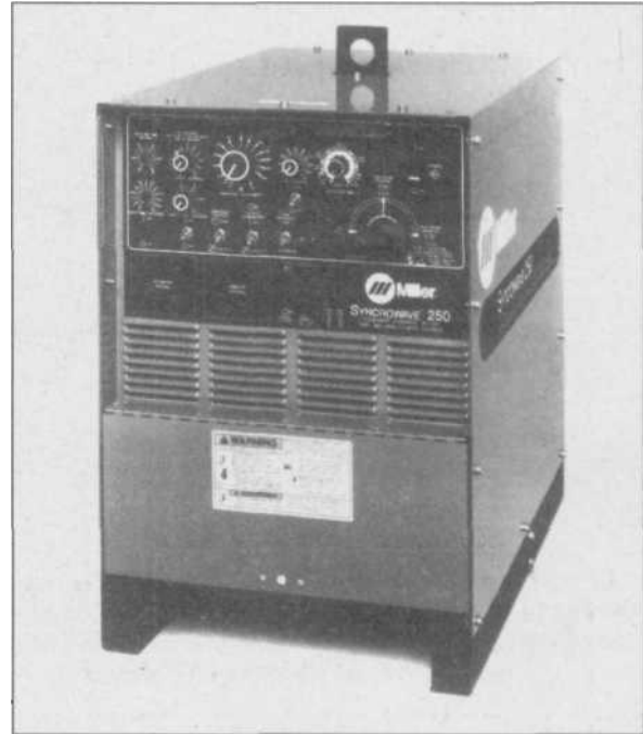
6.7 Most shop-type TIG welders are heavy, bulky power sources that require three-phase input power and water connections, making them less portable than other welding machines. This is a Miller Synchronwave 250, a popular unit in many fabrication and race-car shops.
