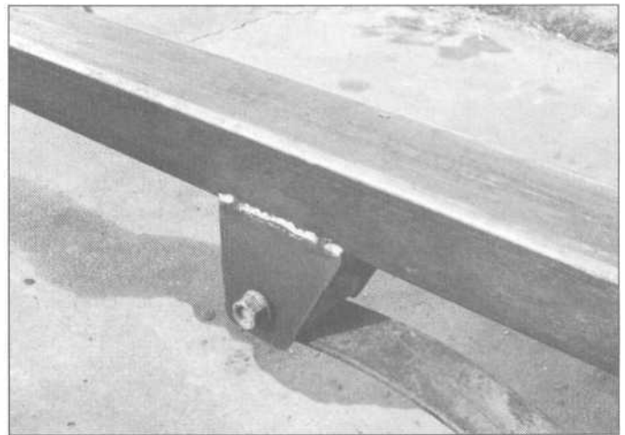
9.23 After some solid tack-welding, pull the springs out so the bushings don't melt, and fully-weld the four front spring mounts. Here the springs are bolted back in.
