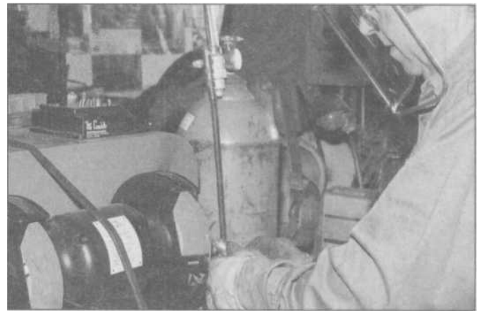
6.27 It's important to sharpen tungstens lengthwise on the tip, so as not to leave any radial grinding marks that could cause arc scatter. Grind points for steel like a pencil, like a crayon for welding aluminum.
