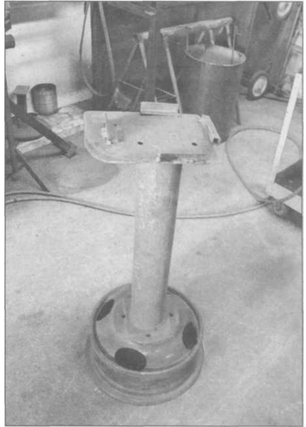
8.41 An old truck rim, a length of round pipe and a piece of scrap plate are combined with welding to make a perfect small welding table or mount for a grinder or sander.
