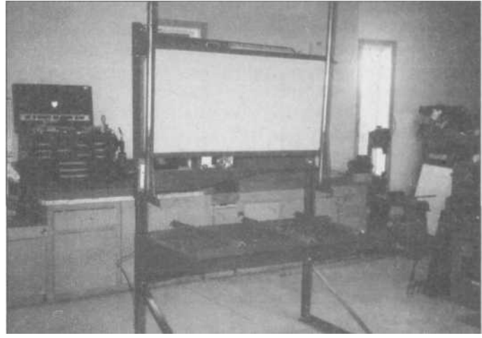
3.48 The complete Daytona MIG shape-cutting table is shown here with the erasable porcelain layout table folded up to take up less space when not being used. This table can be used with a gas torch or plasma cutter.
