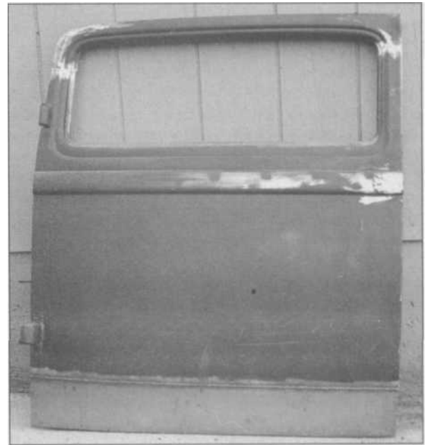
5.63 Street rod shops, customizers and restoration shops are using a MIG welder more and more, for its convenience and ability to handle delicate thin materials. This 1932 Ford door has had a new skin MIG-welded along the bottom where the original door was rotted away.
