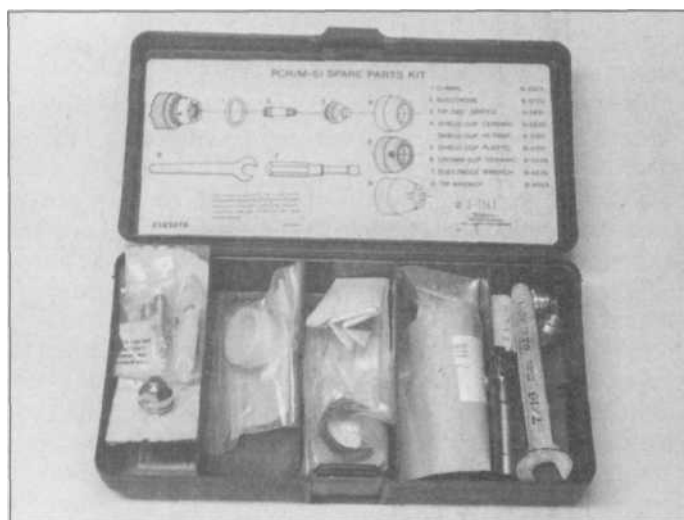
7.19 You'll need to keep on hand some spares of each of the torch components, including wrenches for changing the tip and the electrode.
