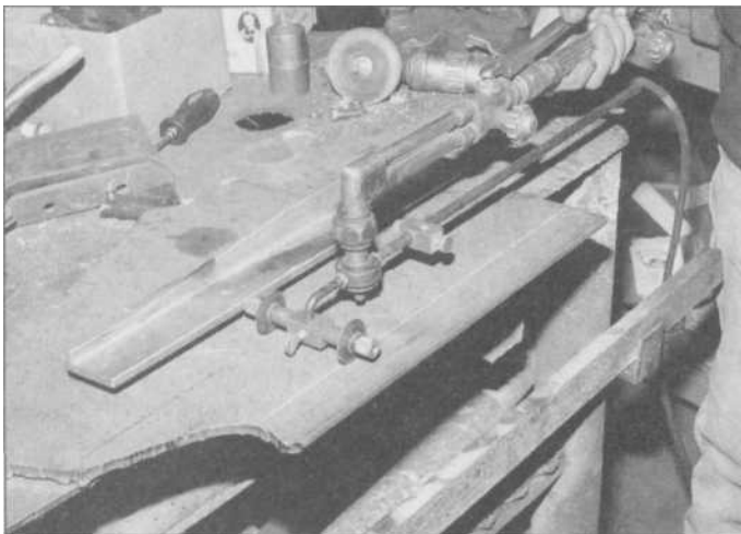
3.55 A great aid to cutting straight lines manually is this "compass" guide. It holds the torch tip firmly, but in a swivel arrangement that allows it to turn as you move along the line, and the torch stays the same distance from the work and much steadier. Here it is being demonstrated against another great tool, a magnetic steel guide that sticks strongly to the work and saves the hassles of setting up a bar or tube with some clamps.
