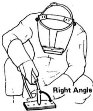
5.52 Instead of a straight butt-weld, panels of thin material are often joined with spot welds, in which the top panel is punched with small holes. You MIG-weld around the hole, joining the top panel to the bottom.
