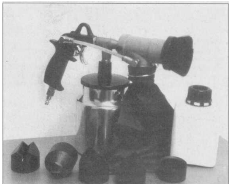
8.47 Daytona MIG sells this handy spot-sandblaster. It is useful for cleaning paint and rust away from a spot you have to weld, like a recess where a regular sander won't reach. Three-quarters of the blasting media is returned to the gun, so it won't make your shop a "sandpit."
