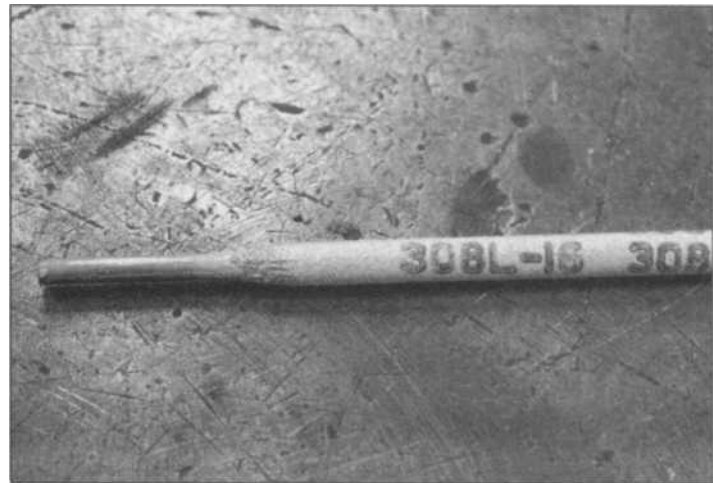
4.27 This is the bare end of the rod, where it fits into the electrode holder. You can judge the size of a rod from this bare end - don't measure the flux coating. Rods are marked as to their type and color-coded.
