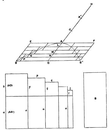
Then we can draw a cylinder or a frustum of a cylinder EBB'F passing through the circle or ellipse about BB' and having AD for its axis; also we can describe a cone or a segment of a cone through the circle or ellipse and having A for its vertex.
