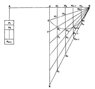
Suppose AO made equal to OQ, and conceive QOA as a lever placed horizontally and supported at O. Suppose the triangle EqQ suspended from OQ in the position drawn, and suppose that the trapezium  $EO_1$  in the position drawn is balanced by an area  $P_1$  suspended from A, the trapezium  $E_1O_2$ in the position drawn is balanced by the area  $P_2$  suspended from A, and so on, the triangle  $E_n O_n Q$  being in like manner balanced by  $P_{n+1}$ .
