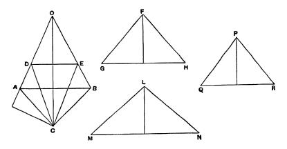
Take a cone FGH with base equal to the surface of the frustum DABE and height equal to the perpendicular (CK) from C on OA.
