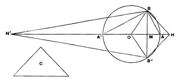
Let C be a cone whose base is equal to the surface of the segment BAB' of the sphere, i.e. to a circle with radius equal to AB [I. 42], and whose height is equal to OA.
