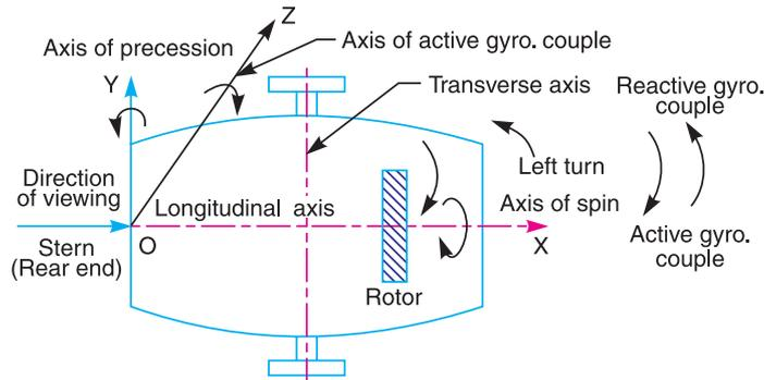
Fig. 14.8. Naval ship taking a left turn.
