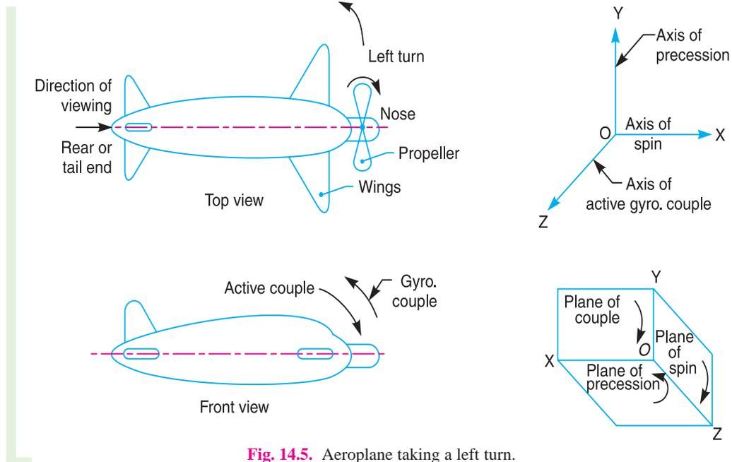
Fig. 14.5. Aeroplane taking a left turn.
