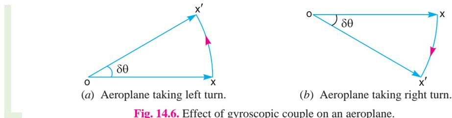
Fig. 14.6. Effect of gyroscopic couple on an aeroplane.
