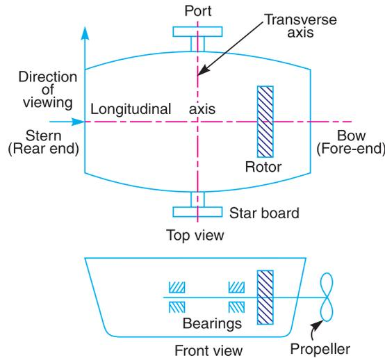
Fig. 14.7. Terms used in a naval ship.
