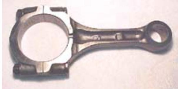
Connecting rod of a petrol engine.
