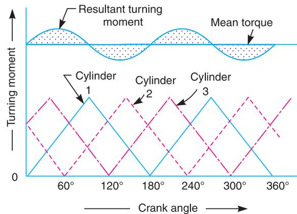
Fig. 16.3. Turning moment diagram for a multi-cylinder engine.
