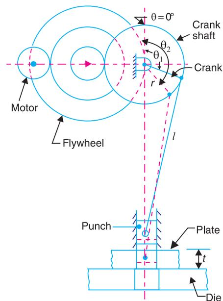
Fig. 16.22. Operation of flywheel in a punching press.
