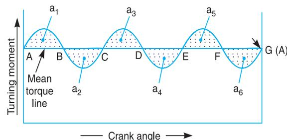
Fig. 16.4. Determination of maximum fluctuation of energy.
