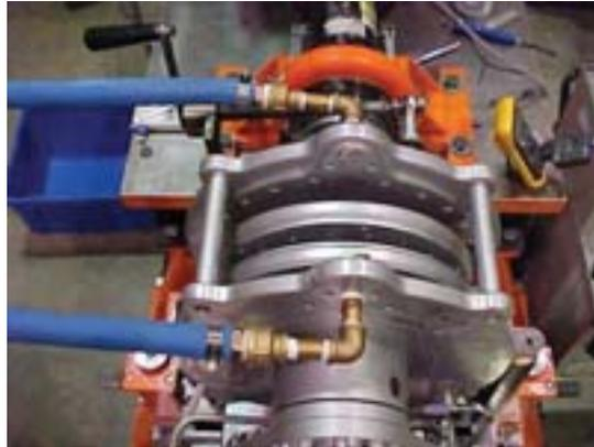
Dynamometers measure the power of the engines.
