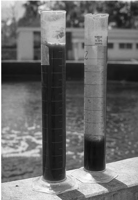
Figure 16.21 Sludge volume index testing for suspended-growth biomass.
