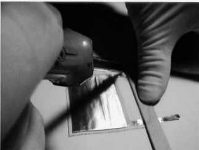
Sealing plastic with solder-iron
